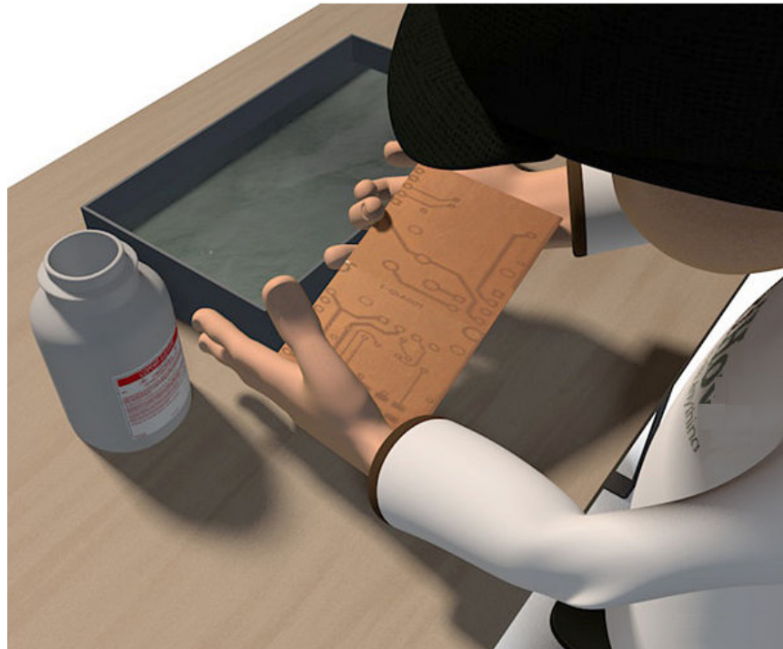
Figure 1-7: Preparing the acid etchant to submerge PCB
