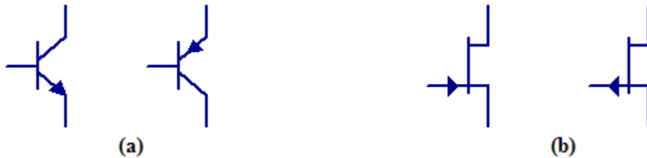
Figure 6-1: Transistor symbol; (a) Bipolar transistor symbols, NPN and PNP, (b) Field effect transistor symbols, N-channel and P-channel
