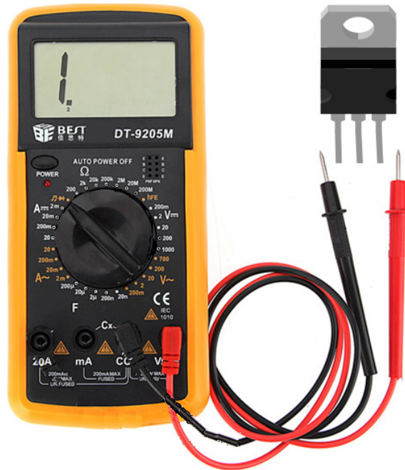
Figure 6-10: Testing MOSFET with digital multimeter set in diode check mode
