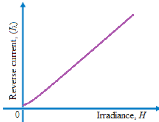
Figure 5-7: General graph of reverse current versus irradiance for a photodiode
