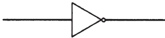
FIGURE 10.4 The symbol of an inverter – the simplest form of digital logic gate.
