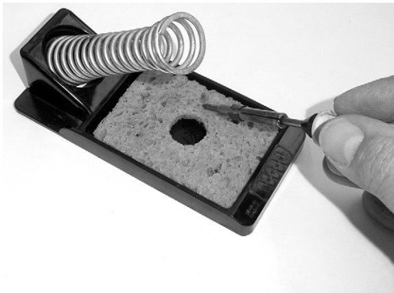
PHOTO 12.24 Cleaning a soldering iron bit tip using a wet sponge. Simply wipe the tip over the sponge surface.
