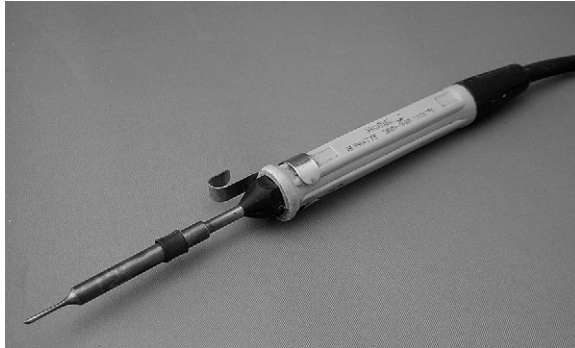
PHOTO 1.3 Low-wattage soldering iron intended for electronics.
