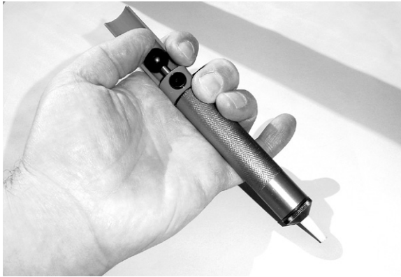
PHOTO 12.40 Priming the desolder pump by pressing down the charger.
