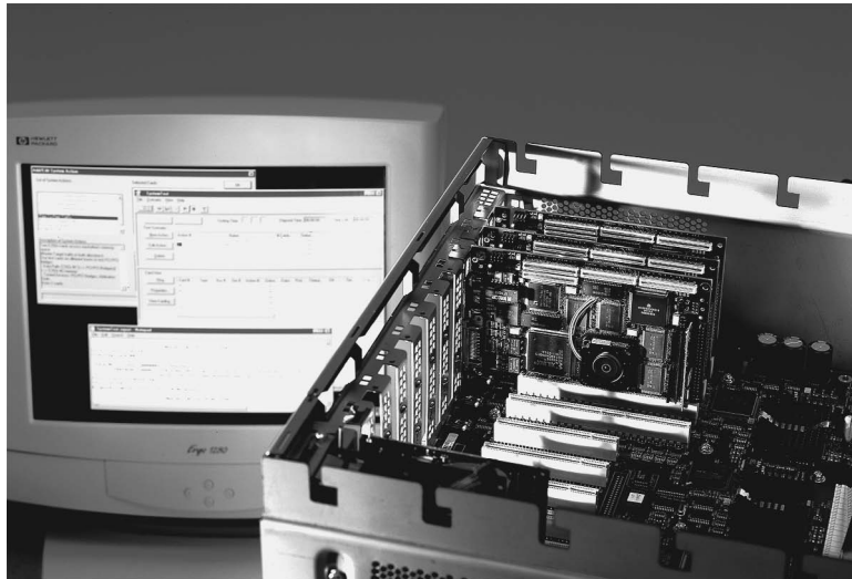
FIGURE 25.4.13 Protocol analyzers come in a number of physical configurations. Shown here are 3 Agilent Technologies E2920 PCI/PCI-X Exerciser and Analyzer cards plugged into a server undergoing production testing.
