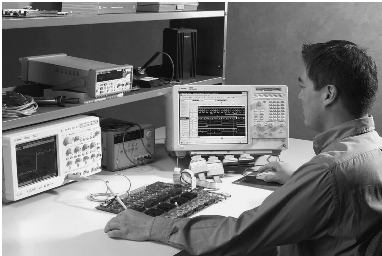
FIGURE 25.4.2 Logic analyzers are supplied as PC-hosted or benchtop versions. Shown here at right is the Agilent Technologies 1680 Benchtop Protocol Analyzer. Note the pods that connect to the device under test in the foreground.
