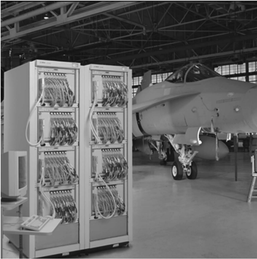
FIGURE 25.6.1 A typical modular instrument: VXI modules have been configured in this dual-rack structure, set on castors, to serve as a portable ground support test system for military avionics. (Photo courtesy of Agilent Technologies)
