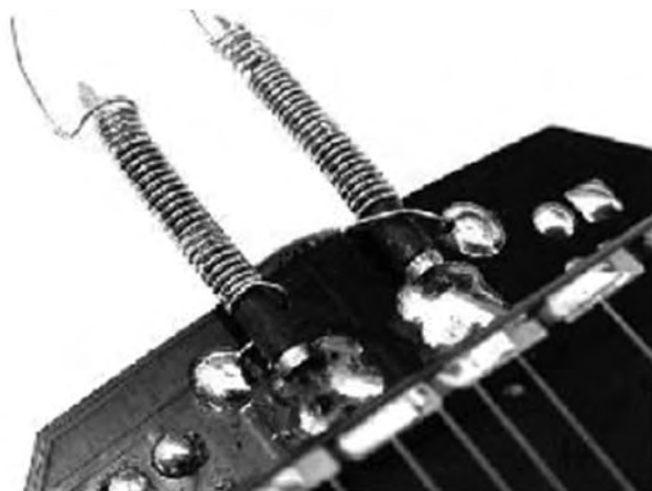
Finished sensor spring installation
