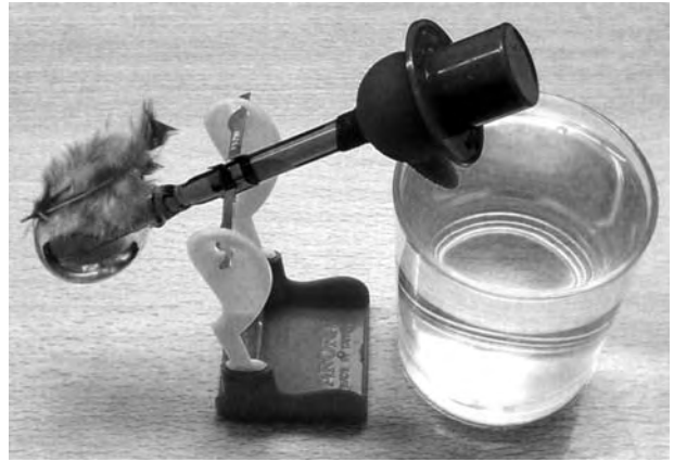
Figure 12-2 The Drinking Bird in action.
