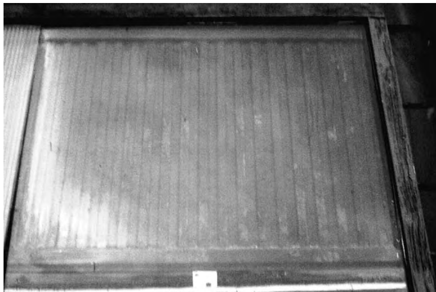
Figure 4-9 A recycled radiator collector.
