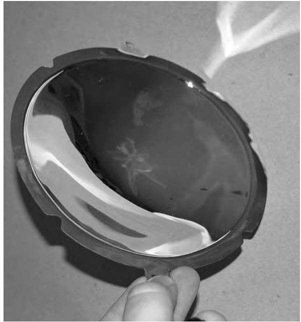
Figure 8-12a and b Parabolic mirrors take incoming parallel light (from the sun) and focus it to a point.
