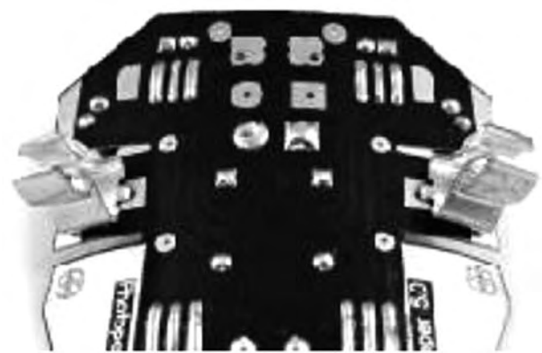
Figure 16-14 Both motor mounts ready. Image courtesy Solarbotics.
