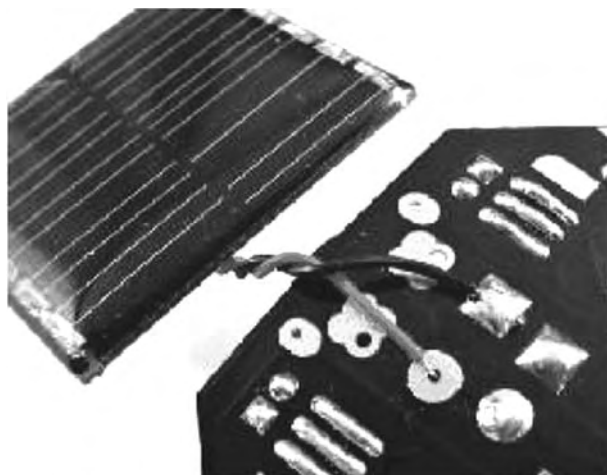
Solder the black wire to the Photopopper square pad, and the red wire to the Photopopper round pad
