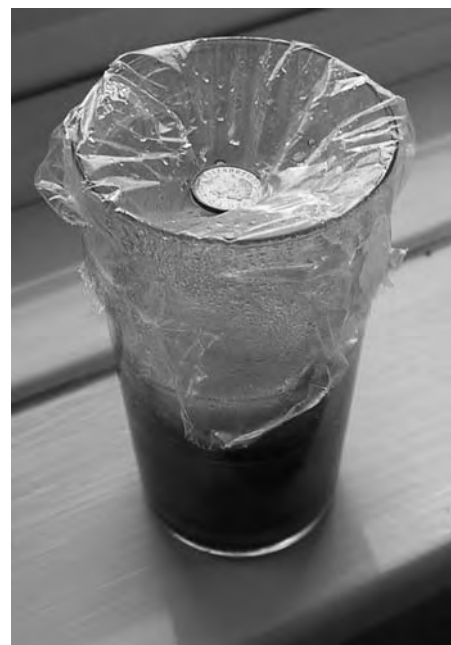
Figure 7-2 Demonstration solar still.
