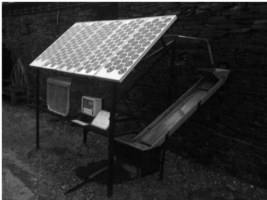
Figure 9-2 The solar pumping display at the Centre for Alternative Technology, U.K.
