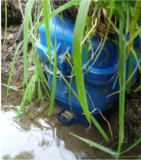
**Fig. 7.** The phosphate sensor *in-situ* during a trial at Broadmeadow Water, Co. Dublin, Ireland in September 2009. The sample inlet is visible below the water line.
