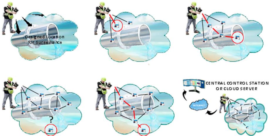
**Fig. 4.** Quick deployment of a wireless sensor network to collect data in provisional critical locations
