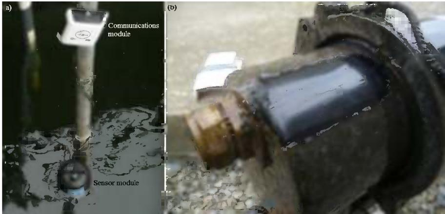
**Fig. 13.** (a) Second generation phosphate analyser *in-situ* at Osberstown Wastewater Treatment Plant, Co. Kildare, Ireland. (b) Biofouling on the analyser body after approx. 2 weeks immersion in wastewater.
