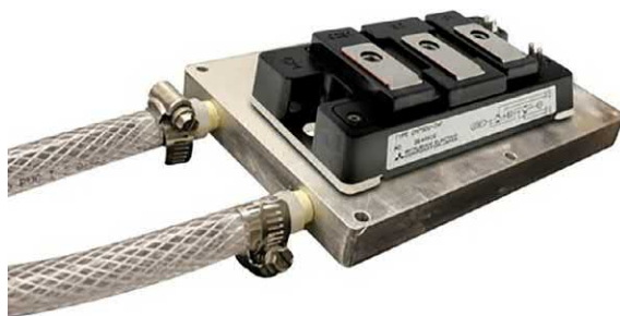
FIG. 8.112 When the amount of produced heat in the switch is considerable, water cooling is used.
