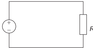
FIG. 8.6 The same resistor (as the one in Fig. 8.5) is connected to a DC source.
