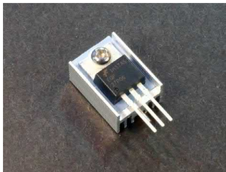
FIG. 8.116 A MOSFET switch with heatsink. The case of the device is often attached to the heat sink with a thermal compound to fill the small voids between the imperfect surfaces of the case and sink.
