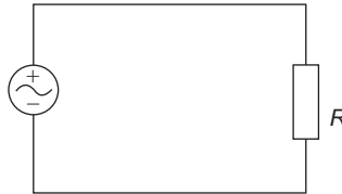
FIG. 8.5 A resistor is connected to a periodic voltage source.
