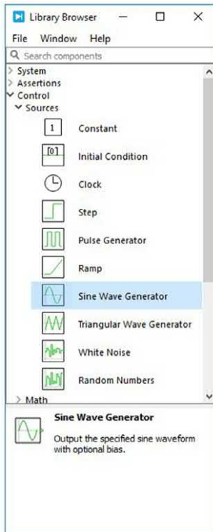
FIG. 3.250 Sine Wave Generator block.
