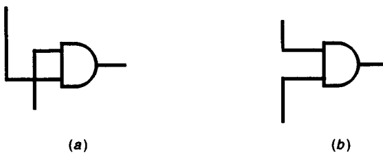
Fig. 2.4. Interchanging gate inputs.
