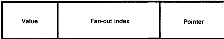
Fig. 6.10. Format of an 'event' in the event memory.
