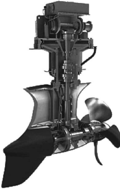
**FIGURE 7.8** Azipull propeller assembly details. (With permission from Rolls-Royce plc. © 2012, all rights reserved Rolls-Royce plc.)
