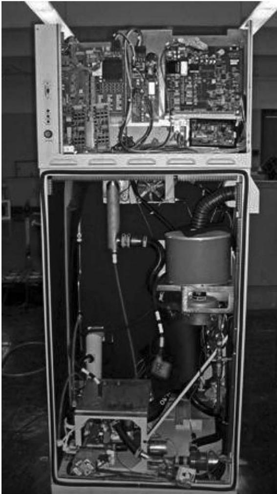
**FIGURE 10.2** A 5-kW fuel cell assembly with 60-Hz inverter at top. (From U.S. Merchant Marine Academy/Plug Power Corporation.)
