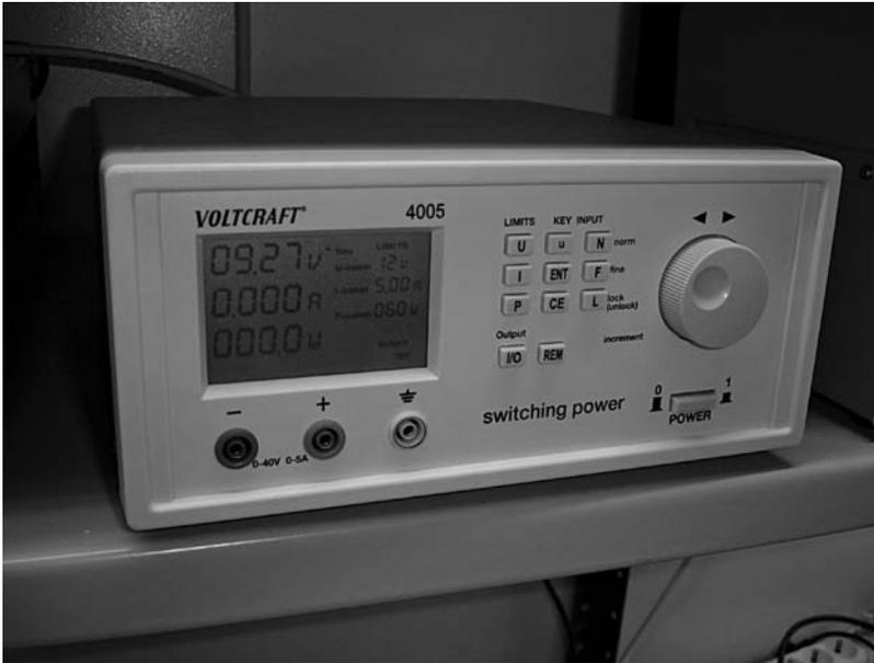
**FIGURE 2.14** Switch mode power supply exterior view (Voltcraft 4005).
