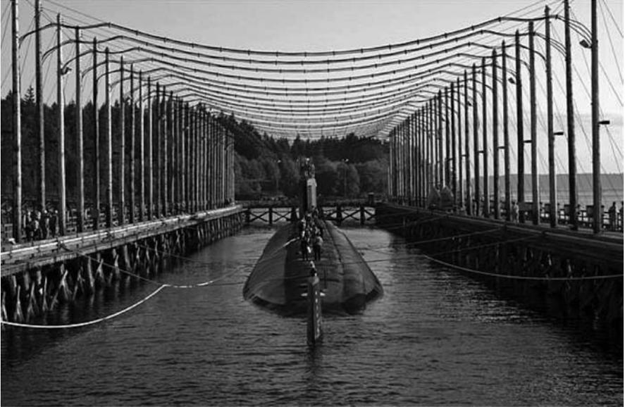
**FIGURE 9.3** *USS Jimmy Carter*, Seawolf-class attack submarine, undergoing deperming at Naval Base Kitsap Bangor.
