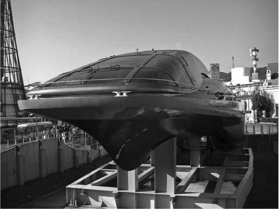
**FIGURE 11.7** Improved MHD-propelled demonstration boat Yamato-1 tested at Kobe, Japan.
