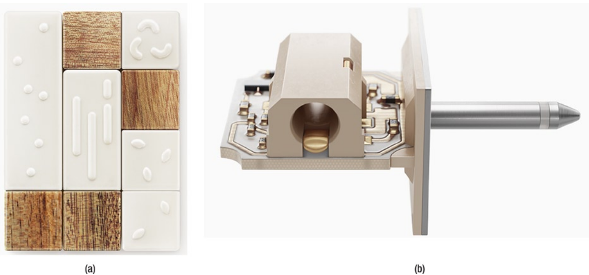
Figure 11-12. (a) Lapka's integrated sensors (b) The organic sensor module (images used with permission from Lapka)
