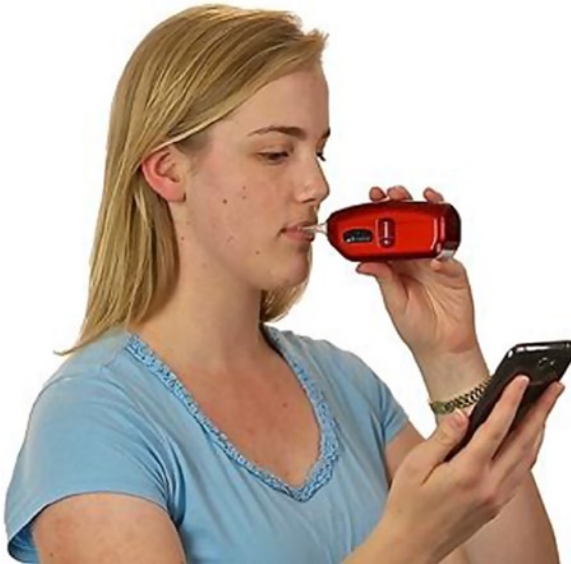
Figure 10-2. Breezing, a metabolism tracker device, is battery-operated and syncs with a smartphone. It includes an application used as user interface (image used with permission from Breezing Company)
