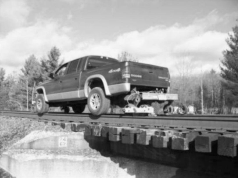
16.4 Photo of the EMAT-based Hy-rail system developed at Wavesinsolids (TISEC, 2011).
