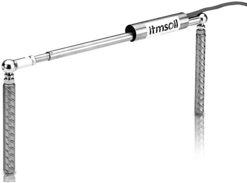
11.3 Crack gauge. (Source: Picture courtesy of itmsoil.)
