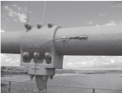
7.3 Fugro SMS sensors. (a) Cable tension; (b) wind speed and air temperature; (c) suspension cable temperature; (d) truss girder temperature.
