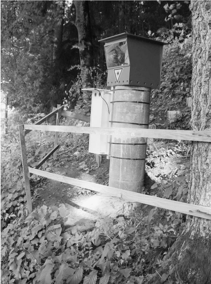
13.15 Robotic laser distance meter installed on a pillar. (Source: Picture courtesy SMARTEC SA and EPFL.)
