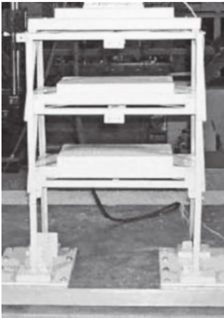
4.2 Three-story 1:10 scale building model.
