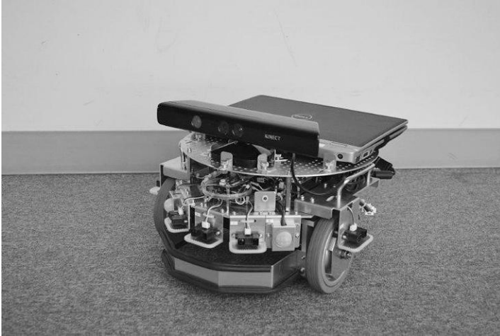
8.7 Sensor agent robot 'e-bio' with a notebook PC and a laser range finder.
