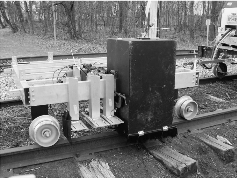
16.5 Early development of the UCSD laser/air-coupled system.
