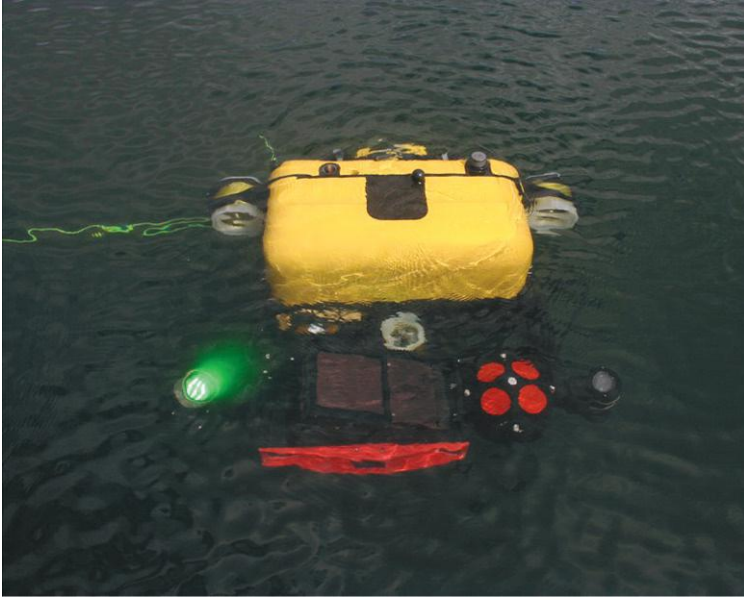
Plate XVI (Chapter 17) Photo of the MIT-Bluefin hovering autonomous underwater vehicle. (Source: Englot et al. , 2009.)
