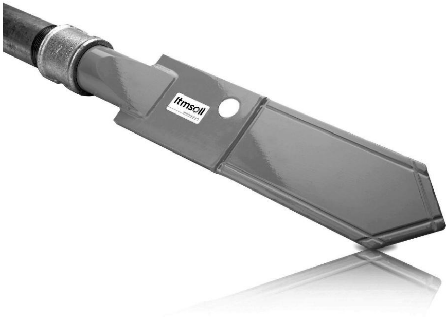
11.5 Spade pressure cell. (Source: Picture courtesy itmsoil.)
