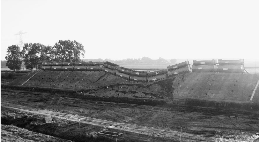
13.7 IJkdijk test levee after collapse. (Source: Image courtesy of Deltares.)
