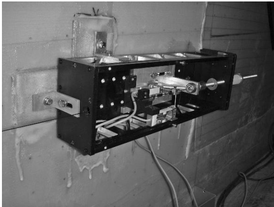
19.6 Active sensor unit of deflection sensor fixed to fiber patches inside a rotor blade (ISD).
