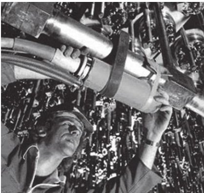
20.2 NDT techniques for NPP pipeline inspections: (a) Pipeline inspection using X-ray; and (b) P-scan inspection of a nuclear reactor.
