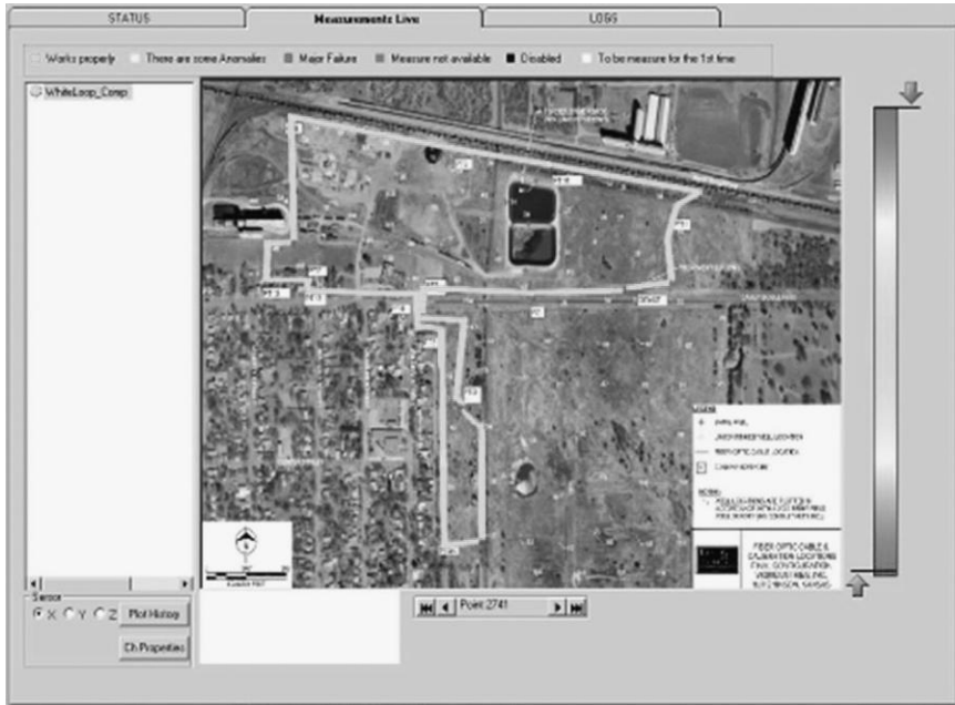
13.10 Cable layout and user interface for real-time display of movement locations. (Source: Photo courtesy of SMARTEC).
