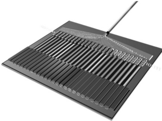
10.28 Schematic of a Si terabit transmitter with 25 single-wavelength hybrid Si lasers externally modulated at 40 Gb/s (Fang et al. , 2008).
