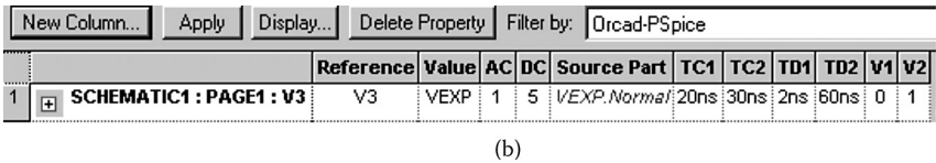
FIGURE 4.8 Exponential Source in PSpice schematic. (a) Symbol, (b) editing model parameters.
