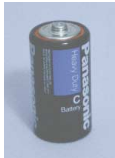
(b) C cell, commonly called a flashlight battery.
