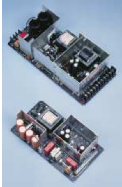
FIGURE 2–17 Fixed power supplies. (Courtesy of Condor DC Power Supplies Inc.)
