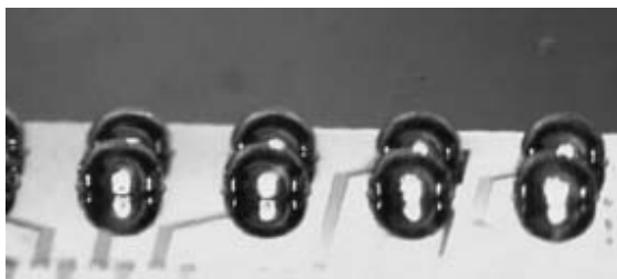
Figure 8.15 Spheres attached to distributed array utilizing laser attach method
