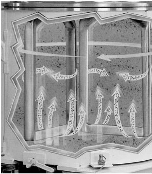
Figure 3.12 A Ross double planetary mixing equipment used for solder paste mixing
