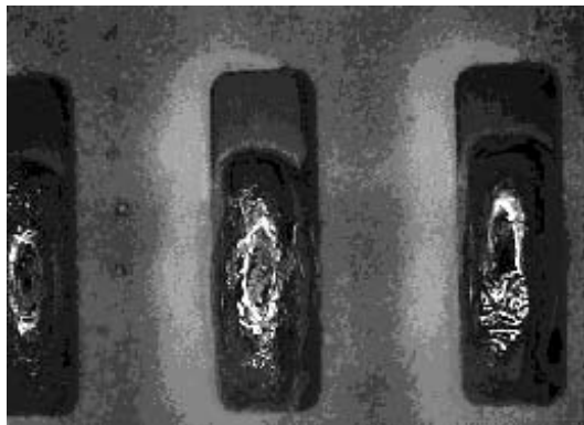
Figure 6.3 Example of nonwetting shown by the exposed copper pads
