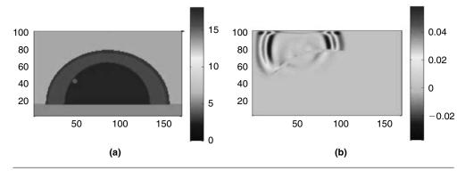
**FIGURE 32.5** Three-dimensional FDTD application of microwave breast cancer detection: (a) geometry map; (b) simulated model space.
