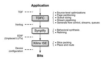
FIGURE 9.8 ■ TDF compilation flow targeting an FPGA.
