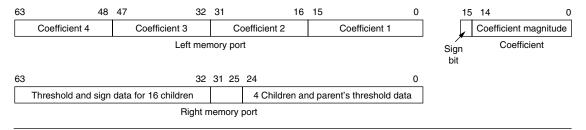
FIGURE 27.15 ■ Data passed to the SPIHT coder to calculate a single block.
