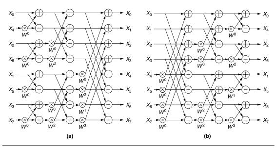
FIGURE 31.12 Variations of the 8-point, radix-2 FFTs with reordered inputs (a) and reordered outputs (b).
