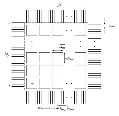
**FIGURE 36.3** ■ Wiring for instruction distribution.
