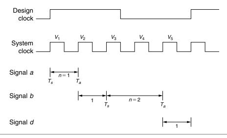
**FIGURE 30.12** The design clock cycle for the circuit mapping shown in Figure 30.8, including send times  $T_s$  and arrive times  $T_a$ .
