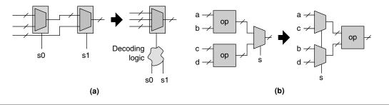
FIGURE 15.20 ■ Word-level optimizations performed by Ye et al. [23].
