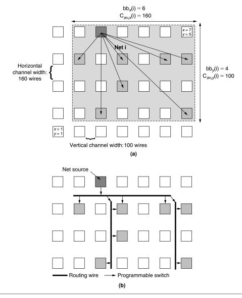
**FIGURE 14.5** An example wirelength cost computation: (a) net bounding box and average channel capacity; (b) best-case routing, with a wirelength of 11.
