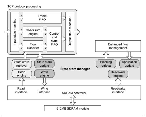
FIGURE 34.6 ■ A block diagram of the TCP processor.
