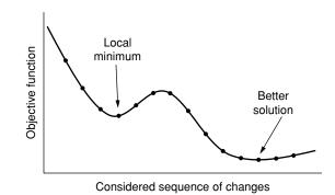
**FIGURE 26.9** Solution-worsening moves accepted by a nongreedy heuristic to escape local minima and find better solutions.
