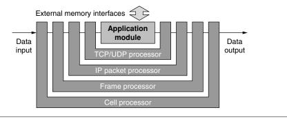
FIGURE 34.5 ■ Implementation of layered protocol wrappers on the FPX platform.
