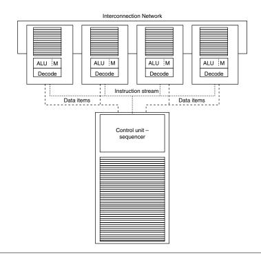
FIGURE 10.2 ■ An SIMD processing array.
