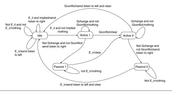
**FIGURE 29.5** The FSM associated with one variable.
