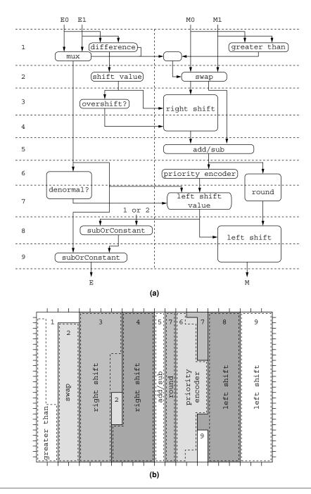
FIGURE 31.3 ■ Adder block (a) and adder layout (b) diagrams.
