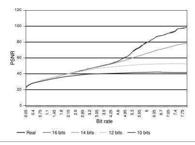
FIGURE 27.10 ■ PSNR versus bitrate for various coefficient sizes.
