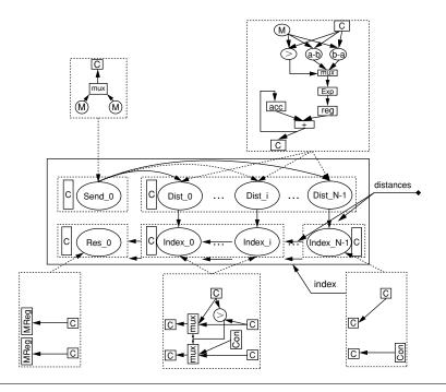
FIGURE 10.5 ■ An extended SIMD architecture.
