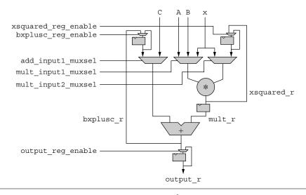
**FIGURE 6.4** • A time-shared datapath for computing  $Ax^2 + Bx + C$ .
