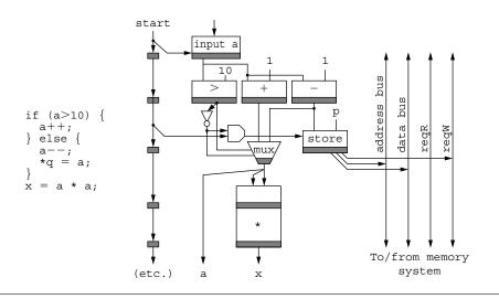
**FIGURE 7.3** If-conversion: Combining if-then-else using predicates and multiplexers.
