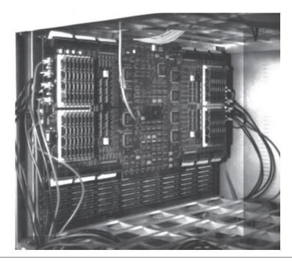
FIGURE 3.5 ■ A Hewlett-Packard Laboratories Teramac board.
