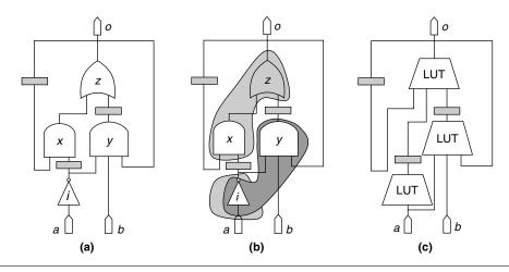
**FIGURE 13.1** Structural technology mapping: (a) original network, (b) covering, and (c) mapping solution.
