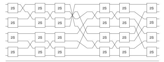
**FIGURE 16.16** Sorter recursion and layout for 8 inputs.
