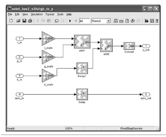
FIGURE 8.1 ■ An RGB-to-Y (intensity) Simulink diagram.
