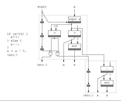
**FIGURE 7.5** ■ Optimizing the common path.
