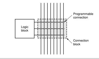
**FIGURE 1.6** Detail of a connection block.
