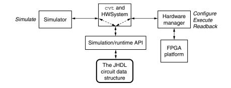
FIGURE 12.4 The JHDL unified simulation/hardware execution environment.
