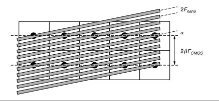
FIGURE 38.14 ■ Nanoscale and CMOS pitch matching via tilt.
