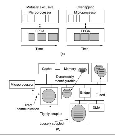
**FIGURE 26.8** Implementation models: (a) mutually exclusive and overlapping. (b) implementation model parameters.
