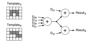
FIGURE 28.3 Common hardware shared between two templates.
