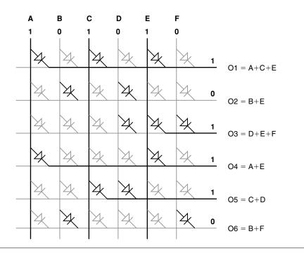
**FIGURE 38.5** The wired-OR plane operation.
