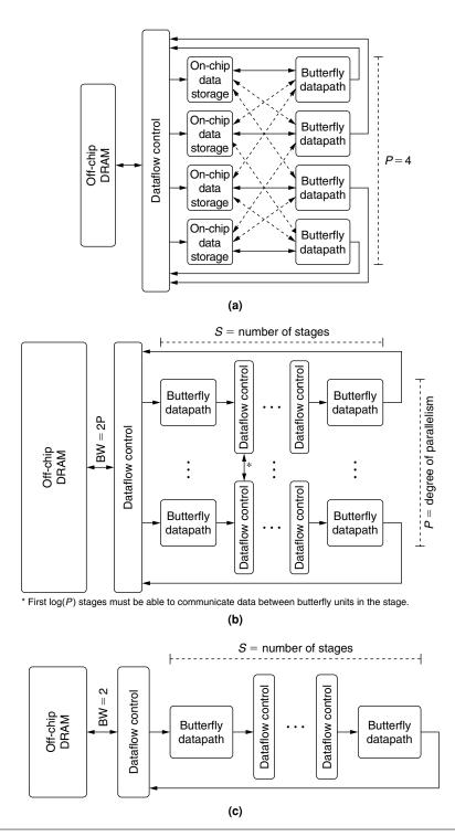
**FIGURE 31.13** Three architectures: (a) parallel, (b) parallel–pipelined, and (c) pipelined for exploiting parallelism in the FFT—from using all parallelism within a single stage to using all parallelism in the stages.
