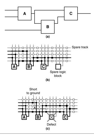
**FIGURE 37.1** Configuring computation to avoid defective elements in a reconfigurable array: (a) logical computation graph, (b) mapping to a defect-free array with spare, and (c) mapping to an array with defects.
