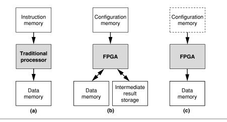
**FIGURE 28.12** • A comparison of a traditional computing model (a) with a dynamically reconfigurable model (b) and a statically reconfigurable custom model (c).
