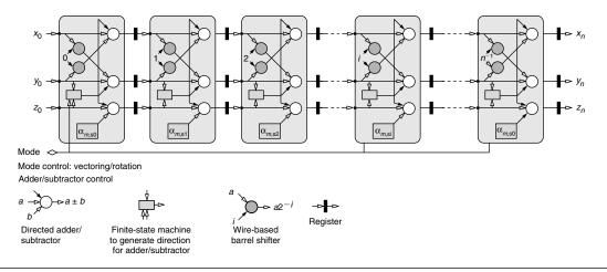
**FIGURE 25.10** A programmable parallel pipelined CORDIC array. In a completely unfolded implementation, the barrel shifters are realized as FPGA routing and so consume no resources other than interconnect.
