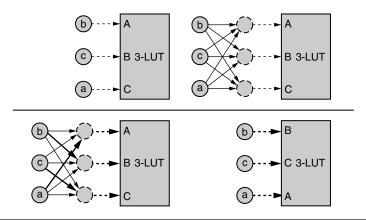
**FIGURE 17.5** Symmetric device inputs are handled by inserting pseudo-multiplexers.
