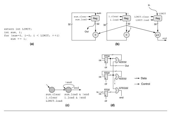
**FIGURE 15.1** From computation to realization.
