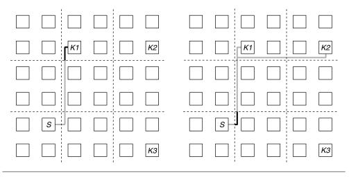
FIGURE 20.5 ■ Multi-terminal nets and region segmentation.
