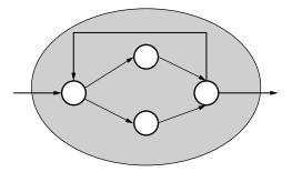
FIGURE 5.3 A single-rate static dataflow graph.
