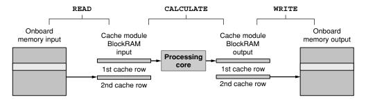
FIGURE 32.11 ■ A structural diagram of the simple 2-row cache module.
