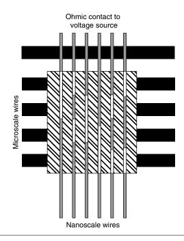
FIGURE 38.8 • A decoder for addressing individual nanowires assembled at nanoscale pitch.
