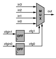
FIGURE 19.2 ■ A configurable 4-input multiplexer used in routing.
