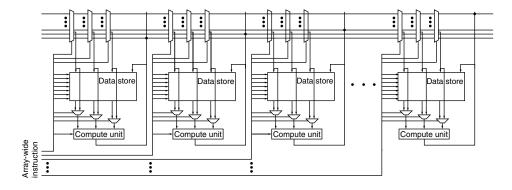
**FIGURE 36.1** ■ The general computational array model.
