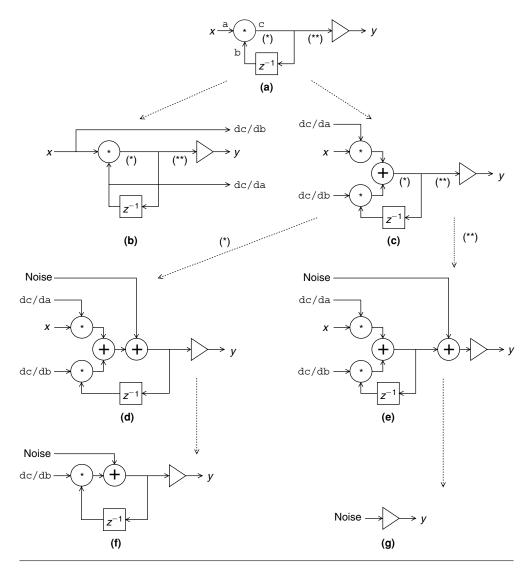
**FIGURE 23.7** An example of perturbation analysis: (a) original dataflow graph; (b) transformed dataflow graph; (c) linearized dataflow graph; (d) variant for (\*) signal; (e) variant for (\*\*) signal; (f) simplified graph for (\*) signal; (g) simplified graph for (\*\*) signal.
