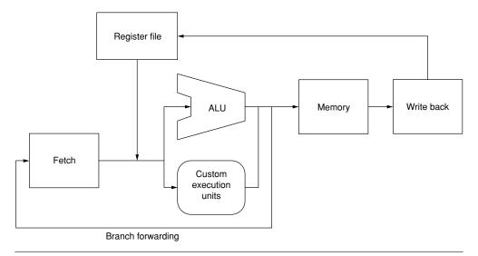
**FIGURE 22.4** A simplified architecture of a custom instruction processor. The standard arithmetic and logic operations are augmented by custom execution units that can accelerate particular applications.
