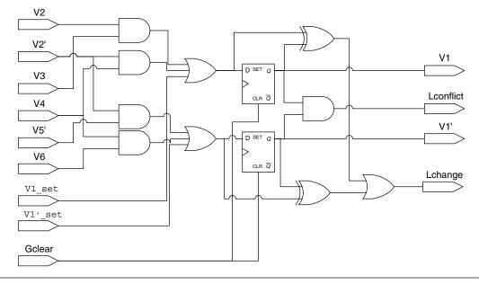
FIGURE 29.3 ■ The implication circuit for one variable, V1.
