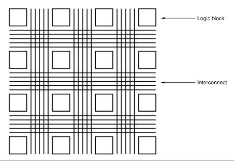
**FIGURE 1.3** The island-style FPGA architecture. The interconnect shown here is not representative of structures actually used.
