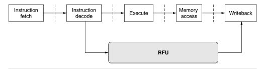
**FIGURE 2.13** An example of a pipeline of a processor with an RFU. (*Source:* Adapted from [16].)
