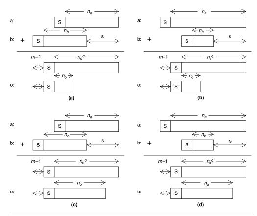
**FIGURE 23.8** Four multiple-wordlength adder formats arising in practice: (a) MSB of input b protruding beyond MSB of input a; (b) MSB of input a protruding beyond MSB of input b; (c) MSB of input b protruding beyond MSB of input a, with "free" output bits; (d) MSB input a protruding beyond MSB of input b, with "free" output bits. (s denotes the value of the BSHL generic; m denotes the value of the NULLMSBS generic.)
