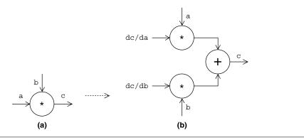
**FIGURE 23.5** ■ A local graph transformation to produce a small-signal model: (a) multiplier node; (b) first-order Taylor model.
