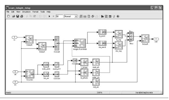
**FIGURE 8.10** A simple datapath with associated explicit control.
