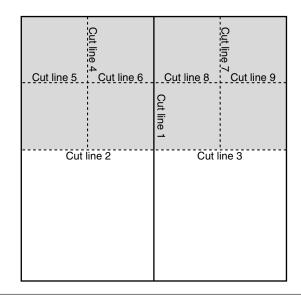
FIGURE 14.8 ■ The partitioning sequence for an island-style FPGA.
