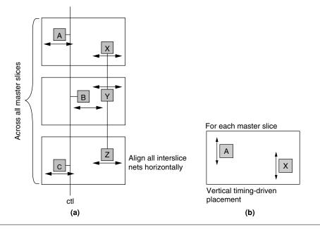
**FIGURE 15.22** Horizontal and vertical microplacement to restore regularity to compacted super-HWOP.
