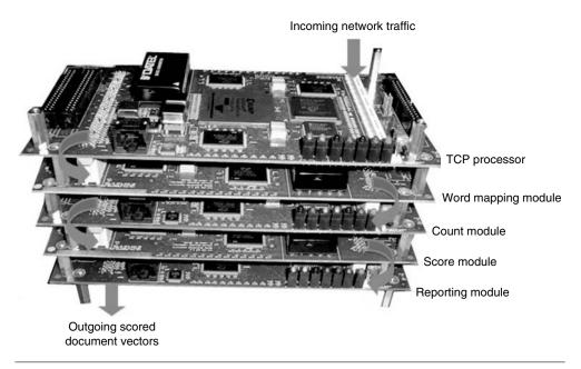
FIGURE 34.11 ■ A stack of the FPX modules implemented the semantic processing system.
