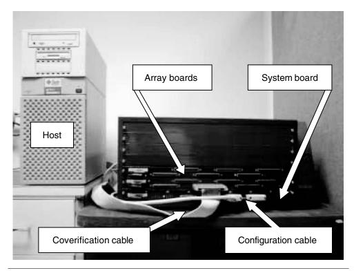
FIGURE 30.10 ■ A VirtuaLogic VLE-2M logic emulation system with two array boards.
