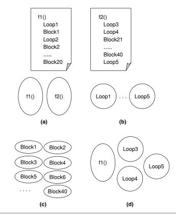
**FIGURE 26.6** The region granularities of an application (*top*): (a) functions; (b) loops; (c) blocks; (d) heterogeneous combination. Finer granularities may expose better solutions, at the expense of a more complex partitioning problem and more difficult estimation challenges.
