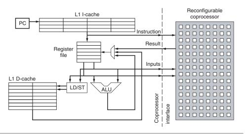
**FIGURE 5.12** A scalar processor with a reconfigurable coprocessor.
