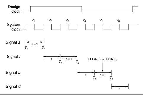
**FIGURE 30.19** The design clock cycle for the incremental mapping shown in Figure 30.18.
