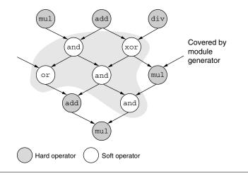
**FIGURE 15.13** Subgraph covering with flexible generator.
