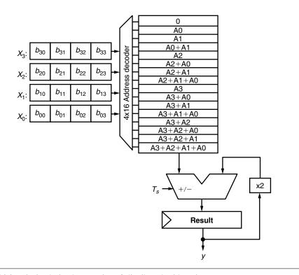
FIGURE 24.1 • A simple implementation of distributed arithmetic.
