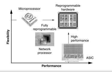
**FIGURE 34.2** Flexibility and performance trade-offs for networking systems that use microprocessors, network processors, ASICs, and reprogrammable hardware.
