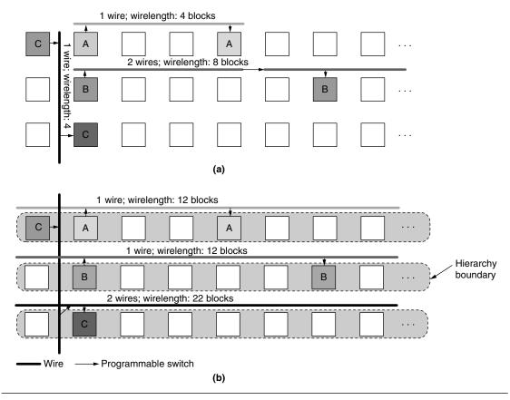
**FIGURE 14.2** ■ Influence of the routing architecture on wirelength for a given placement: (a) sample routings on a Stratix-II FPGA (island style), and (b) sample routings on an APEX FPGA (hierarchical).
