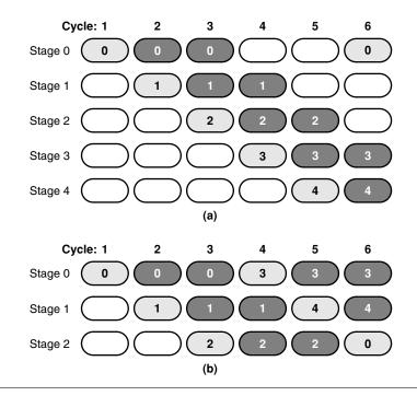
**FIGURE 2.3** The virtual pipeline stages of an application (a). The light gray blocks represent the configuration of a pipeline stage; the dark gray blocks represent its execution. The mapping of virtual pipeline stages to three physical pipeline stages (b). The physical pipeline stages are labeled each cycle with the virtual pipeline stage being executed. (*Source:* Adapted from [6].)
