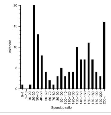
**FIGURE 29.6** A performance comparision of the FPGA SAT accelerator and the software version implementing the same algorithm as hardware.
