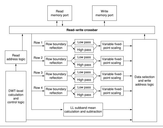
FIGURE 27.9 A discrete wavelet transform architecture.
