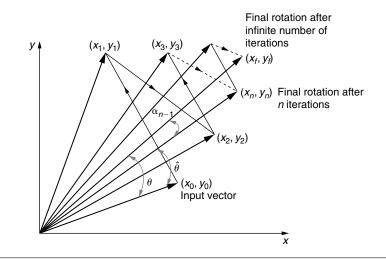
**FIGURE 25.3** Each iteration of a CORDIC rotation introduces vector growth by a factor of  $\frac{1}{\cos \alpha_i} = (1 + \sigma_i^2 2^{-2i})^{1/2}.$
