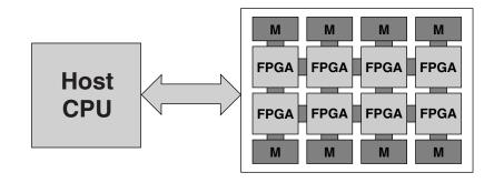
**FIGURE 3.1** ■ The traditional processor/coprocessor arrangement for reconfigurable computing hardware.
