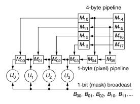
FIGURE 28.8 A systolic image array pipeline.
