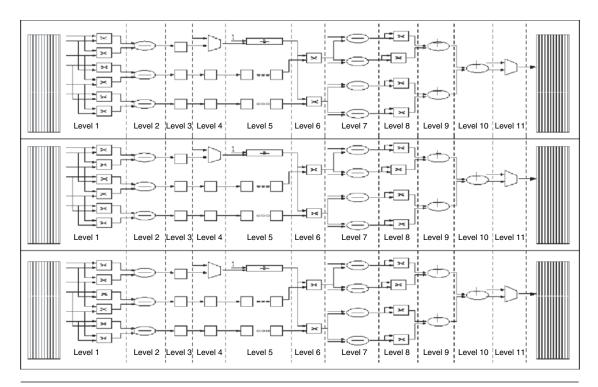
FIGURE 10.6 SIMD with pipelined vector units.
