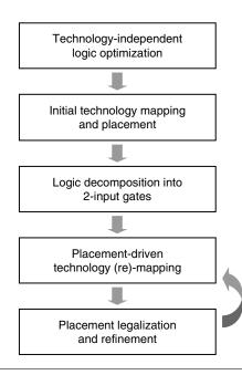
FIGURE 13.6 ■ Iterative mapping, placement.
