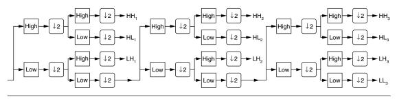
FIGURE 27.8 A generic 2D biorthogonal DWT.
