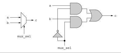
FIGURE 6.1 A structural 2-input multiplexer.
