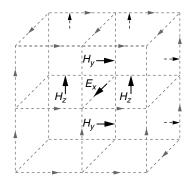
FIGURE 32.2 ■ Example of electric and magnetic components on a 4-cell grid.
