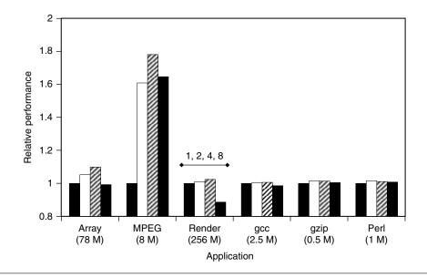
FIGURE 35.16 ■ Performance versus processor width.
