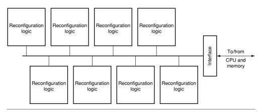
**FIGURE 4.6** ■ In a block reconfigurable device, configurations can be relocated to any of the interconnected and equivalent blocks of reconfigurable logic.
