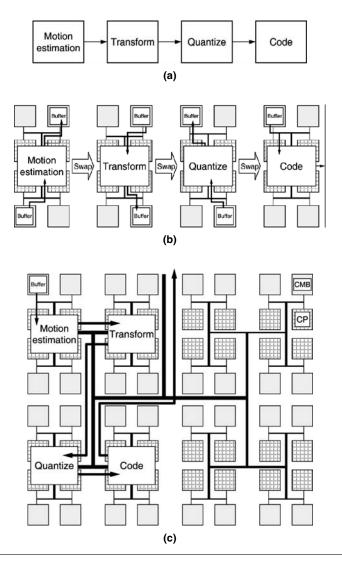
**FIGURE 9.1** Score application and sequential versus fully spatial execution: (a) a video compression task, (b) a capacity-limited sequential implementation, and (c) a fully spatial implementation on SCORE hardware.
