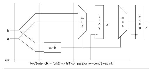
FIGURE 16.12 ■ Two-sorter layout and behavior specification.
