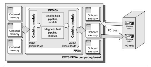
FIGURE 32.10 A structural diagram of the memory interface.
