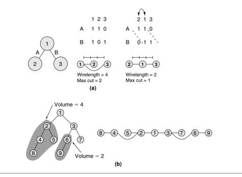
FIGURE 15.16 ■ Postmapping linear placement.
