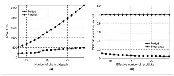
**FIGURE 25.11** ■ (a) Comparison of the FPGA resource requirements for folded and linear array CORDIC architectures—circular coordinates. (b) Throughput in rotations/vectoring operations per second for the two architectures. A normalized clock rate of 1 is assumed.
