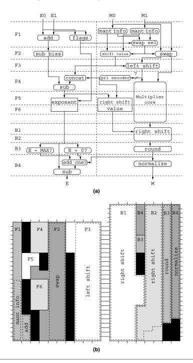
FIGURE 31.4 ■ Multiplier block (a) and multiplier layout (b) diagrams.
