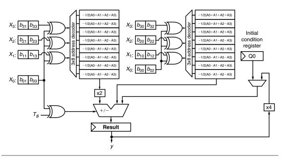
**FIGURE 24.4** Two-bit-at-a-time reduced memory DA implementation.
