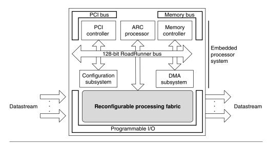
**FIGURE 2.11** Chameleon's RCP architecture. (*Source:* Adapted from a figure obtained off of Chameleon System's home page, which is no longer available.)
