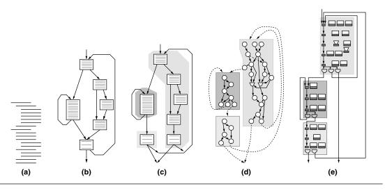
**FIGURE 7.6** Overall compiler flow: (a) original C source code, (b) CFG basic blocks, (c) clustering of basic blocks into hyperblocks, (d) construction of the DFG, and (e) circuit generation from the DFG.
