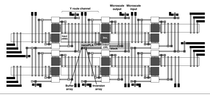
**FIGURE 38.13** In nanoPLA block tiling with edge I/O to lithographic scale.
