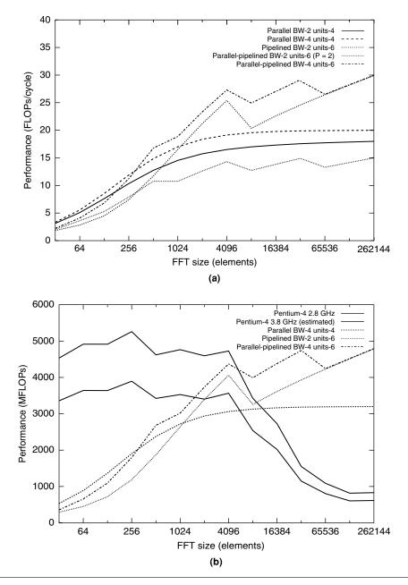
**FIGURE 31.14** ■ A comparison of performance for different FFT architectures in FLOPs per cycle (a) and a comparison of FFT implementation on FPGAs and CPUs (b).
