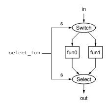
FIGURE 5.6 Data-driven function selection in the dataflow model.
