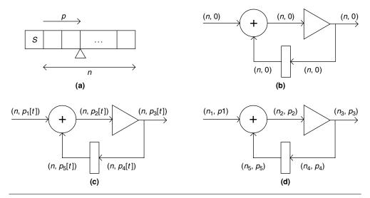
**FIGURE 23.1** ■ The multiple-wordlength paradigm: (a) signal parameters ("s" indicates a sign bit); (b) fixed point; (c) floating point; (d) multiple wordlength. The triangle represents a constant coefficient multiplication, or "gain"; the rectangle represents a register, or unit sample delay.
