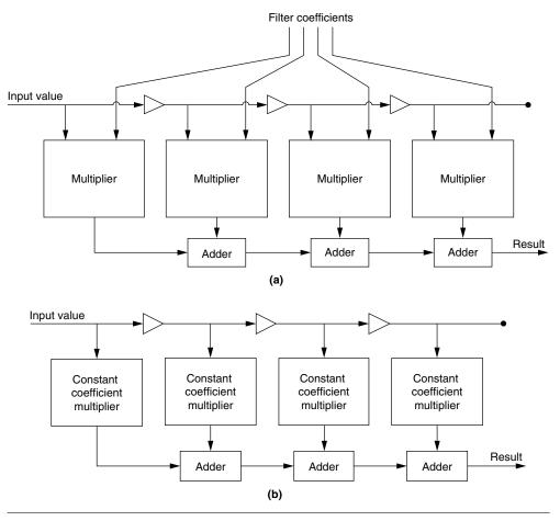
**FIGURE 22.2** FIR filters utilizing (a) general multipliers with variable filter coefficients and (b) instance-specific multipliers specialized to filter coefficients.
