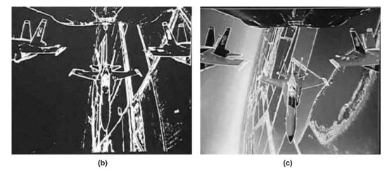
**FIGURE 8.15** (a) The Sobel edge detection filter running on the BEE2, showing the BEE2 console and video output on two LCD displays, with (b, c) two examples of edge detection results based on interactive user configuration from the console.
