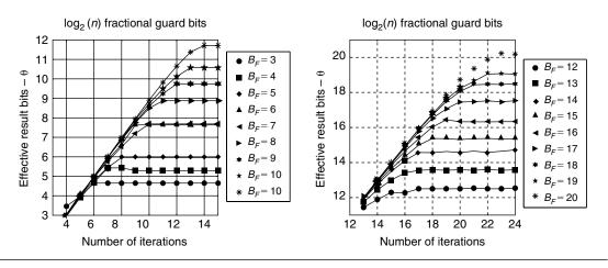
**FIGURE 25.6** The efficitive number of result bites for a CORDIC vector processor (circular coordinates). The number of fractional guard bites is  $G_F = \lceil log_2(n) \rceil$ .
