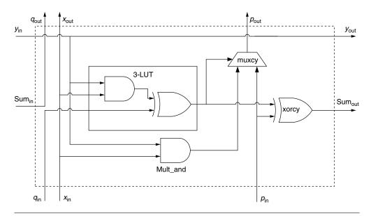
FIGURE 22.8 ■ This cell design can be replicated in a grid arrangement to create a multiplier.
