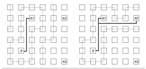
FIGURE 20.4 ■ PathFinder exploration and multi-terminal nets.
