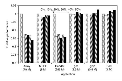
FIGURE 35.17 ■ Performance versus random processor defects.
