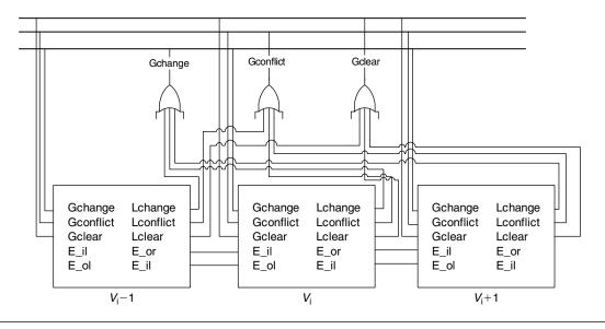
FIGURE 29.4 ■ The global topology for a basic SAT solver circuit.
