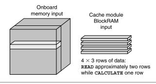
**FIGURE 32.14** A structural diagram of the  $4 \times 3$  row caching module.
