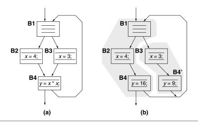
**FIGURE 7.9** The commonly taken path in the loop is B1-B2-B4 (a). Hyperblock formation (b)—tail duplication occurs with basic block B4. This enables constant propagation and then constant folding for the expressions x\*x, although this is actually done after conversion to the DFG.
