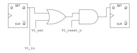
FIGURE 29.9 ■ One stage of the pipelined bus.
