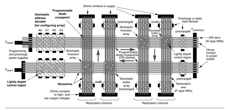
**FIGURE 38.10** ■ A simple nanoPLA block.
