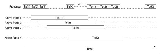
FIGURE 35.7 ■ An array-insert operation demonstrating processor and Active Page computations.
