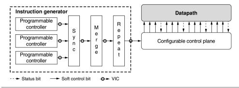
FIGURE 2.9 ■ RaPiD's instruction generator. (Source: Adapted from [5].)
