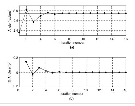
**FIGURE 25.4** Convergence of CORDIC vectoring. The top plot (a) shows the true angle of the input vector  $\arg(x_s + jy_s)$  (solid line) overlaid with  $\arg(x_i + jy_i)$ , i = 1, ..., 16. The bottom plot (b) is the percentage angle error as a function of the iteration number.
