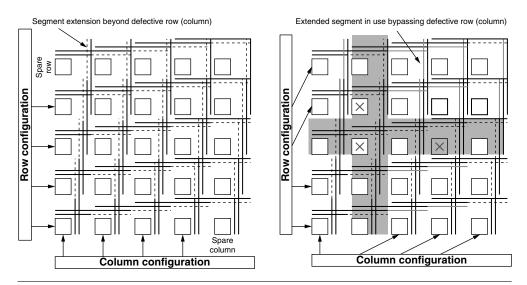
FIGURE 37.3 Arrays designed to support row and column sparing.
