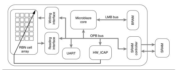
**FIGURE 33.8** The setup of a complete and centralized self-reconfigurable evolvable platform.
