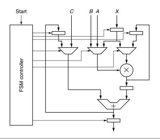
**FIGURE 5.9** FSMD for a single multiply and add datapath for quadratic equation evaluation.
