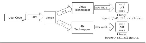
FIGURE 12.2 ■ The relationship of user code, Logic class methods, and Techmapper objects.
