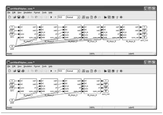
**FIGURE 8.13** Two versions of the model schematic for the  $biplex\_core$  library component, with the size of the FFT set to 6 (2<sup>6</sup>) and 4 (2<sup>4</sup>). The schematic changes dynamically as the parameter is adjusted.
