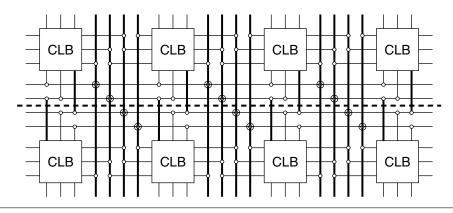
**FIGURE 11.5** A generic FPGA architecture may have resources (*bold lines*) that cross the boundary (*dashed line*) between two hardware tasks.
