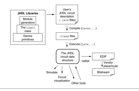
FIGURE 12.1 ■ An overview of the design process and the JHDL system.
