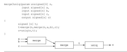
**FIGURE 9.5** ■ The TDF compositional operator.
