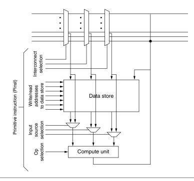
FIGURE 36.2 ■ Primitive instruction (pinst) for programmable bitops.
