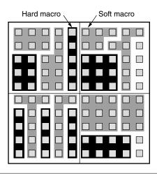
FIGURE 15.17 ■ Bin-based two-dimensional HWOP floorplanning.
