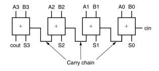
FIGURE 1.10 ■ A simple 4-bit full adder.
