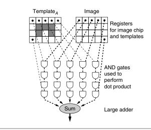
FIGURE 28.4 ■ The ASIC version of the equivalent function.
