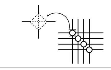
FIGURE 1.7 ■ An example of a common switch block architecture.
