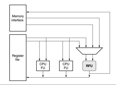
FIGURE 2.12 ■ The datapath of the processor + RFU architecture.
