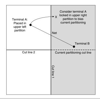
FIGURE 14.9 An example of terminal propagation.
