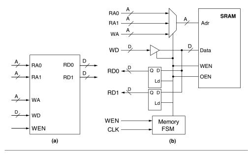
**FIGURE 30.13** A mapping of a multiported design memory to a single-ported emulator memory: (a) parallel-accessed multiport memory; (b) sequentially accessed single-port multiplexed memory. *Source:* Adapted from Agarwal [1].
