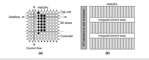
FIGURE 15.4 Common datapath layouts: (a) classical linear and (b) multistripe.
