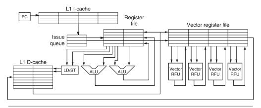
**FIGURE 5.14** A super-scalar processor with vector functional units.
