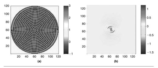
**FIGURE 32.6**  $\blacksquare$  (a) The floorplan of the spiral antenna model; (b) an FDTD-simulated two-dimensional space.
