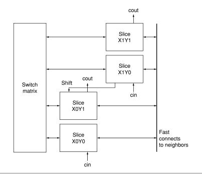
**FIGURE 1.16** ■ Xilinx Virtex-II Pro configurable CLB. (*Source:* Adapted from [8], Figure 32, p. 35.)
