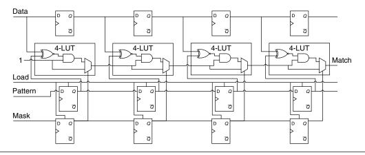
**FIGURE 22.11** • A general bit-level pattern matcher, shown for 4-bit patterns. The pattern matcher circuit is controlled by a pattern and a mask, which can be loaded by asserting the load signal. If the mask bit is set for a particular position, the matcher will attempt to detect a match between the pattern bit and the data bit.
