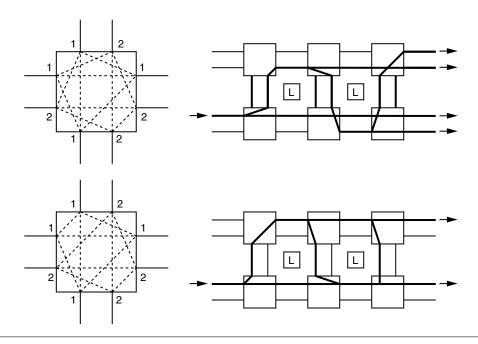
FIGURE 20.7 Switch box style and routability.
