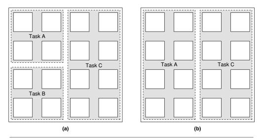
**FIGURE 11.2** Flexible binding allows tasks to use a different number of resources based on hardware capacity and resource availability. In this example, Task A can either occupy less area at the expense of performance (a), or achieve a higher data rate at the expense of area (b).
