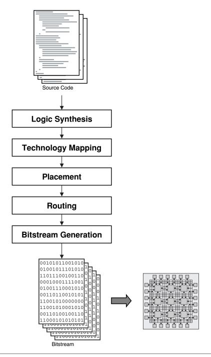
**FIGURE I.2** ■ A typical FPGA mapping flow.
