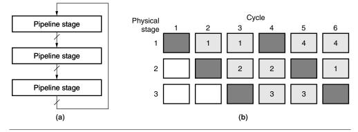
**FIGURE 4.5** • A pipeline reconfigurable architecture with three physical stages (a). A 3-stage physical pipeline implementing a 4-stage virtual pipeline (b). Numbers within physical pipeline stages indicate the implemented virtual pipeline stage. Shaded stages are reconfiguring for the given cycle.
