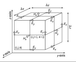
**FIGURE 32.1** ■ The geometrical representation of the three-dimensional Yee cell.
