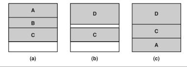
**FIGURE 4.4** ■ Three configurations have been programmed on the hardware (a). In (b), A and B have been removed, and D has been relocated/configured to an available area, causing fragmentation. Defragmentation relocates configuration C to make room for configuration A when it is again needed, this time to a new location in the array (c).
