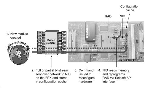
**FIGURE 34.13** Remote reconfiguration of the FPX platform.
