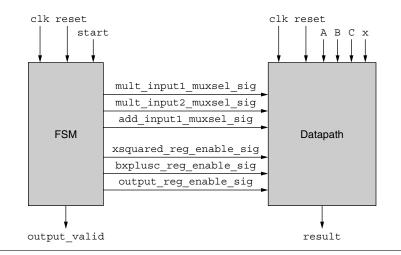
**FIGURE 6.3** • A structural representation of the FSM datapath design.
