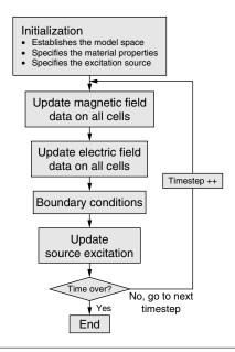
FIGURE 32.3 ■ The flow diagram of the FDTD algorithm.
