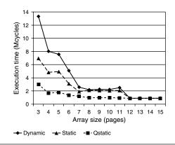
**FIGURE 9.10** JPEG decoder scaling: Total execution time is compared among fully dynamic, fully static, and quasi-static schedulers.
