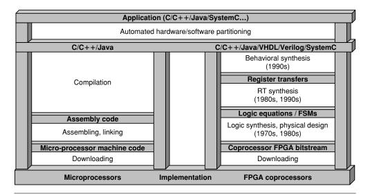
**FIGURE 26.2** The codesign ladder: evolution toward automated hardware/software partitioning due to synthesis tools and FPGA technologies enabling a similar design starting point, and similar implementation manner of downloading bits into a prefabricated device.
