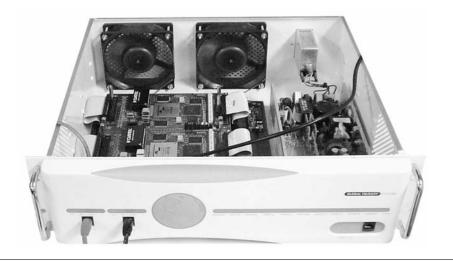
**FIGURE 34.12** FPX modules integrated in a rack-mount chassis.
