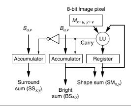
FIGURE 28.9 ■ Computation logic for equations 28.1, 28.3, and 28.4.
