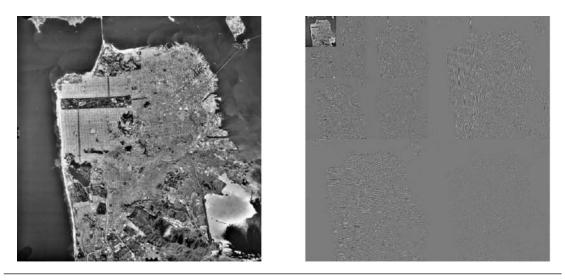
FIGURE 27.3 ■ An image of San Francisco (a) and the resulting 3-level DWT (b).
