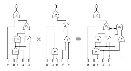
FIGURE 13.4 ■ Combining networks to create a choice network.
