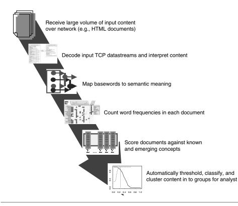
**FIGURE 34.10** Dataflow for the semantic processing system.
