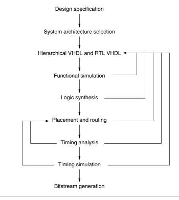
FIGURE 6.7 ■ FPGA compilation flow.
