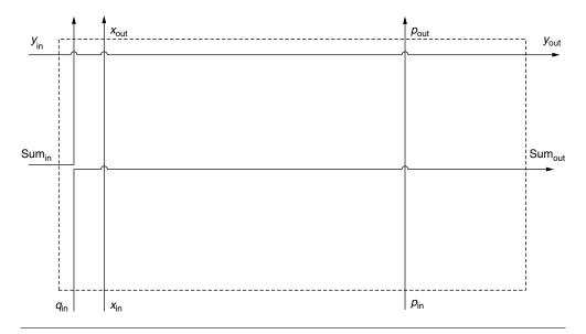
**FIGURE 22.9** The impact of partial evaluation on multiplier cell logic when  $X_{in}$  = False.
