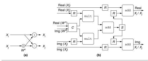
**FIGURE 31.11** ■ Basic butterfly operation (a) and basic butterfly datapath (b). The component S is a switch that directs inputs to alternate outputs. The components marked as R replicate the input once and C is a crossover to facilitate the complex multiply.
