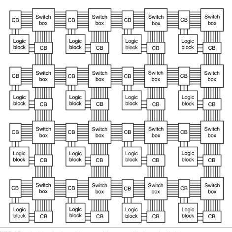
**FIGURE 1.5** • An island-style architecture with connect blocks and switch boxes to support more complex routing structures. (The difference in relative sizes of the blocks is for visual differentiation.)
