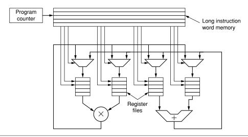
**FIGURE 5.10** VLIW-style control of a single multiply and add datapath.
