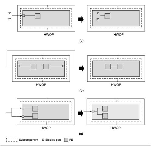
FIGURE 15.21 Context-sensitive optimizations performed by Ye et al. [23].
