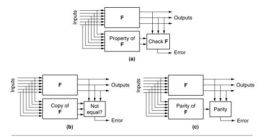
**FIGURE 37.8** A concurrent error-detection strategy and options: (a) generic formulation, (b) duplication, and (c) parity.
