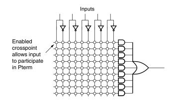
FIGURE 37.6 ■ A PAL OR-term with a collection of substitutable Pterm inputs.
