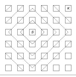
**FIGURE 20.3** A conventional routing search wave.
