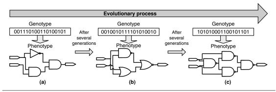
FIGURE 33.3 ■ The evolutionary design of digital circuits: (a) intial random circuit, (b) intermediate circuit, and (c) final circuit.
