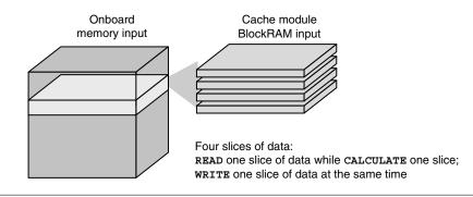
FIGURE 32.13 ■ A structural diagram of the 4-slice caching design.
