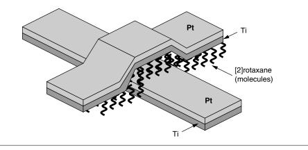
FIGURE 38.4 ■ Switchable molecules sandwiched between nanoscale wires.
