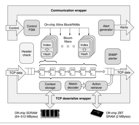
FIGURE 34.9 ■ A block diagram of SIFT.
