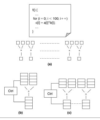
**FIGURE 26.7** Alternative region implementations for an original application (*top*) requiring 100 multiplications: (a) 100 multipliers; (b) 1 multiplier; (c) 2 multipliers. Alternative region implementations may have hugely different performances and sizes.
