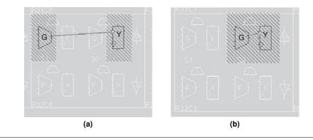
FIGURE 16.7 ■ The overlay combinator: (a) AND2 >-> FD clk; (b) AND2 >l> FD clk.
