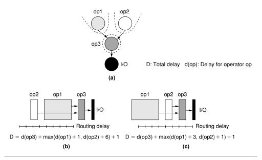
FIGURE 15.15 Simultaneous tree covering and placement.
