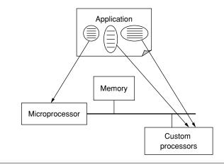
**FIGURE 26.1** ■ A diagram of hardware/software partitioning, which divides an application between a microprocessor component ("software") and custom processor components ("hardware").
