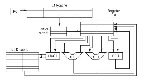
**FIGURE 5.11** A super-scalar processor with an RFU.
