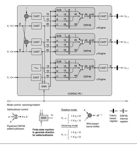
FIGURE 25.12 ■ Processing element *i* of a Virtex-4 DSP48-based CORDIC processor.
