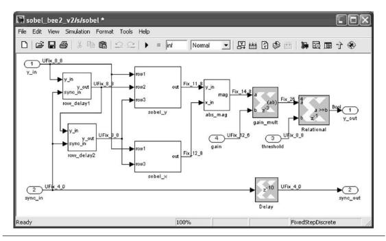
**FIGURE 8.3** ■ The Sobel edge detection filter, processing an 8-bit video datastream to produce a stream of Boolean values indicating edges in the image.
