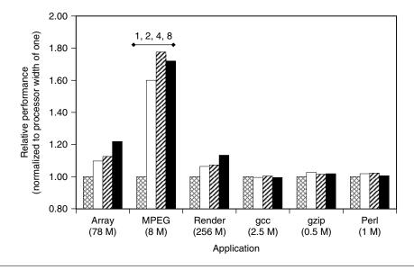
FIGURE 35.15 ■ Performance of multiplexing versus VLIW processor width.
