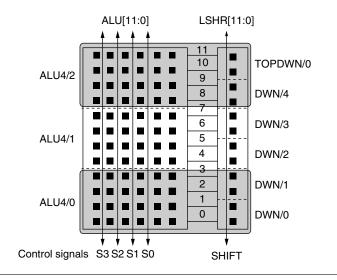
FIGURE 15.19 Extracting inter-HWOP regularity.
