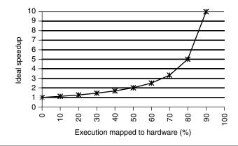
FIGURE 26.3 ■ Hardware/software partitioning speedup following Amdahl's Law.
