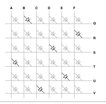
FIGURE 38.6 ■ An example crossbar routing configuration.
