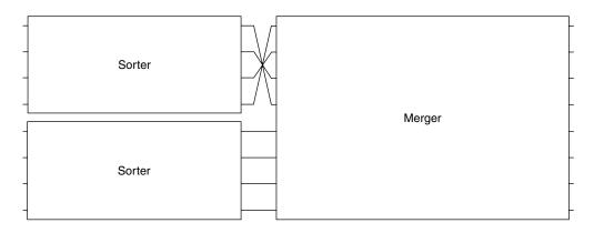
**FIGURE 16.11** The recursive structure of a sorter.
