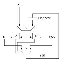
FIGURE 36.7 Saturated accumulator cyclic dependency.
