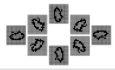
**FIGURE 28.5** ■ Example of eight rotation templates of a SAR 16 × 16 bitmap image.
