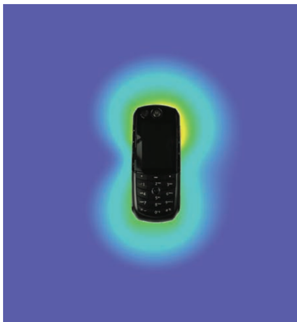
Figure 1.1 Antenna near-field radiation of a mobile phone (courtesy Prof. D. Manteuffel, Univ. Kiel, Germany).
