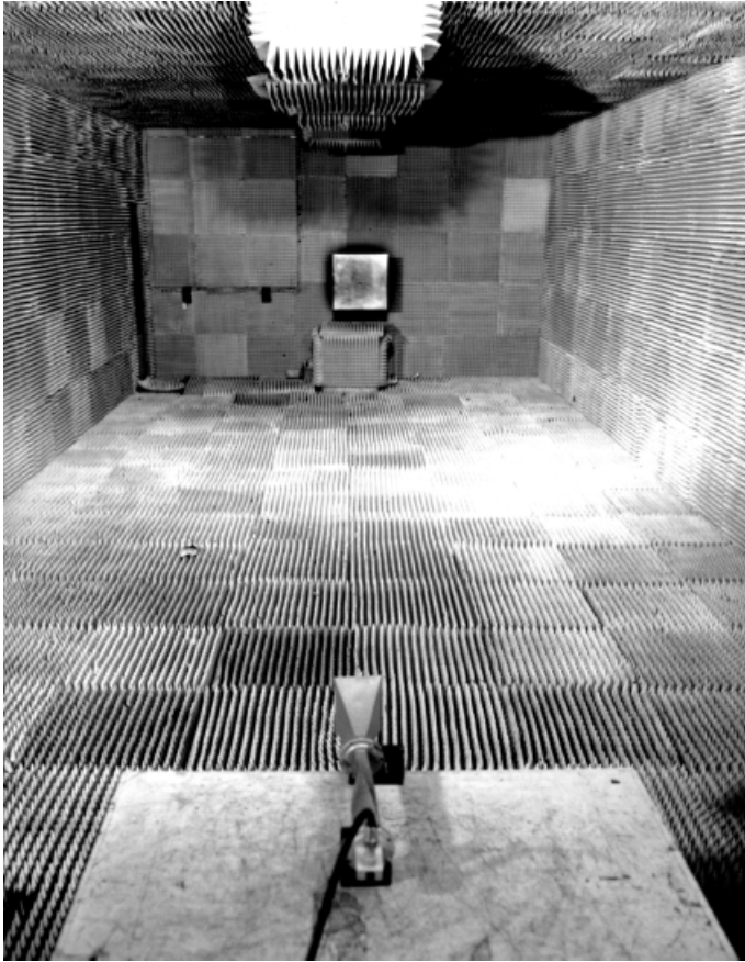
FIGURE 3.36 Standard indoor anechoic chamber at Texas A&M University.
