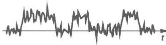
Figure 2.20 Binary signal corrupted by noise.
