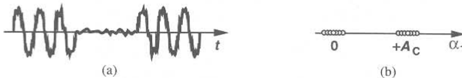
Figure 3.15 Effect of noise on (a) an ASK signal and (b) its constellation.
