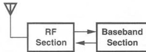
Figure 1.3 RF and baseband processing in a transceiver.
