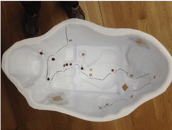
FIGURE 6-72 Richard streamlined his handmade Clouds with a vacuum-formed shell template with specific holes for LEDs and speaker outputs; the electronics fit into the shell perfectly
