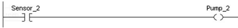
Figure 3-4 Normally open contact. Real-world input Sensor_2 is false so the normally open contact is not energized. The rung is false and the output is off.
