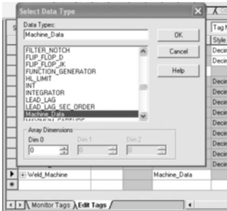
Figure 2-22 The programmer entered a new tag name (Weld_Machine) and chose Machine_Data as the type.
