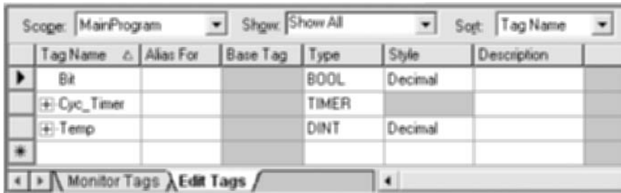
Figure 2-13 Tag editor screen. Note that three tags have been defined. Bit is a BOOL-type tag. Cyc_Timer is a TIMER-type tag. Temp is a DINT-type tag. Note the scope of these tags is program scope (named MainProgram). Note also that the two selection tabs at the bottom are Monitor Tags and Edit Tags and that the Edit Tags tab is active.
