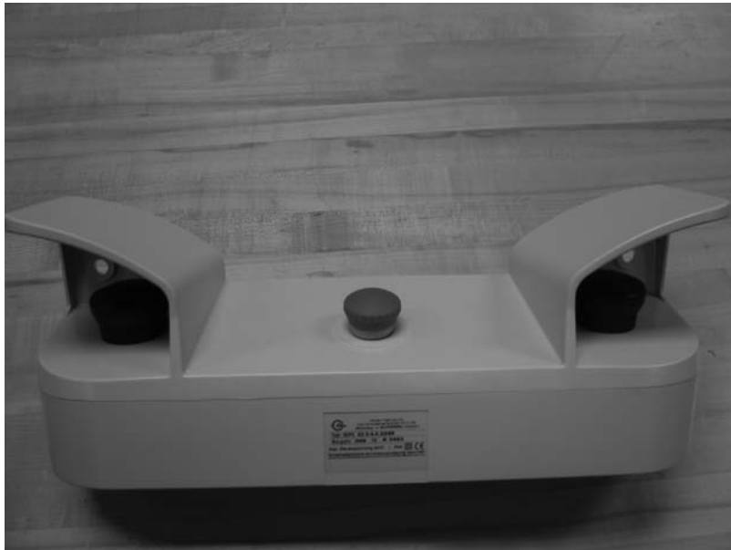
Figure 3-14 A two-hand safety switch. The two hand switches are on the left and the right of the photo.
