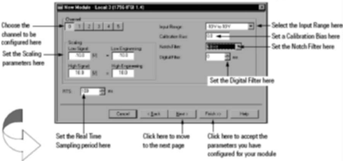
Figure 5-21 Configuring channels in an analog module. (Courtesy of Rockwell Automation, Inc.)
