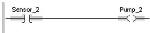
Figure 3-5 Normally open contact. Real-world input Sensor_2 is true so normally open contact is energized. Thus the rung is true, and the output is on.
