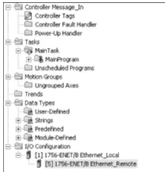
Figure D-10 Controller Organizer screen after the Ethernet (Ethernet_Remote) module was added.
