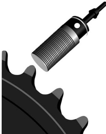
Figure 6-53 An inductive sensor used to sense teeth on a gear. (Courtesy ifm efector inc.)
