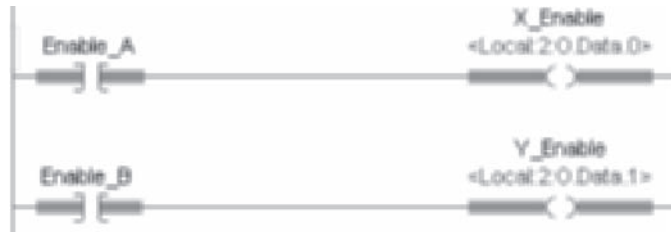
Figure E-30 Logic to enable the two drives. Note that the outputs from the output module are connected to the drive enable input on each drive.
