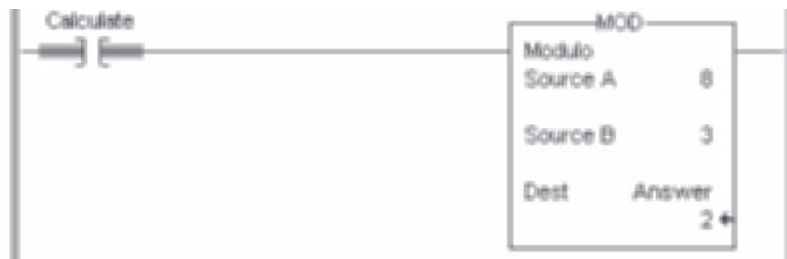
Figure 7-8 Use of a MOD instruction in RSLogix 5000.
