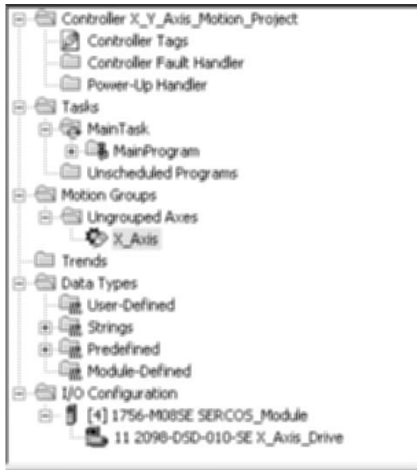
Figure E-11 Controller Organizer screen after the drive and tag were added for the X_Axis.
