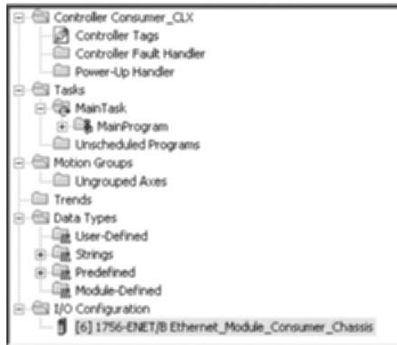
Figure C-8 Controller Organizer after the module was added.
