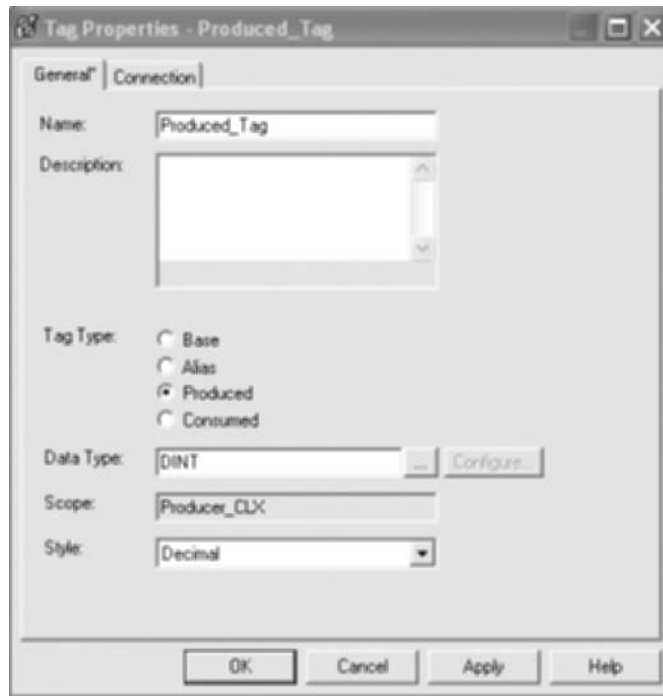
Figure C-2 Tag Properties screen for the tag. Note that the Tag Type is Produced. Note also the Connection tab on top of the screen.
