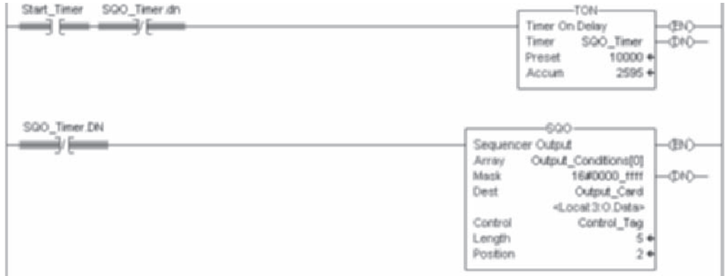
Figure 8-19 Simple SGO instruction ladder logic.
