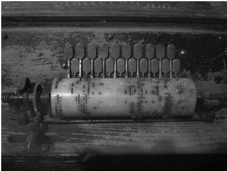
Figure 8-17 Music organ (drum controlled). Note the pegs that activate the valves as the drum is turned at slow speed.
