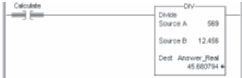
Figure 7-4 Use of a DIV instruction. In this example the result is a decimal number because the Dest tag is a Real.
