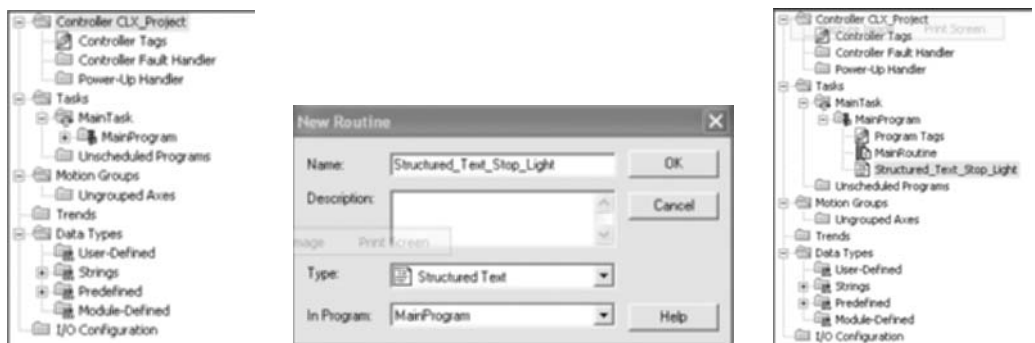
Figure 9-2 On the left is the Controller Organizer. If you right-click on MainProgram , you can create a new routine. In the center is the New Routine configuration screen. Note that Structured Text was chosen for the language Type. The figure on the right shows the Controller Organizer after the new routine was created. After the new routine is chosen, you can click on the name of the routine in the main program list and the screen shown in Figure 9-3 will appear.
