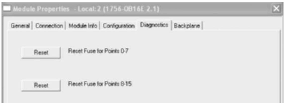
Figure 5-18 Resetting fuses in the programming software.
