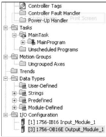
Figure A-13 Controller Organizer after an input and an output module were added.
