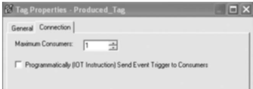
Figure C-3 Tag Properties, Connection parameters. In this example only one other controller (consumer) will be allowed to get the data for this tag because 1 was entered in Maximum Consumers.
