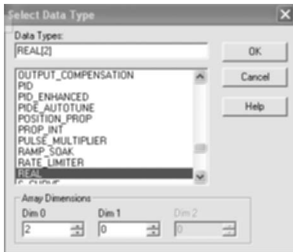
Figure 13-32 Declaring the data type for the tag array that will hold the X and Y position to move to.
