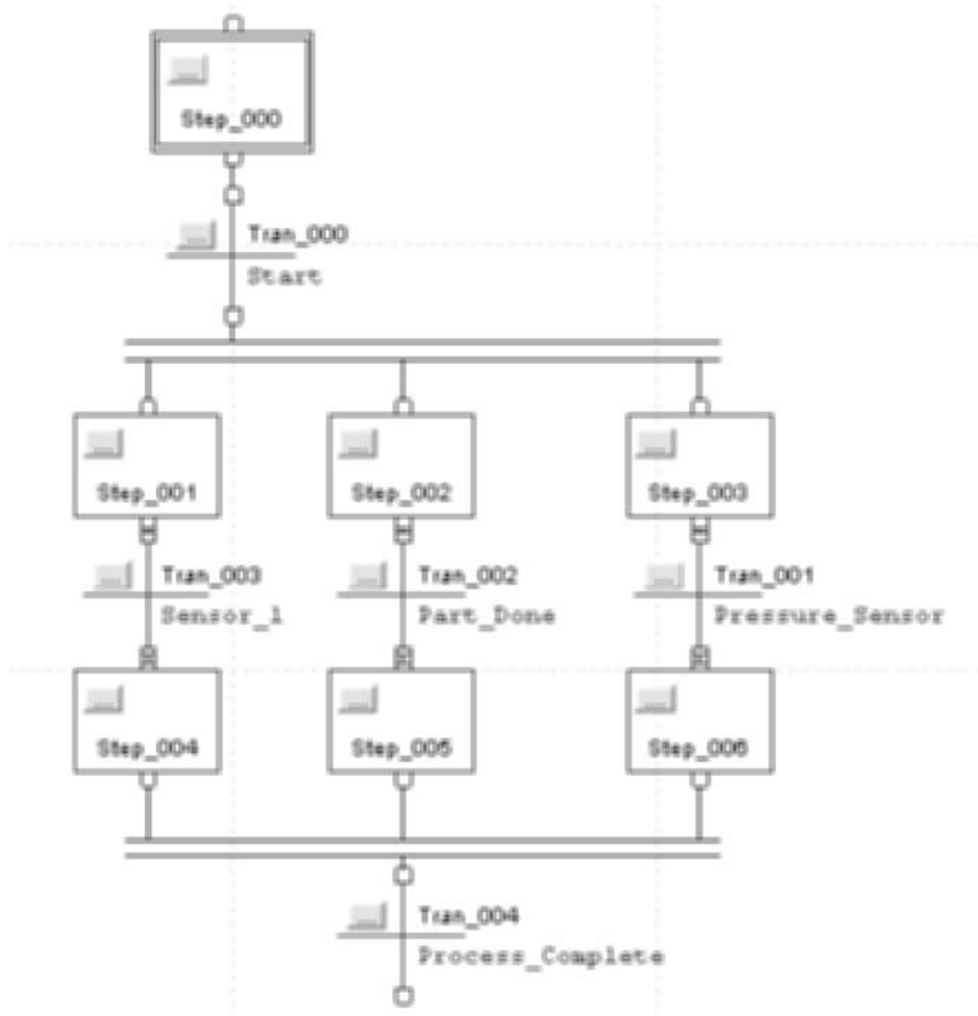
Figure 10-51 A simultaneous branch SFC.
