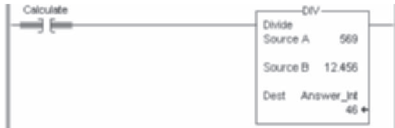
Figure 7-3 Use of a DIV instruction in RSLogix 5000. In this example the result is a whole number because the Dest tag is an Int.
