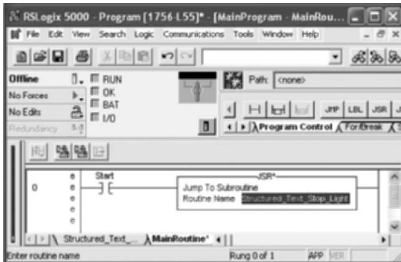
Figure 9-4 A JSR instruction being used to call (run) the ST routine. Note that in this example, the JSR will only be executed while the Start contact is true.
