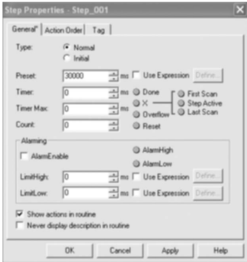
Figure 10-49 Step properties. Note that a Preset of 30000 milliseconds was used to create a 30-second preset.
