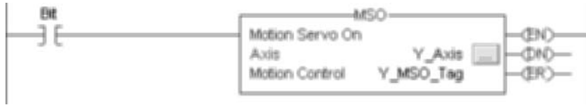
Figure 13-18 Note that in motion commands the axis must be chosen (Y_Axis in this example). A tag of type motion must be created for each instruction.
