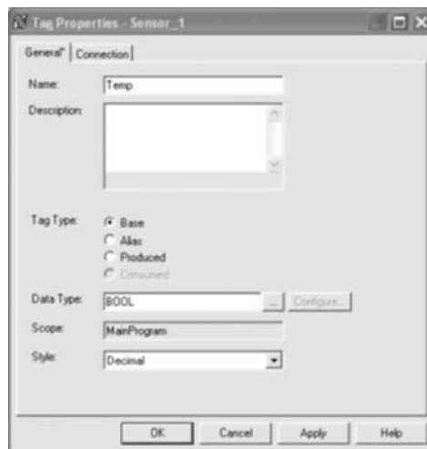
Figure 2-11 How a tag is configured in CLX. Note the choices: Base, Alias, Produced, and Consumed. Note that the programmer also has a choice of the Scope and Style of the tag in this screen.
