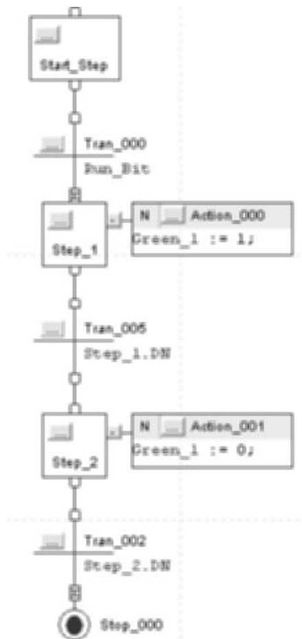
Figure 10-43 Use of a stop element.
