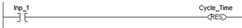
Figure 4-10 Use of a CLX RES instruction to reset a timer’s accumulated time.
