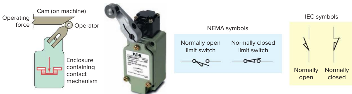
Figure 6-13 Mechanically operated limit switch. Source: Photo courtesy Eaton Corporation.
