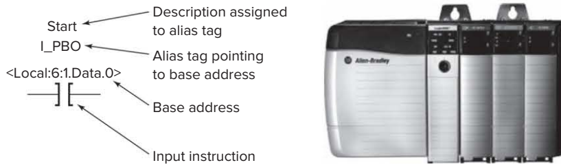
Figure 2-5 Allen-Bradley ControlLogix tag-based addressing format. Source: Image Courtesy of Rockwell Automation, Inc.
