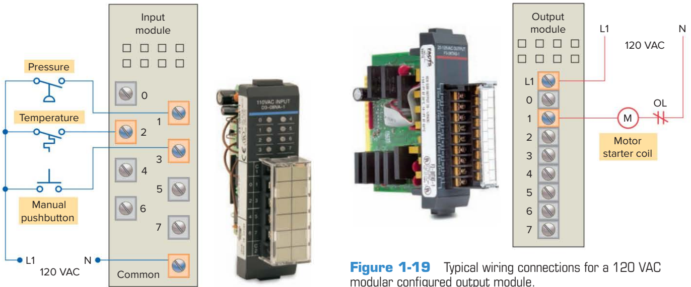
Figure 1-18 Typical wiring connections for a 120 VAC modular configured input module. Source: Photo courtesy Automation Direct, www.automationdirect.com .
