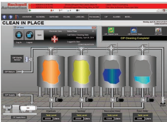
Figure 1-25 Human Machine Interface (HMI) Source: Image Courtesy of Rockwell Automation, Inc.
