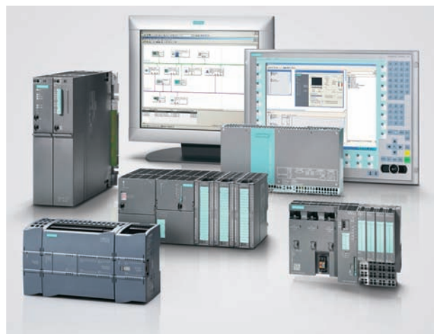
Figure 1-27 Typical range of sizes of programmable controllers. Source: Courtesy Siemens.
