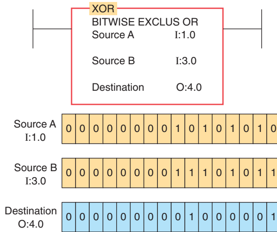
Figure 4-26 Word-level XOR instruction. Source: Image Courtesy of Rockwell Automation, Inc.
