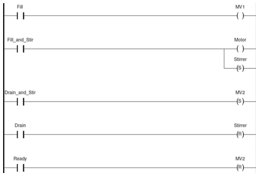
Figure 9.25 Program code based on the state flags
