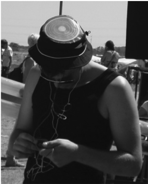
19.13 A photograph of the solar hat comprising sun hat, polymer solar cells and integrated radio. Demonstrated at the Roskilde Music Festival in 2008.
