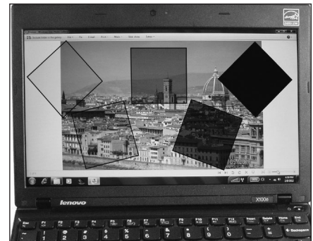
The light from an LCD display is linearly polarized. A number of square polarizers have been placed on the screen of this laptop computer at different angles until the light is totally extinguished. There are five polarizers placed on the screen at different angles.
