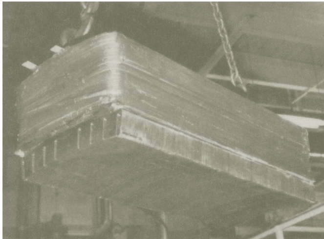
FIGURE 4.25 Shunt field winding.
