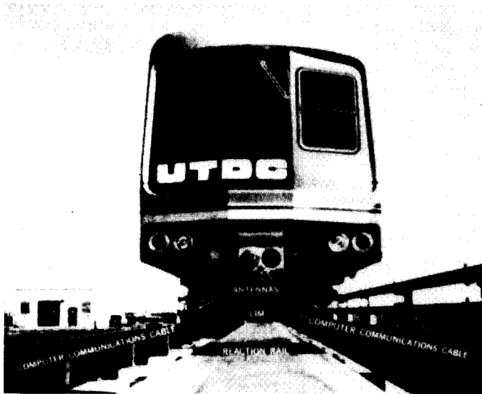
FIGURE 5.49 Transportation test vehicle using LIM. (Courtesy of Urban Transportation Development Corporation, Kingston, Canada.)
