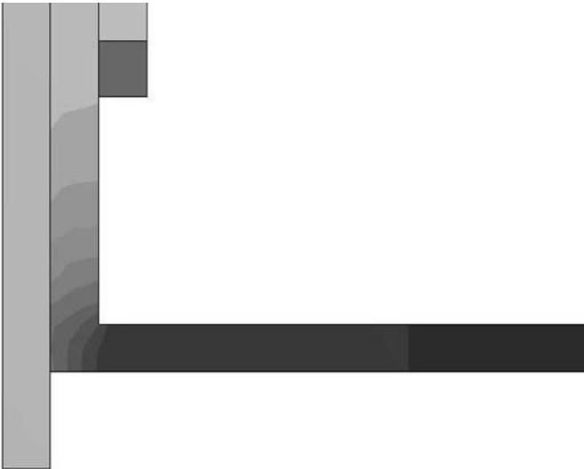
FIGURE A.3 Temperature distribution in the bracket near the bend.
