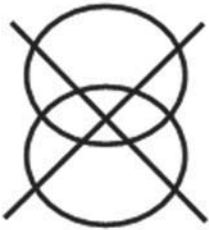
Figure 10.2 Inverter without transformer
