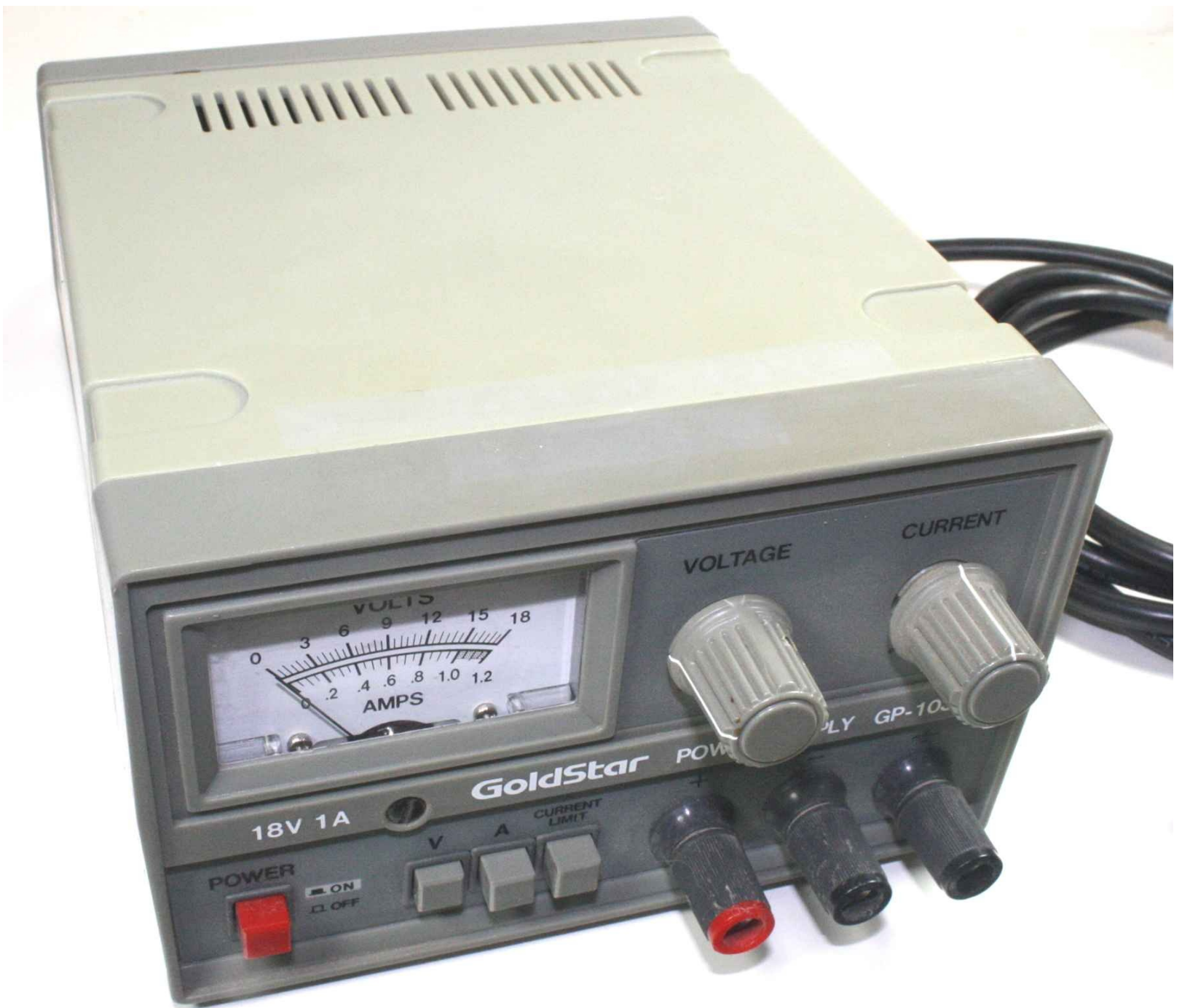
Figure 5-18. Variable-output bench DC power supply
