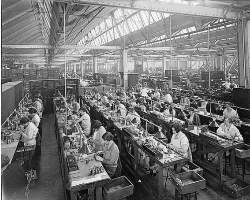
Figure 15-1. A vacuum tube radio assembly line at the Atwater-Kent factory circa 1925 (photograph from Library of Congress)
