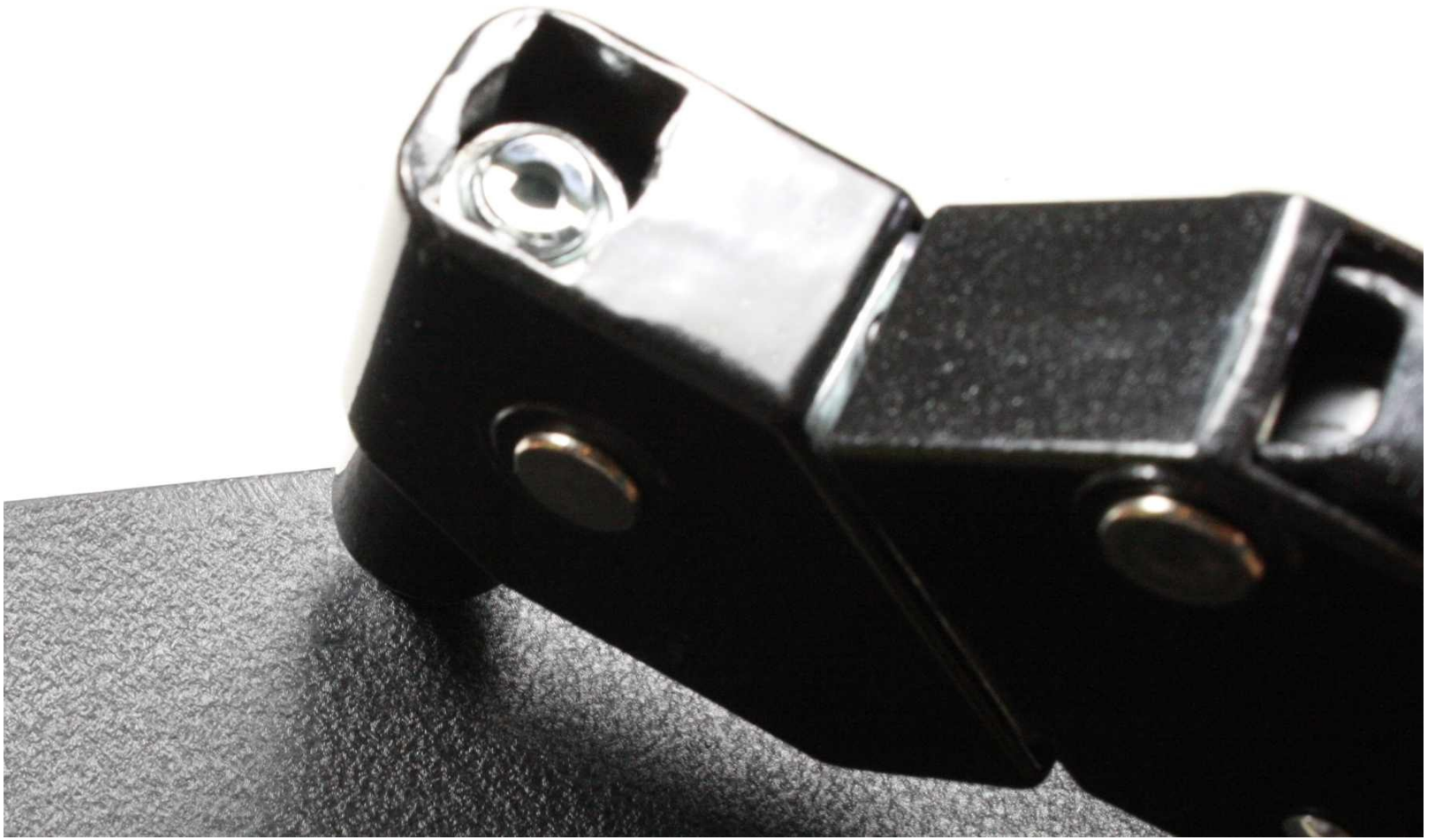
Figure 4-20. Installing a blind rivet: setting the rivet
