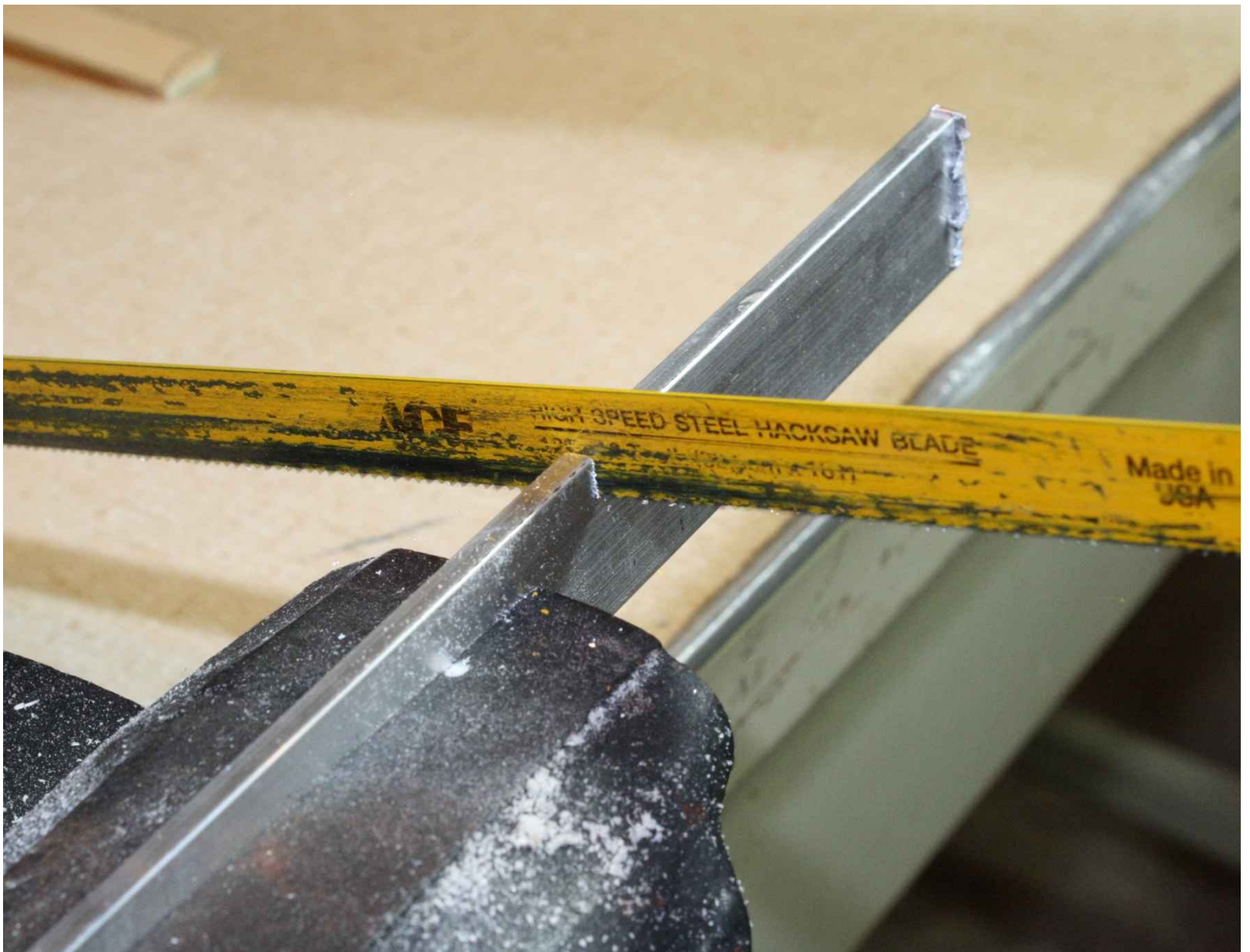
Figure 4-49. Cutting with a hacksaw
