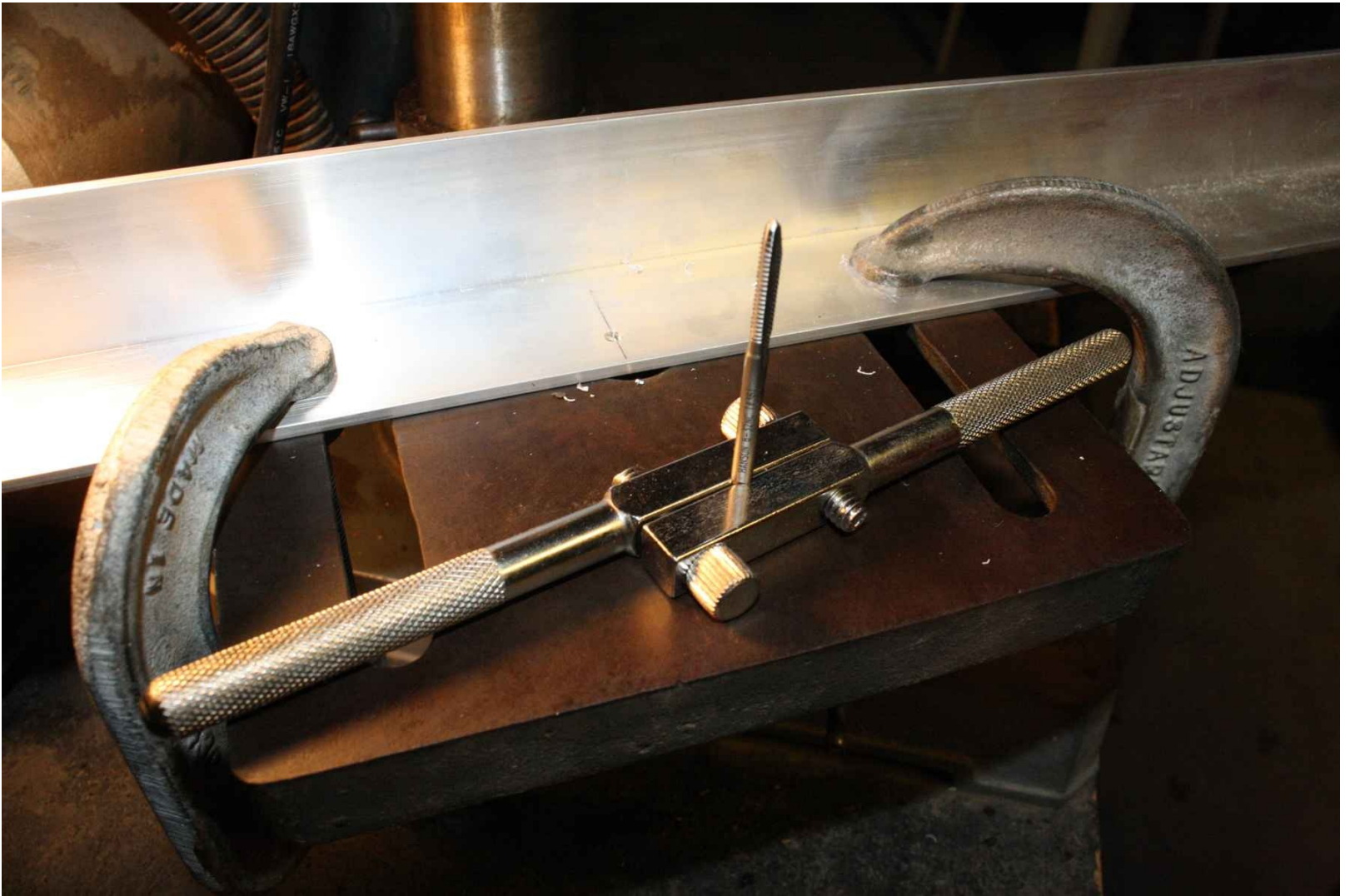
Figure 4-61. Tap mounted in tap handle tool, ready to go
