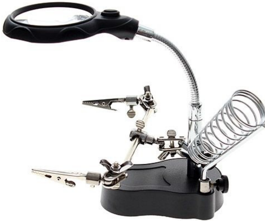
Figure 3-17. A "third-hand" fixture for holding work with small clamps
