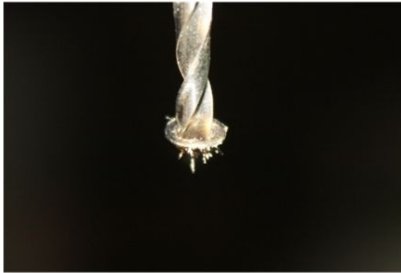
Figure 4-23. Drilling out the head of a counter-sunk screw
