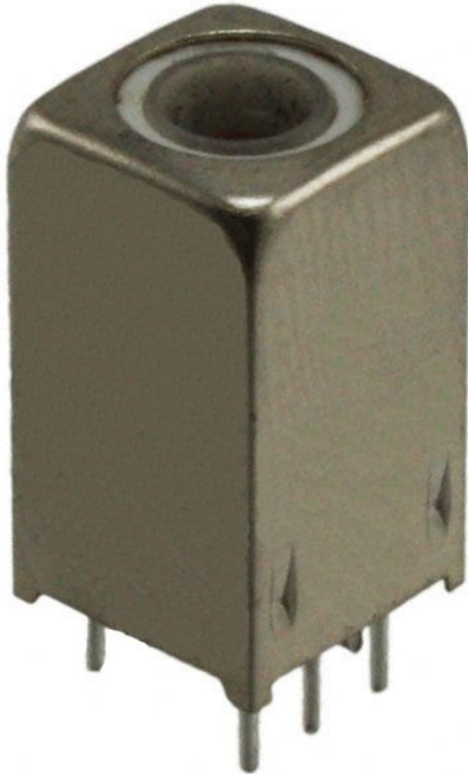
Figure 8-37. Typical PCB-mounted variable inductor
