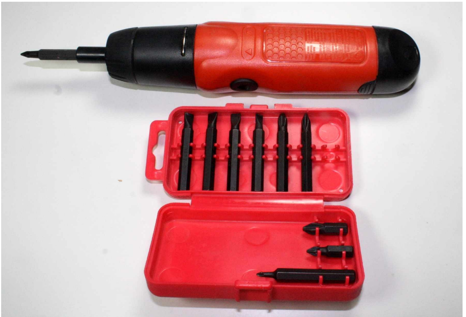
Figure 4-5. Battery-operated electric screwdriver
