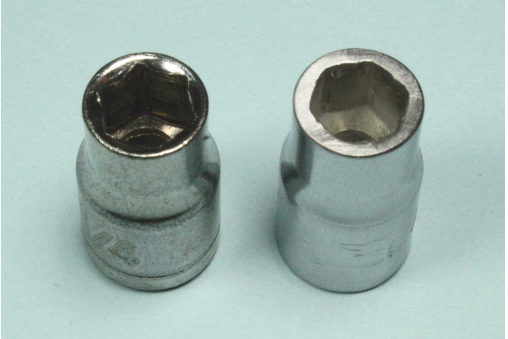
Figure 4-12. Small sockets before and after flush seating modification
