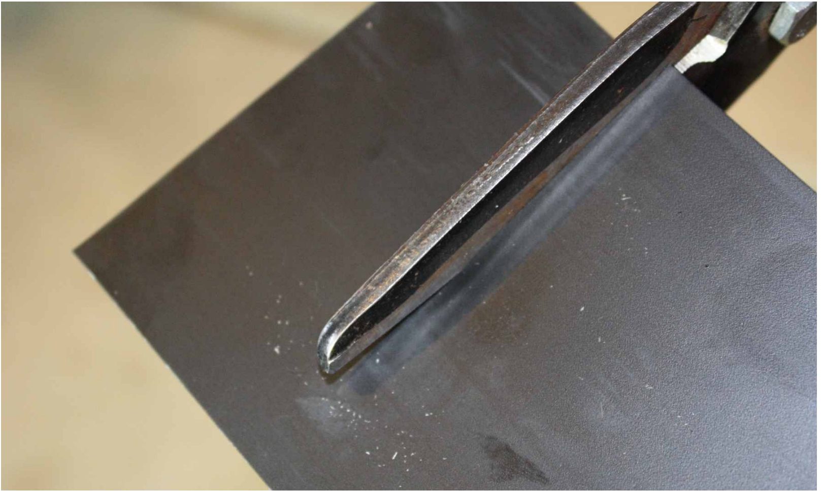
Figure 4-52. Using shop shears on sheet plastic
