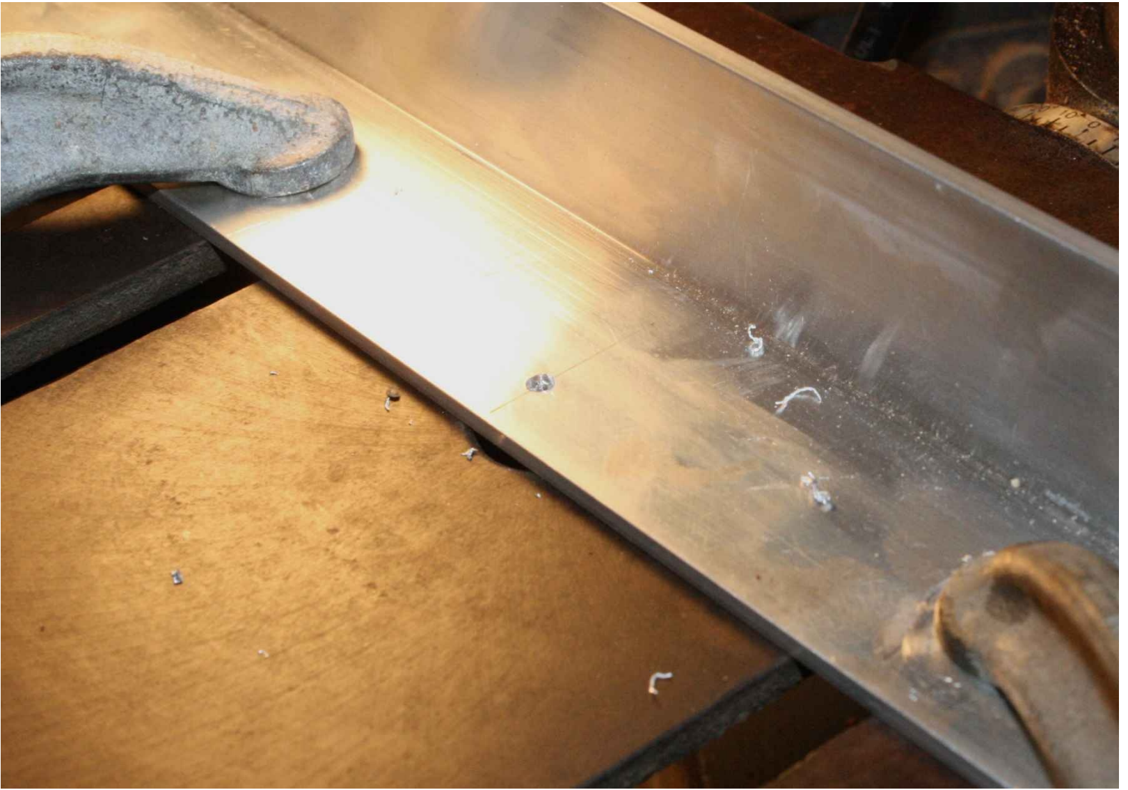
Figure 4-60. Drilled hole ready to tap
