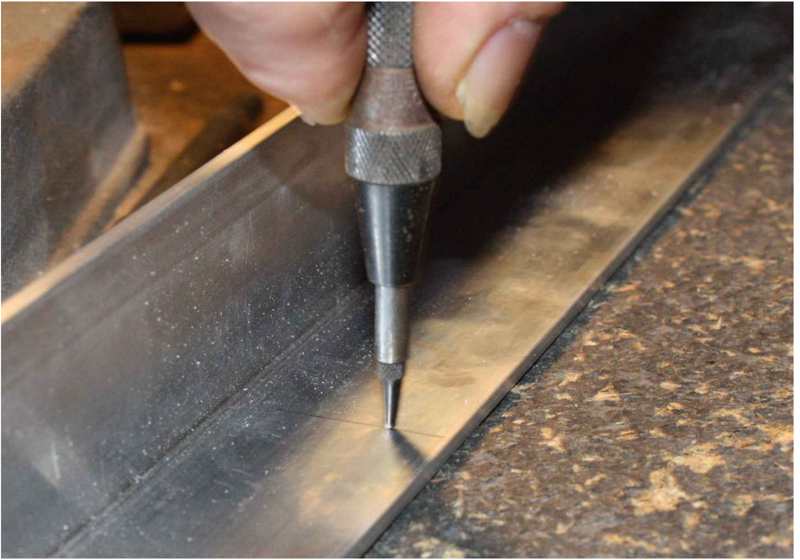
Figure 4-58. Preparing to drill a hole for tapping
