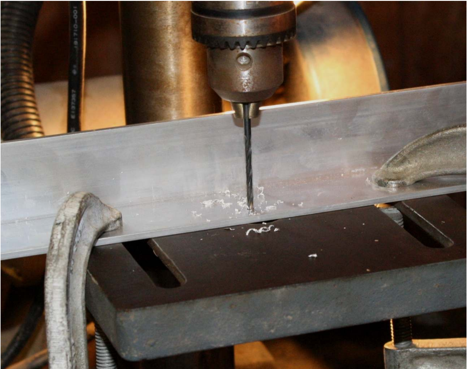
Figure 4-59. Drilling a hole for tapping with a drill press
