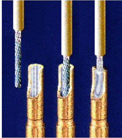
Figure 7-21. NASA-style solder-cup connection
