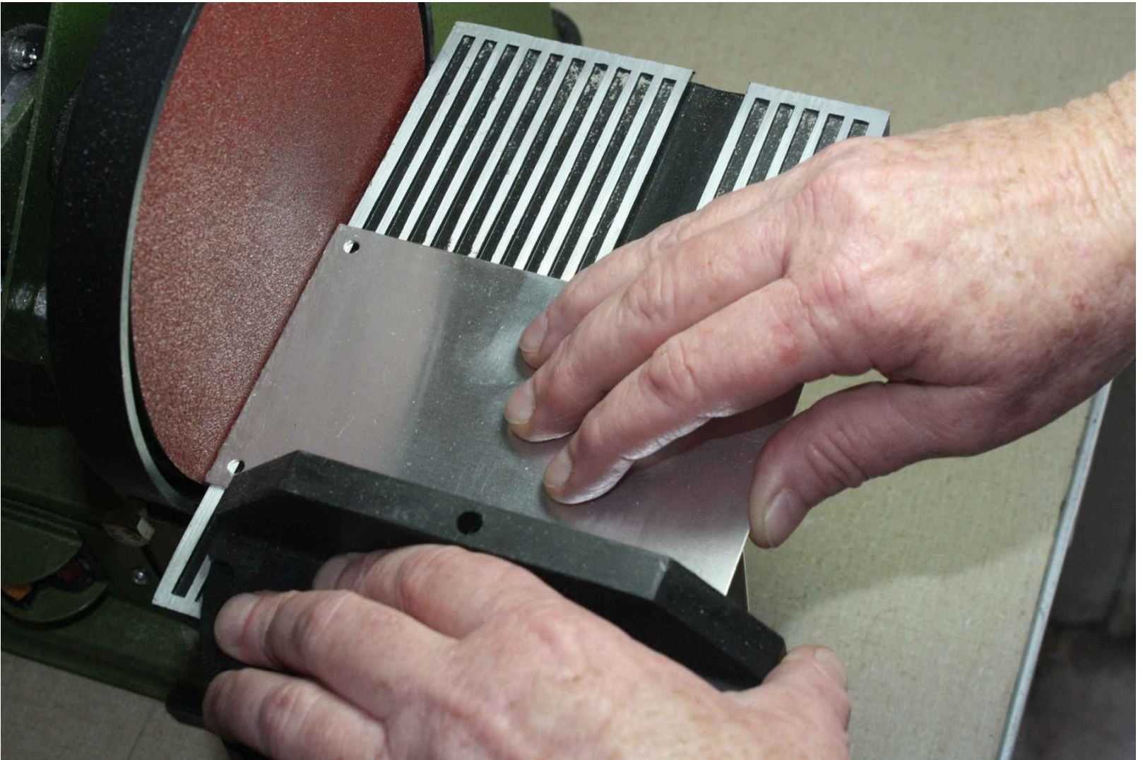
Figure 16-4. Reducing the overall size of a project box cover panel
