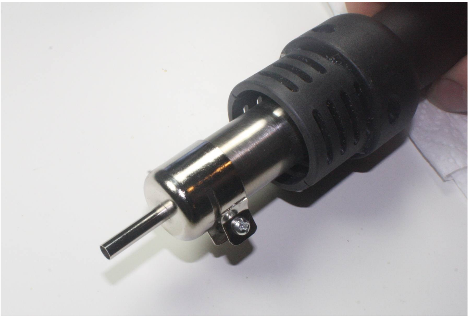
Figure 4-46. Hot-air tool for SMT soldering and desoldering
