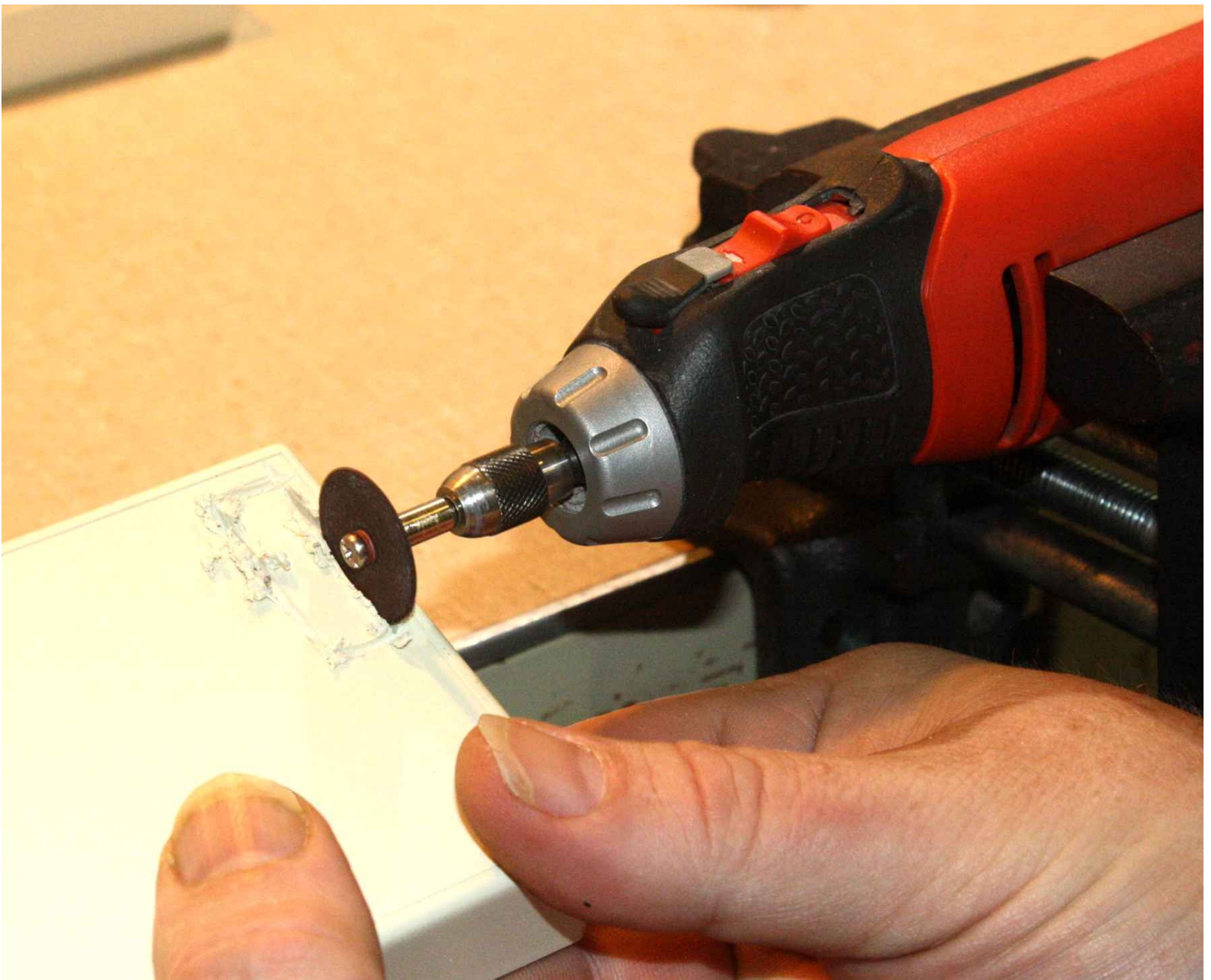
Figure 4-71. Rotary tool in a bench vise
