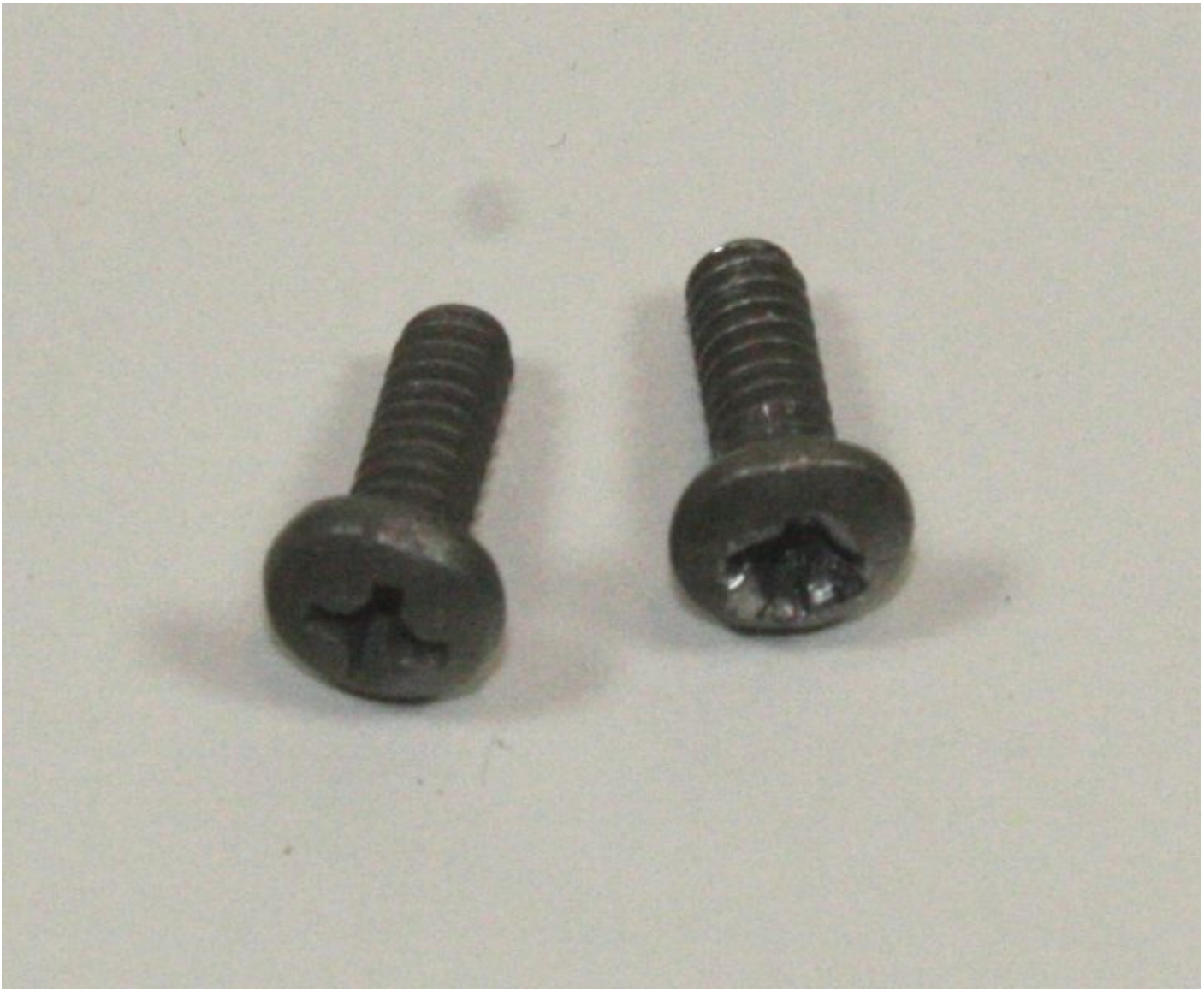
Figure 4-4. Damaged Phillips screw
