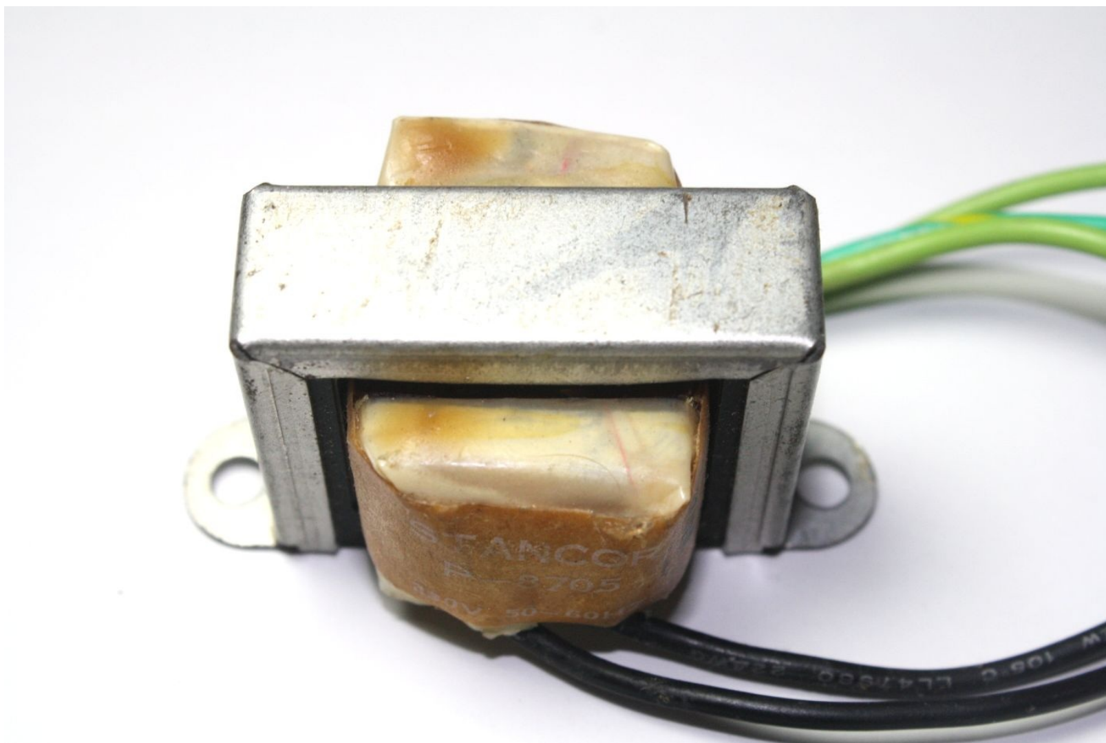
Figure 8-38. A typical small power transformer
