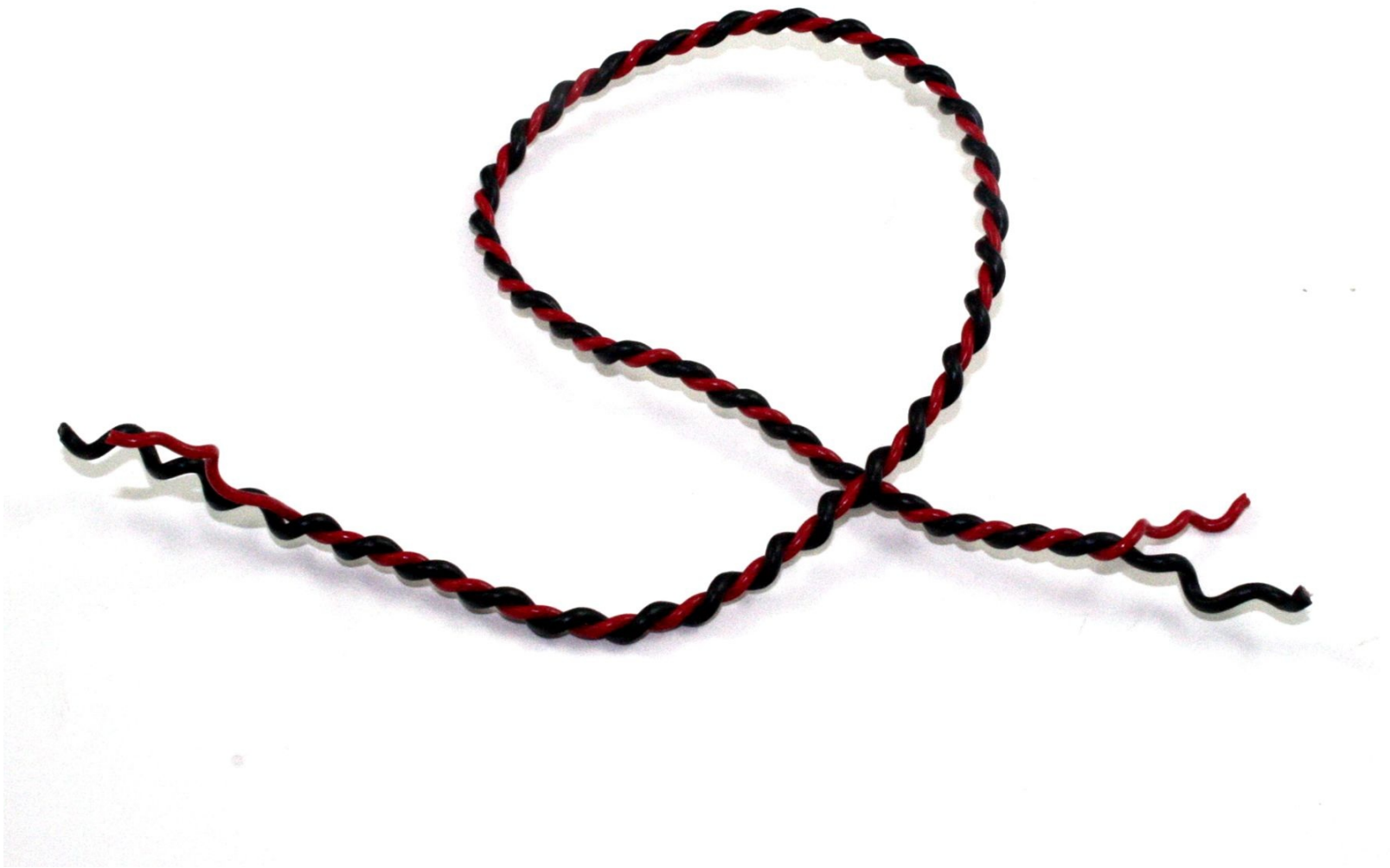
Figure 7-7. Result obtained with the improvised twist tools
