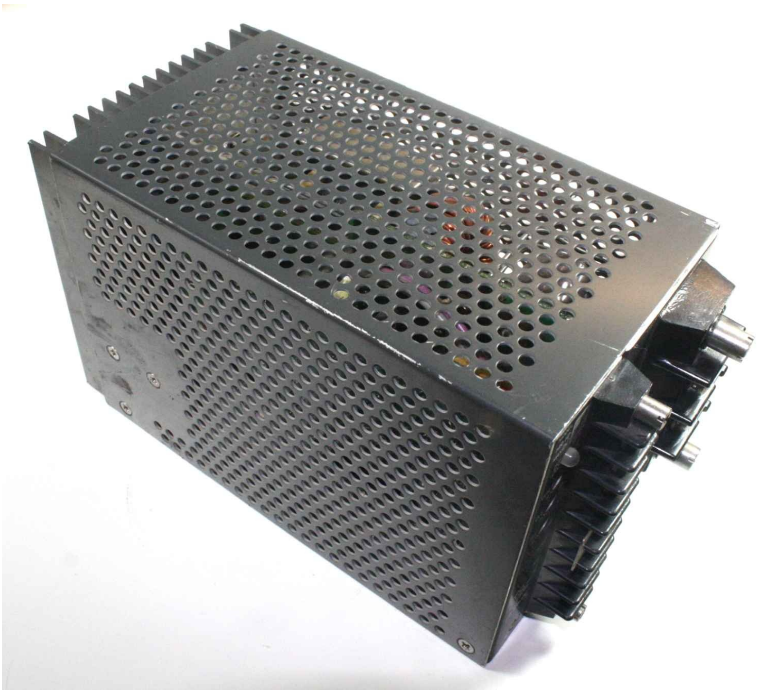
Figure 5-20. Modular 5V DC switching power supply
