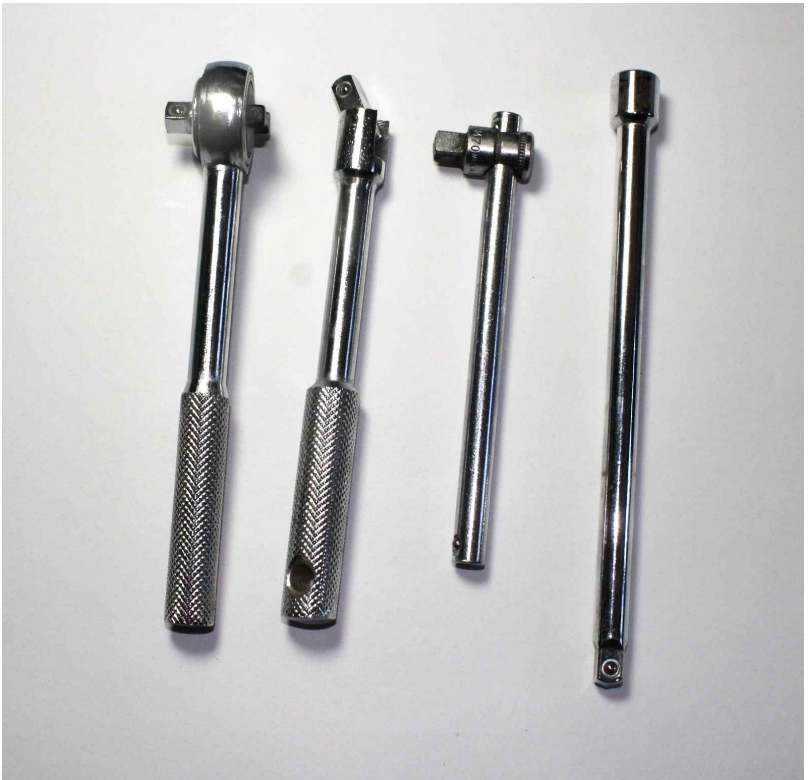
Figure 4-9. 1/4" drive socket handles and extension
