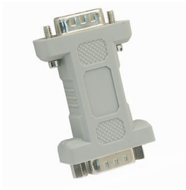
Figure 14-19. A DB-9 RS-232 null-modem adapter
