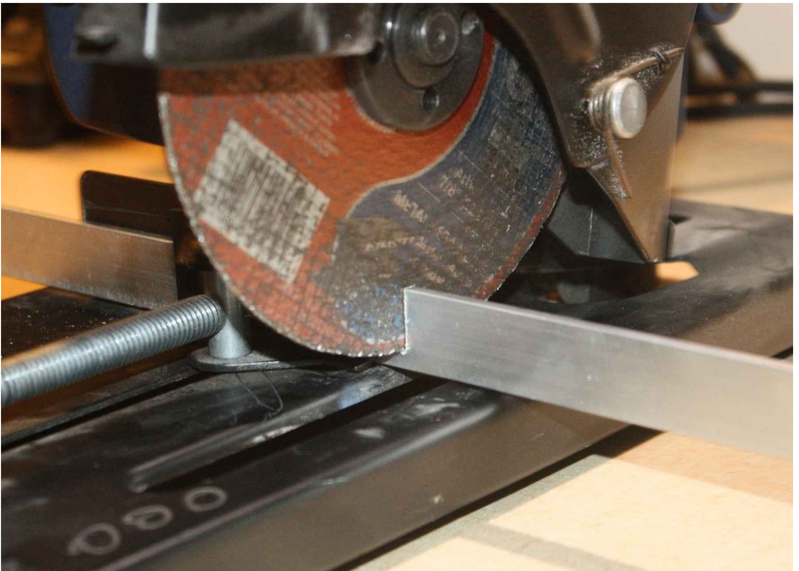
Figure 4-48. Miniature cut-off saw in action
