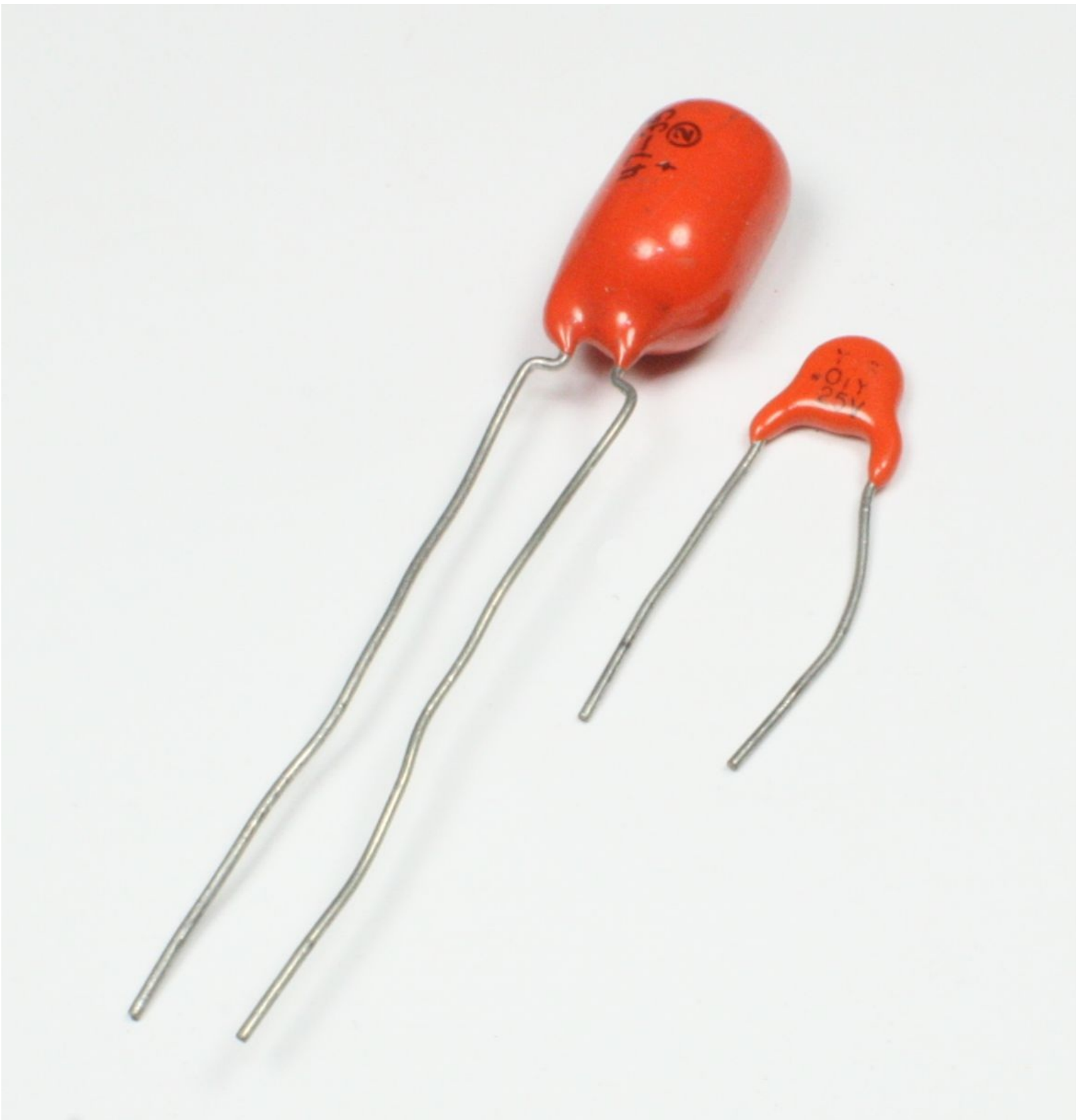
Figure 8-30. A generic example of a tantalum electrolytic capacitor
