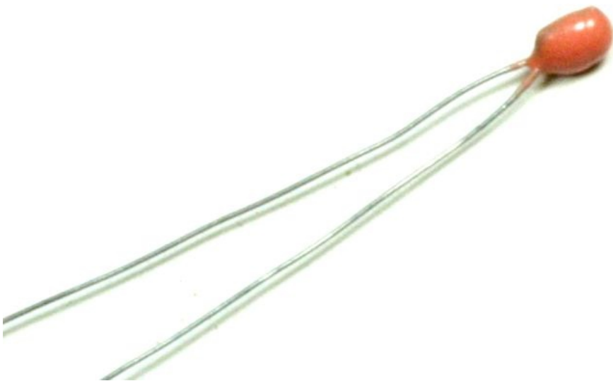
Figure 8-23. Small bead type of NTC thermistor
