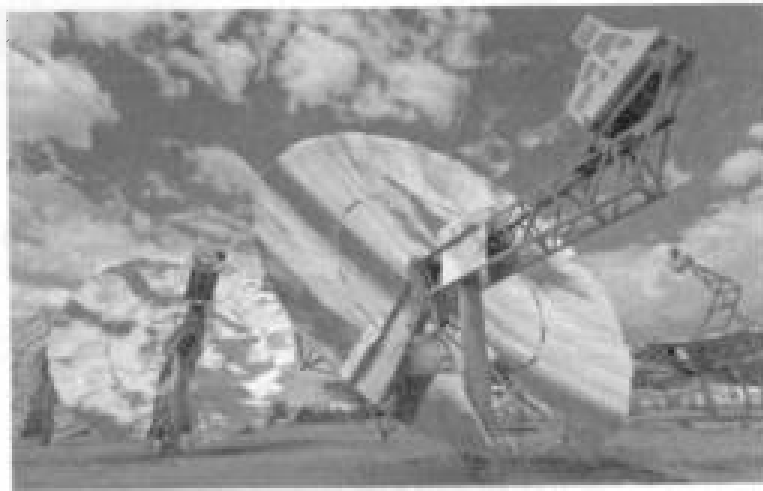
FIGURE 1.11 Dish Stirling systems – SunCatchers by Tessera Solar, "Courtesy of Sandia National Laboratories."
