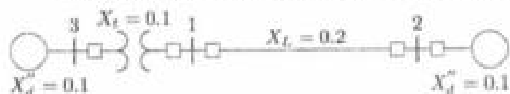
FIGURE 9.20 One-line diagram for Problem 9.3.
