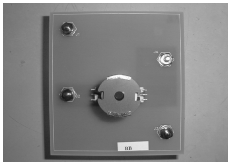
FIGURE 9.4 Pot core mounted on a plug-in board.
