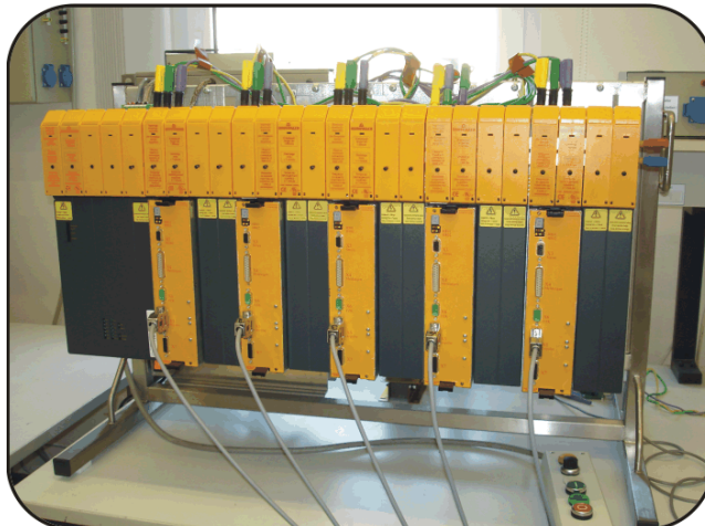
Figure 18A.16 Virtual machine – five inverters in parallel [1]
