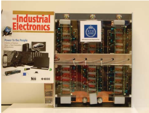
Figure 4.1 40 kVA SiC inverter (300 × 370 × 100 mm) shown together with a copy of the IEEE Industrial Electronics Magazine [1]
