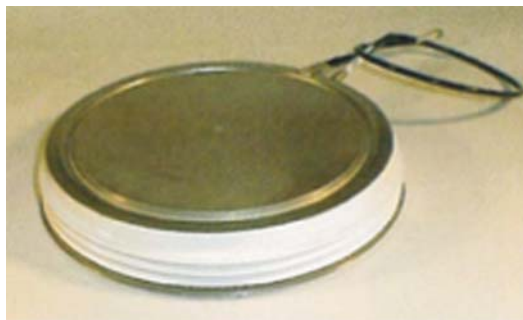
Figure 22.18 IEGT device (Courtesy of Toshiba)
