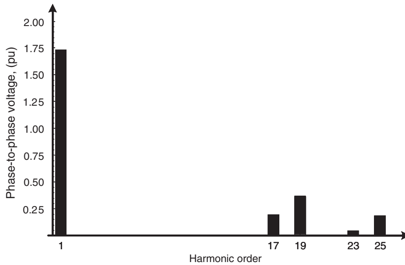
FIGURE 32.26 Line voltage harmonic spectrum for the voltage waveform in Fig. 32.25a.
