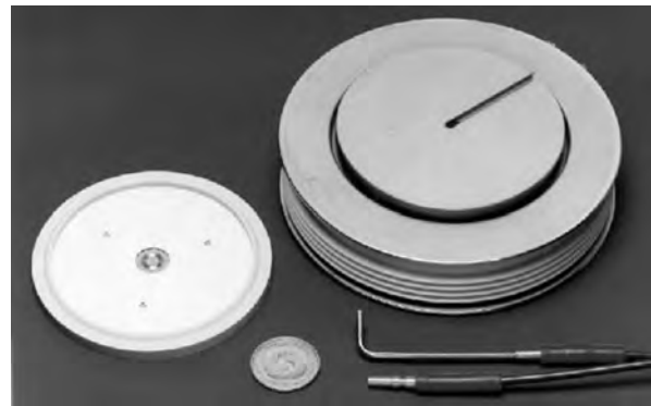
FIGURE 30.24 Silicon wafer and construction of the LTT. The light guides appear in the bottom right-hand corner.
