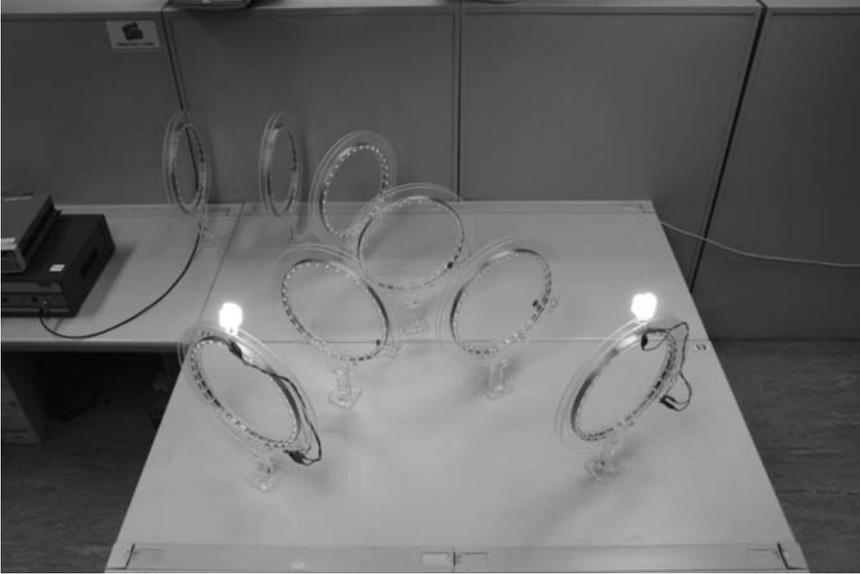
*Figure 19.9 A Y-shaped domino WPT system powering two compact fluorescent lamps*
