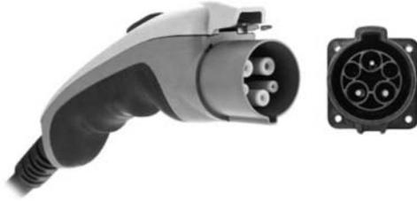
Figure 14.4 Type-1 vehicle and charger Interface
