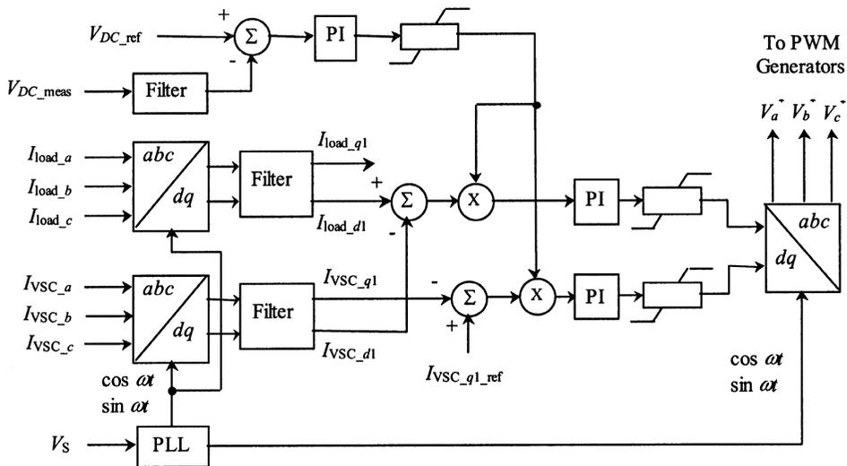
Fig. 8.62 Current controller in the  $dq0$  frame.
