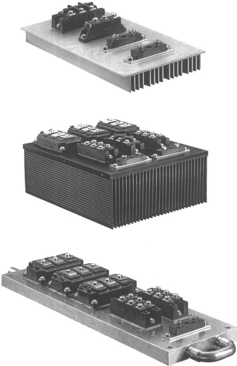
**Fig. 5.13** Heat sinks: (a) air cooled extruded heat sink (velocity = 5 m/s,  $R_{sa} = 0.2$  C/W, weight = 2.6 lb/ft); (b) air cooled fabricated heat sink (velocity = 5 m/s,  $R_{sa} = 0.02$  C/W, weight = 21 lb/ft); and (c) liquid cooled heat sink (flow rate = 5 lt/s,  $R_{sa} = 0.002$  C/W, weight = 4.5 lb/ft). (Courtesy of R-Theta, Inc., Mississauga, Ontario, Canada.)
