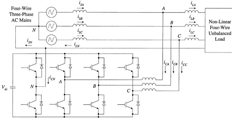
Fig. 6.94 Four-wire four-pole VSC based shunt connected active filter.
