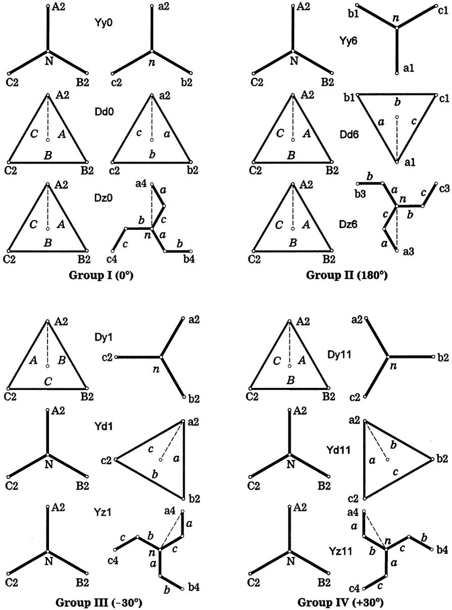
Fig. 2.40 Voltage phasor diagrams of polyphase transformers.
