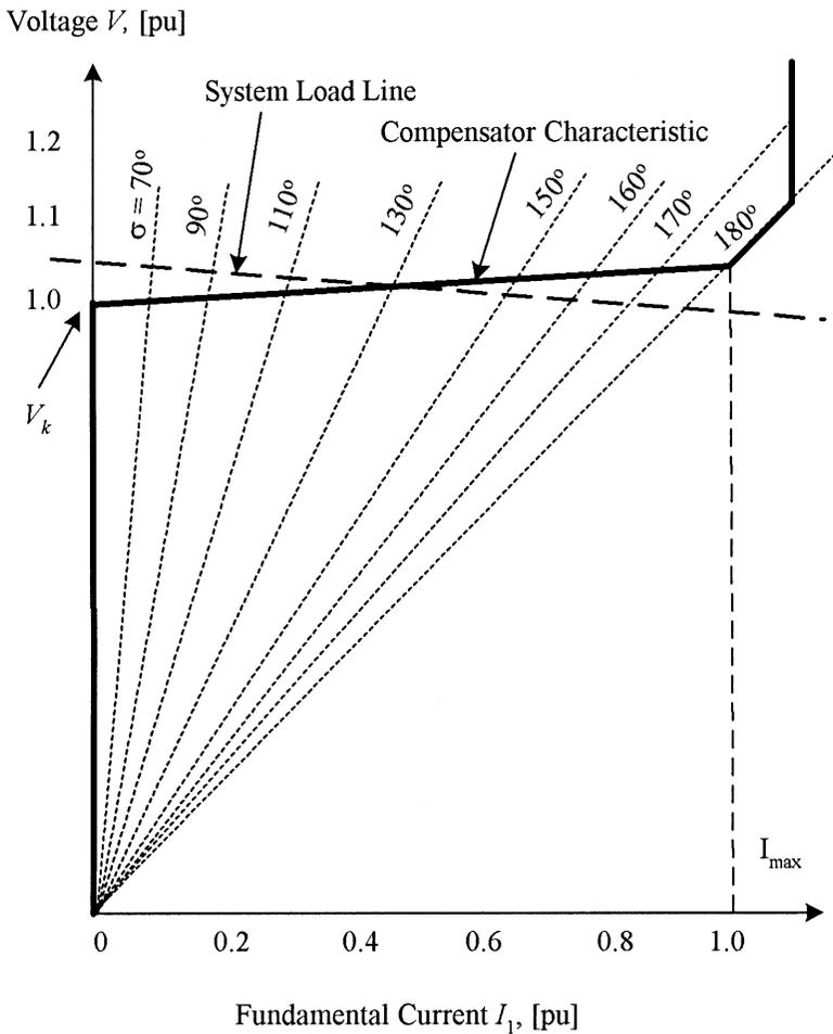
Fig. 6.4 Fundamental voltage/current characteristic in the TCR compensator.
