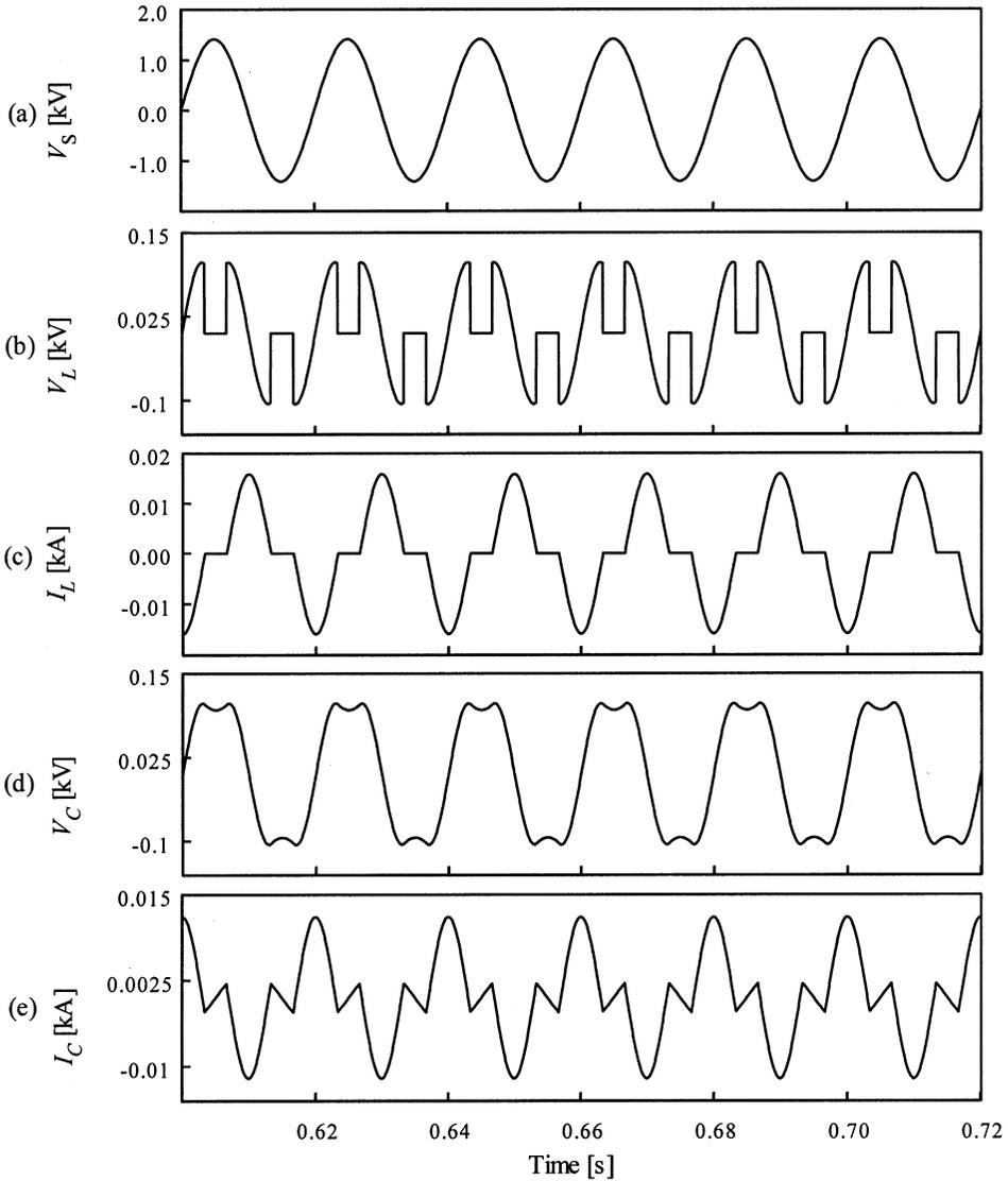
**Fig. 8.28** TCSC characteristic waveforms for the model circuit with  $\alpha = 130^\circ$ . (a) voltage  $V_S$  of the source; (b) voltage  $V_L$  at the TCSC inductor; (c) current  $I_L$  through the TCSC inductor; (d) voltage  $V_C$  at the TCSC capacitor; and (e) current  $I_C$  through the TCSC capacitor.
