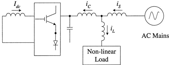
Fig. 6.82 CSC based shunt connected active filter.
