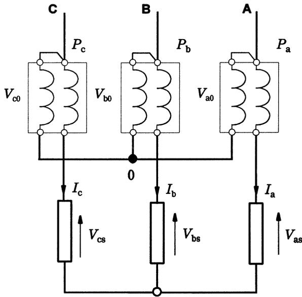
Fig. 2.34 Three-wattmeter connection.
