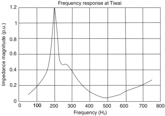
Fig. 7.8 Frequency response impedance as seen from node 1.
