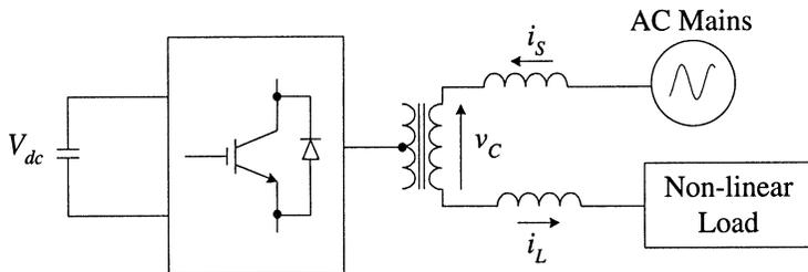
Fig. 6.84 VSC based series connected active filter.
