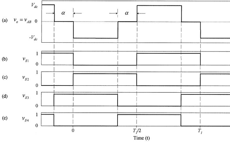
**Fig. 6.29** Key waveforms of the single-phase full-bridge phase-shifted controlled VSC circuit operation. (a) output voltage  $v_o = v_{AB}$ ; (b) control signal for switch  $S_1$ ; (c) control signal for switch  $S_2$ ; (d) control signal for switch  $S_3$ ; and (e) control signal for switch  $S_4$ .
