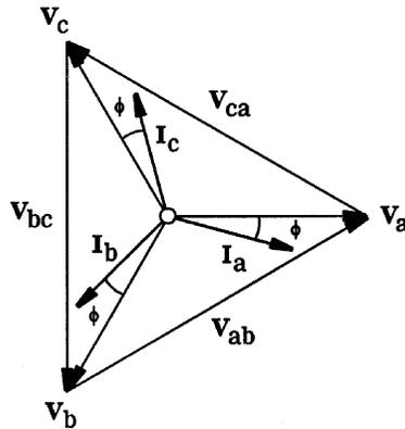
Fig. 2.21 Phasor diagram for balanced wye-connected load.
