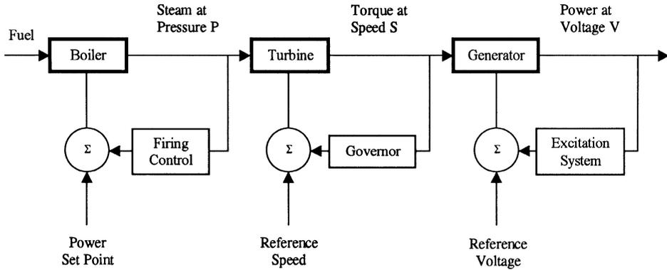
Fig. 1.4 Main controls of a generating unit.
