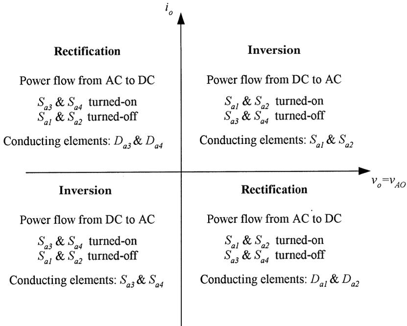
Fig. 6.36 Quadrants of operation of the three-level single-phase half-bridge NPC VSC.
