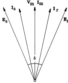
Fig. 3.9 Phasor diagram of symmetrical line.
