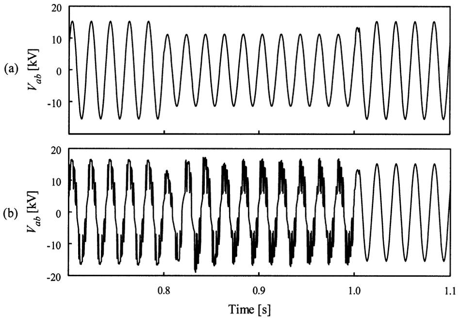
Fig. 8.53 Voltage  $V_{ab}$  at the load point: (a) without D-STATCOM; and (b) with D-STATCOM operating.
