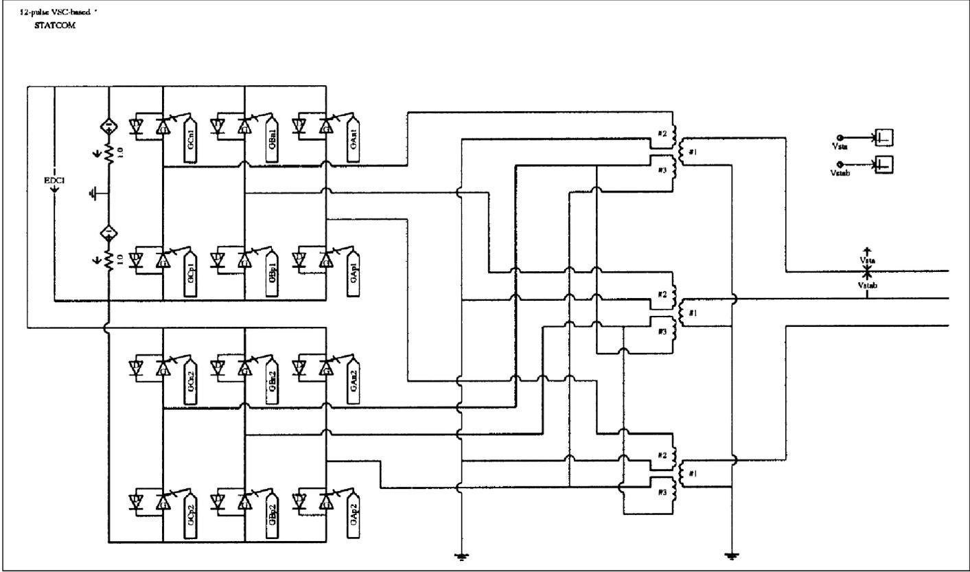
Fig. 8.45 Circuit of a 12-pulse VSC-based STATCOM implemented in PSCAD/EMTDC.
