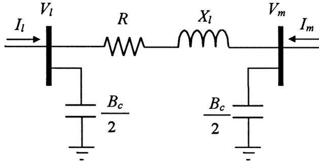
Fig. 4.11 Nominal  $\pi$  representation of the transmission line.
