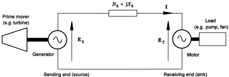
**Fig. 2.16** Transmission system with prime mover, generator, motor and load. The voltages at both ends of the transmission system are assumed to be controlled, so the symbol  $E$  is used instead of  $V$ . At the sending end, the voltage is  $E_s$ ; at the receiving end,  $E_r$ .
