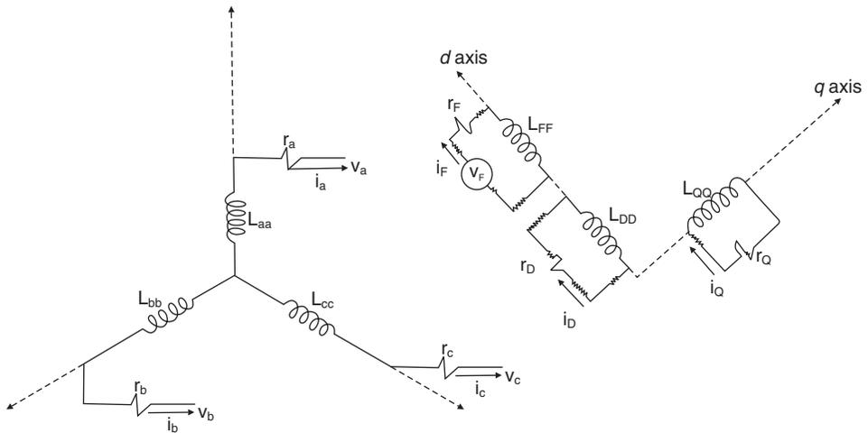
Fig. 1.3 Coupled windings of a synchronous machine.
