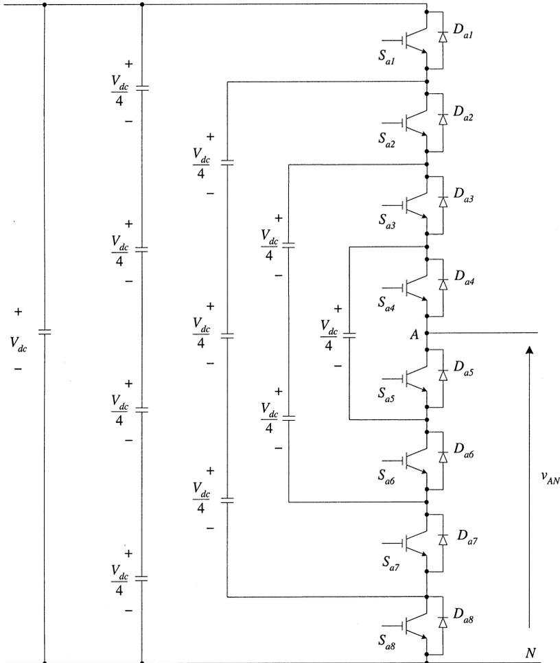
Fig. 6.43 Five-level flying capacitor converter phase leg.
