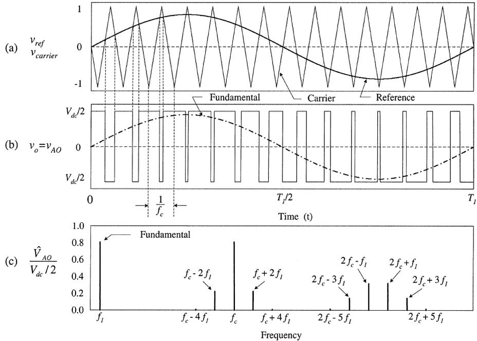
**Fig. 6.47** Two-level sinusoidal PWM method. (a) reference (sinusoidal) and carrier (triangular) signals ( $f_c = 15 \cdot f_1$  and  $M_a = 0.8$ ); (b) voltage waveform  $v_{AO}$ ; and (c) normalized harmonic amplitude of the voltage waveform  $v_{AO}$ .
