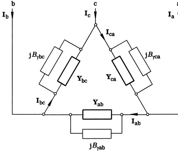
Fig. 2.24 Unbalanced delta-connected load with power-factor correction admittances.
