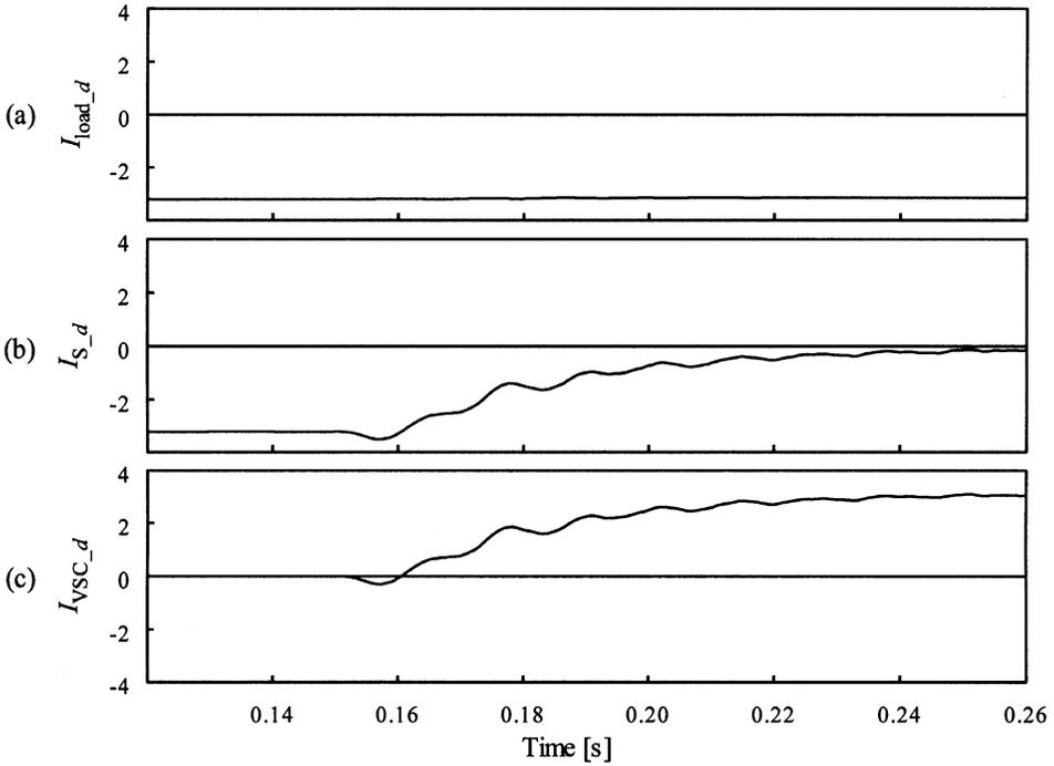
**Fig. 8.69** Reactive components in the rotating frame: (a) load current  $I_{load\_d}$ ; (b) source current  $I_{s\_d}$ ; and (c) converter current  $I_{VSC\_d}$ .
