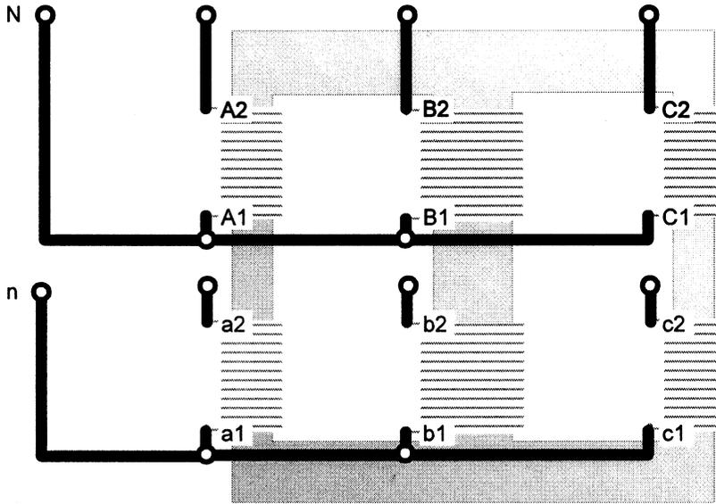
Fig. 2.39 Electrical connections of a Yy0 transformer.
