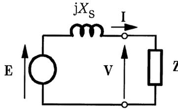
Fig. 9.1 Simple AC circuit.
