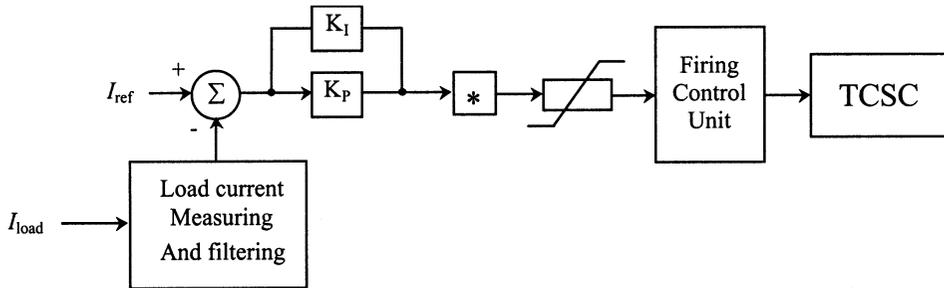
**Fig. 8.30** A typical PI controller for a TCSC.
