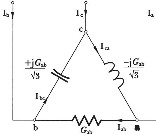
Fig. 2.26 Steinmetz network with balanced line currents.
