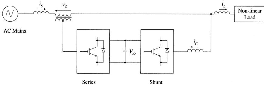
Fig. 6.85 VSC based series/shunt combined active filter.
