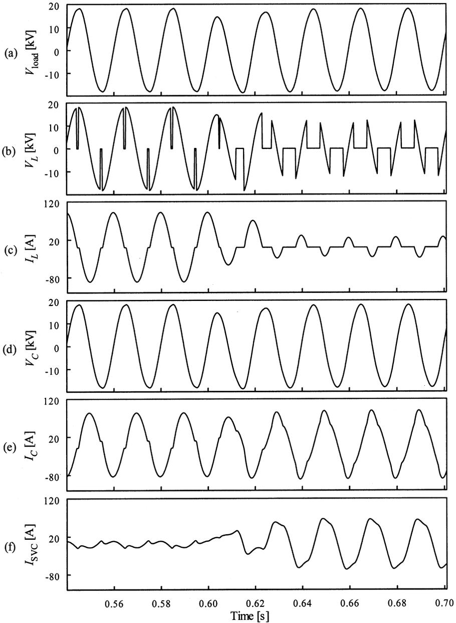
**Fig. 8.24** SVC characteristic waveforms in closed-loop mode: (a) voltage  $V_{load}$  at the load point; (b) voltage  $V_L$  at the SVC inductor; (c) current  $I_L$  through the SVC inductor; (d) voltage  $V_C$  at the SVC capacitor; (e) current  $I_C$  through the SVC capacitor; and (f) total current  $I_{SVC}$  through the SVC.
