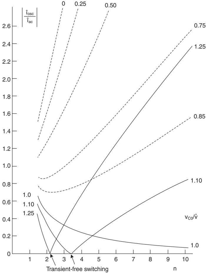
Fig. 6.20 Amplitude of oscillatory current component. Thyristors gated when  $dv/dt = 0$ .
