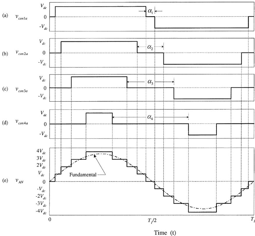
**Fig. 6.45** Key waveforms for the nine-level cascaded multilevel converter topology based on the single-phase full-bridge VSC circuit operation. (a) output voltage of converter 1,  $v_{con1a}$ ; (b) output voltage of converter 2,  $v_{con2a}$ ; (c) output voltage of converter 3,  $v_{con3a}$ ; (d) output voltage of converter 4,  $v_{con4a}$ ; and (e) converter phase voltage  $v_{AN}$ .
