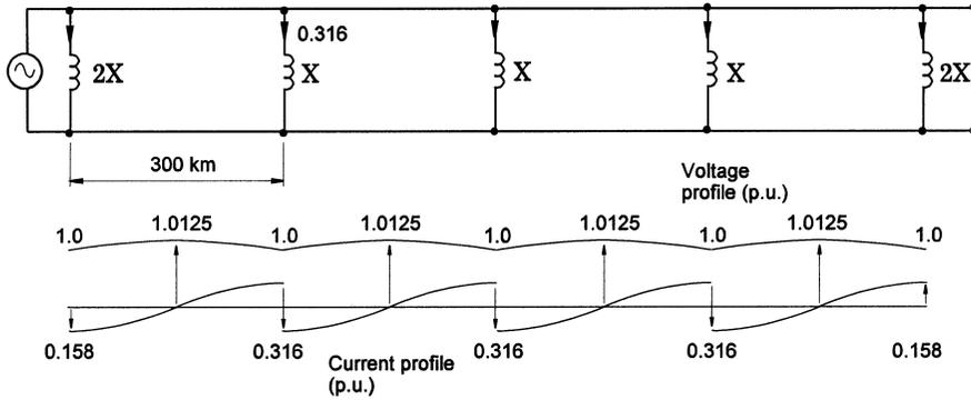
Fig. 3.13 Multiple shunt reactors along a long line.
