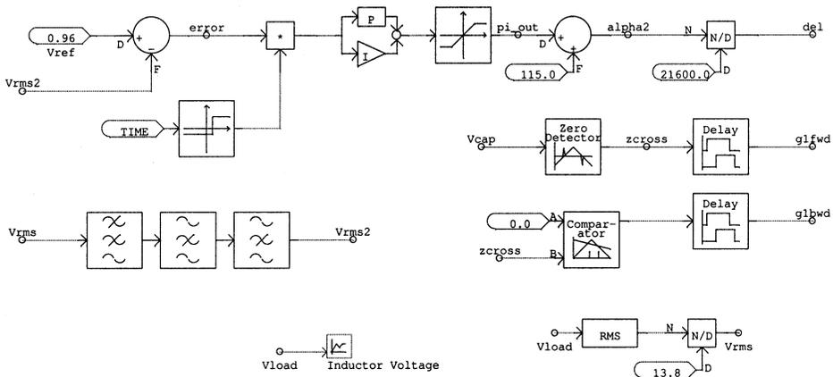
Fig. 8.18 SVC control scheme implemented in PSCAD/EMTDC.
