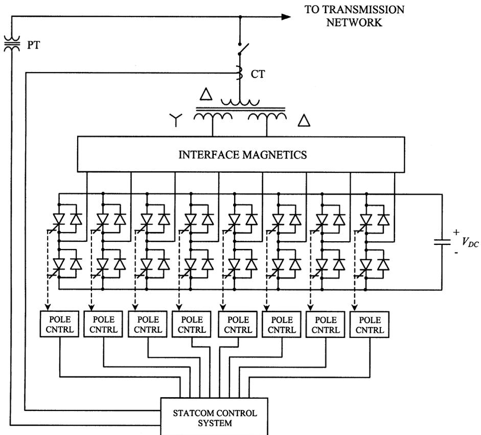
Fig. 8.41 Single-line diagram of a 48-pulse VSC-based STATCOM.
