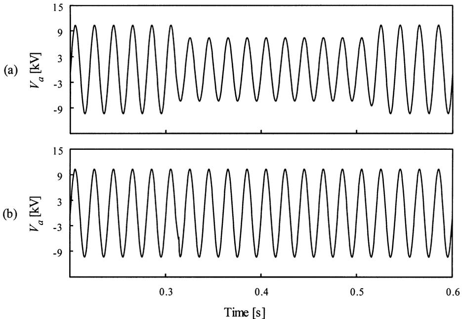
**Fig. 8.97** Phase voltage  $V_a$  at the load point. The fault is applied at  $t = 0.31$ s: (a) without SSTS; and (b) with SSTS operating.
