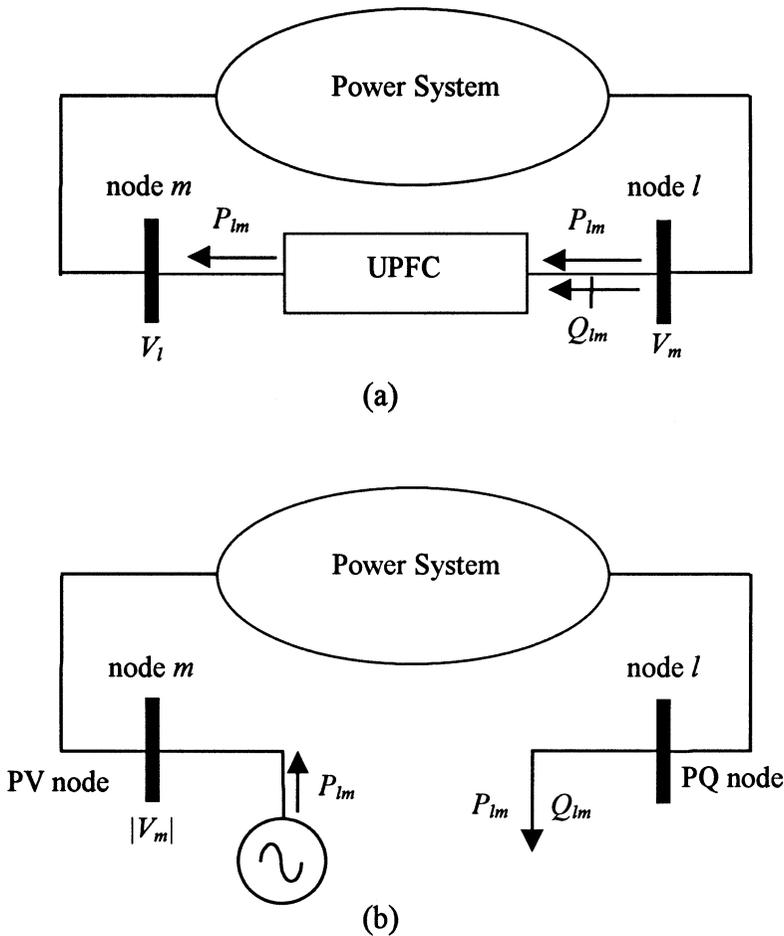
Fig. 4.22 UPFC model based on conventional power flow concepts.
