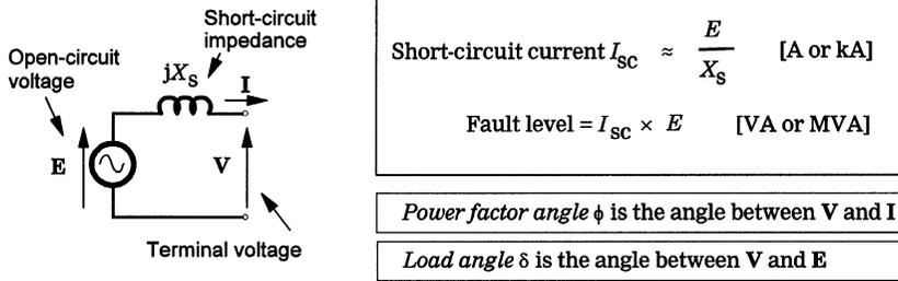
Fig. 2.1 Thévenin equivalent circuit of one phase of a supply system (neglecting resistance).
