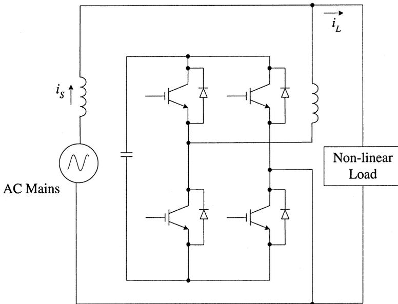
Fig. 6.91 VSC based single-phase shunt connected active filter.
