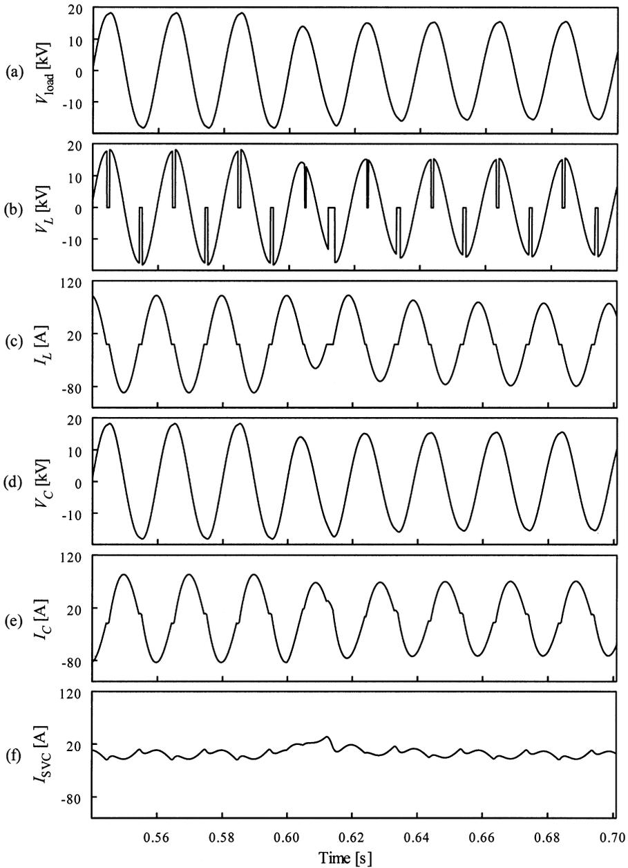
**Fig. 8.23** SVC characteristic waveforms in open-loop mode: (a) voltage  $V_{load}$  at the load point; (b) voltage  $V_L$  at the SVC inductor; (c) current  $I_L$  through the SVC inductor; (d) voltage  $V_C$  through the SVC capacitor; (e) current  $I_C$  through the SVC capacitor; and (f) total current  $I_{SVC}$  through the SVC.
