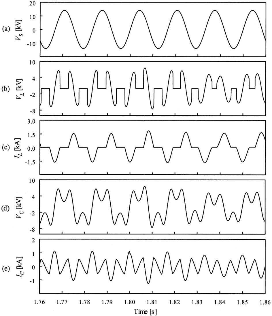
**Fig. 8.37** Waveforms in the TCSC operating with closed-loop control. Disturbance occurs at  $t = 1.8$  s: (a) voltage  $V_S$  of the source; (b) voltage  $V_L$  at the TCSC inductor; (c) current  $I_L$  through the TCSC inductor; (d) voltage  $V_C$  at the TCSC capacitor; and (e) current  $I_C$  through the TCSC capacitor.
