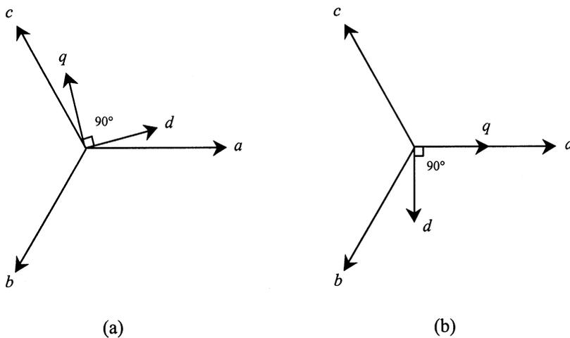
Fig. 8.63 (a) An arbitrary rotating frame; and (b) chosen rotating frame of reference.
