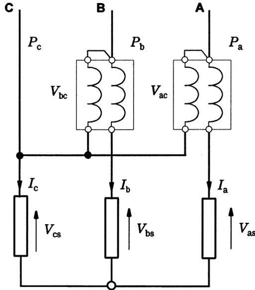
Fig. 2.35 Two-wattmeter connection.
