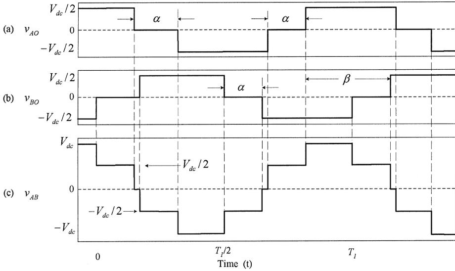
**Fig. 6.38** Key waveforms of the three-level single-phase full-bridge NPC VSC circuit operation. (a) line-to-DC bus mid-point voltage waveform  $v_{AO}$ ; (b) line-to-DC bus mid-point voltage waveform  $v_{BO}$ ; and (c) line-to-line voltage waveform  $v_{AB}$ .
