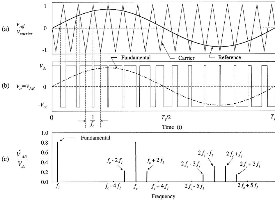
**Fig. 6.48** Two-level sinusoidal PWM with a single-phase full-bridge VSC. (a) reference (sinusoidal) and carrier (triangular) signals ( $f_c = 15 \cdot f_1$  and  $M_a = 0.8$ ); (b) voltage waveform  $v_{AB}$ ; and (c) normalized harmonic amplitude of the voltage waveform  $v_{AB}$ .
