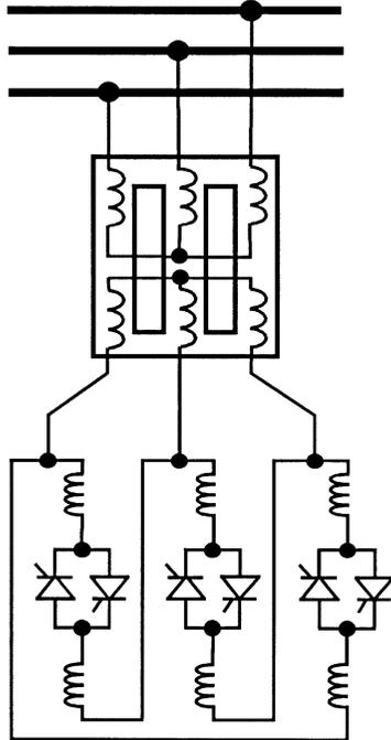
Fig. 1.9 Three-phase thyristor-controlled reactor connected in delta.
