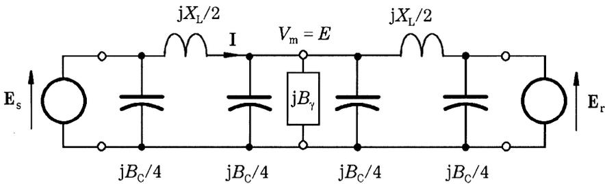
Fig. 9.8 Lumped-parameter representation of line with mid-point compensator.
