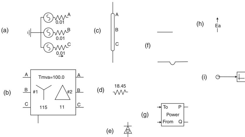
Fig. 8.6 Set of components required for the circuit of the example: (a) three-phase voltage source; (b) three-phase wye-delta transformer; (c) three-phase voltage signal sensor; (d) resistor; (e) diode; (f) wires; (g) active and reactive power meter; (h) voltage signal meter; and (i) signal plotting block.
