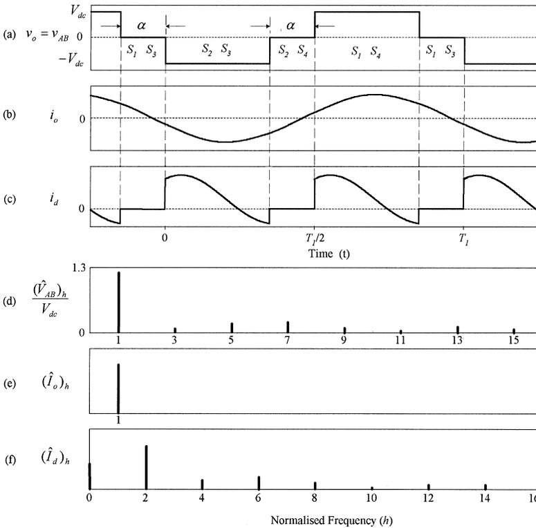
**Fig. 6.30** Key waveforms of the single-phase full-bridge phase-shifted controlled VSC circuit operation. (a) output voltage  $v_o = v_{AB}$ ; (b) output current  $i_o$ ; (c) DC bus current  $i_d$ ; (d) harmonic spectrum of the output voltage  $v_o = v_{AB}$ ; (e) harmonic spectrum of the output current  $i_o$ ; and (f) harmonic spectrum of the input DC bus current  $i_d$ .
