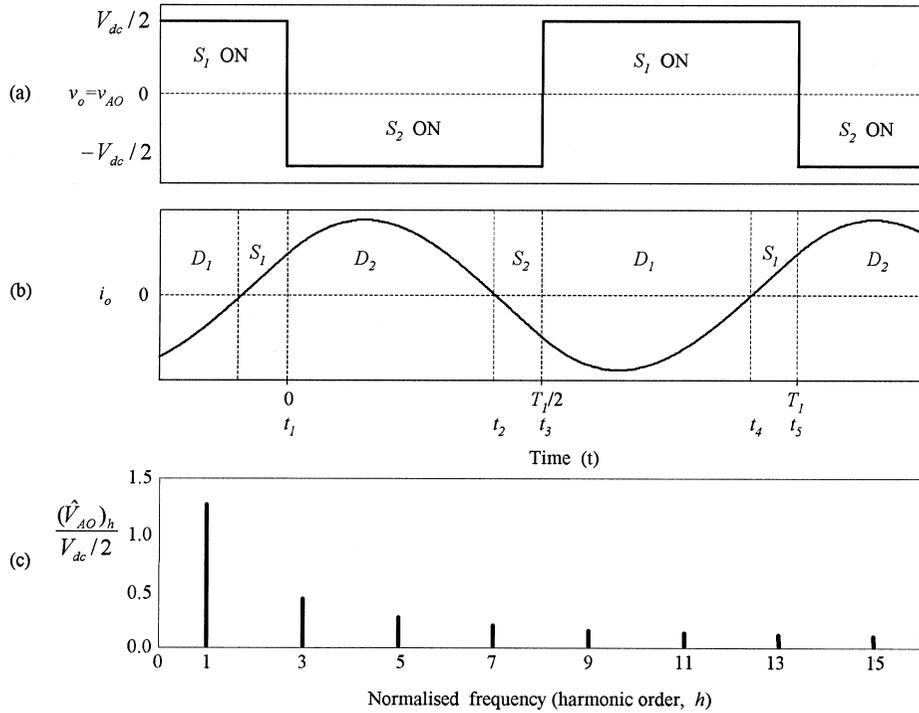
**Fig. 6.24** Key waveforms of the single-phase half-bridge VSC circuit operation. (a) output voltage  $v_o = v_{AO}$ ; (b) output current  $i_o$ ; and (c) harmonic spectrum of the output voltage  $v_o = v_{AO}$ .
