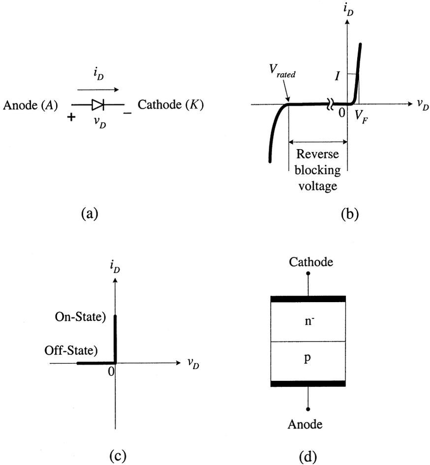
**Fig. 5.1** Diode: (a) circuit symbol; (b) typical  $i-v$  characteristics; (c) ideal  $i-v$  characteristics; and (d) typical structure.
