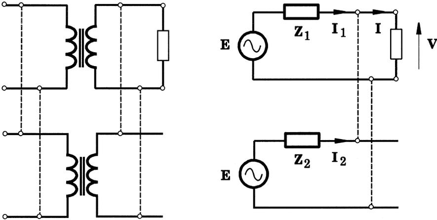
Fig. 2.43 Parallel transformers.
