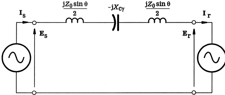
Fig. 3.22 Simplified equivalent circuit of series compensated line.
