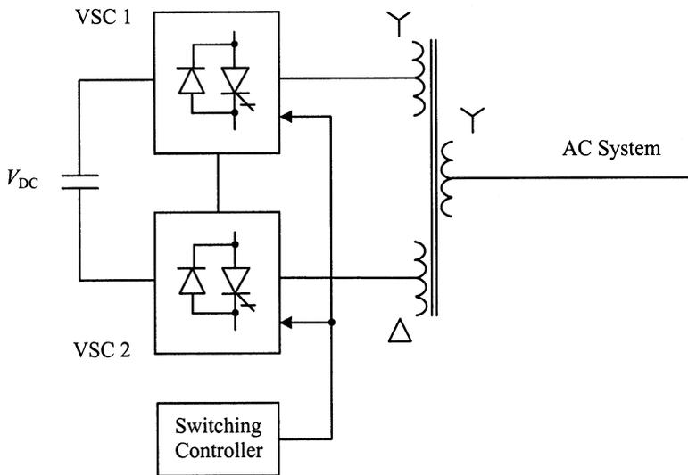
Fig. 8.44 Circuit used to implement a 12-pulse VSC-based STATCOM.
