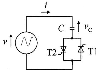
Fig. 6.16 Circuit for analysis of transient-free switching.
