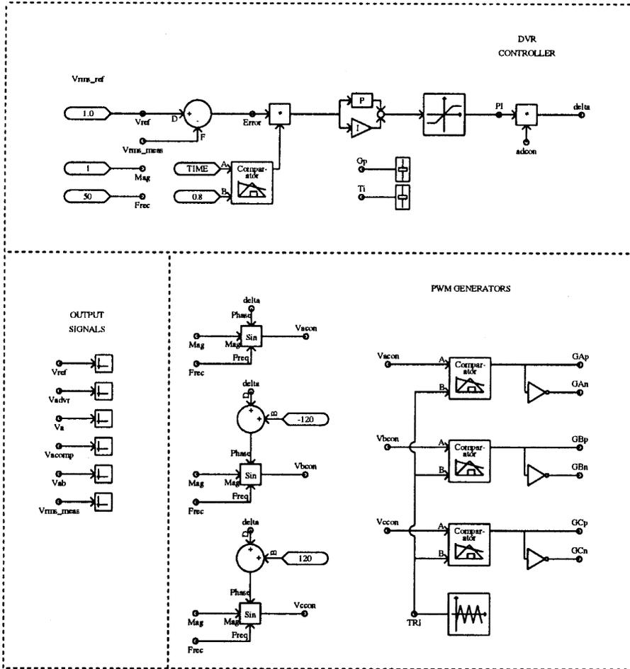
Fig. 8.58 DVR controller implemented in PSCAD/EMTDC.
