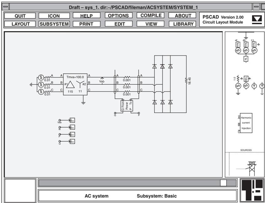
Fig. 8.8 Draft tool after completing the schematic drawing.
