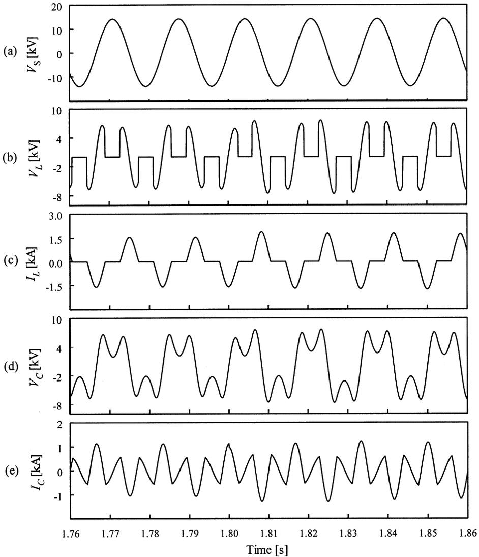
**Fig. 8.36** Waveforms in the TCSC operating with open-loop control. Disturbance occurs at  $t = 1.8$  s: (a) voltage  $V_S$  of the source; (b) voltage  $V_L$  at the TCSC inductor; (c) current  $I_L$  through the TCSC inductor; (d) voltage  $V_C$  at the TCSC capacitor; and (e) current  $I_C$  through the TCSC capacitor.
