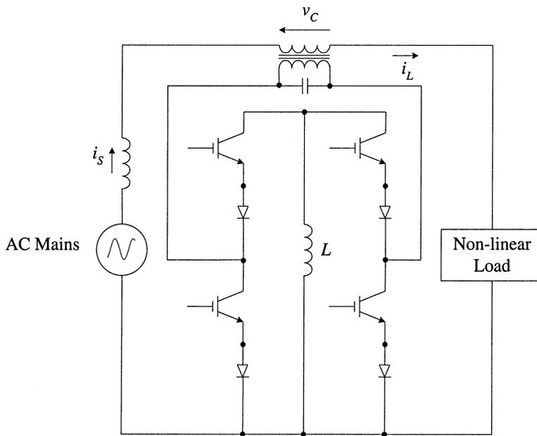
Fig. 6.87 CSC based single-phase series connected active filter.
