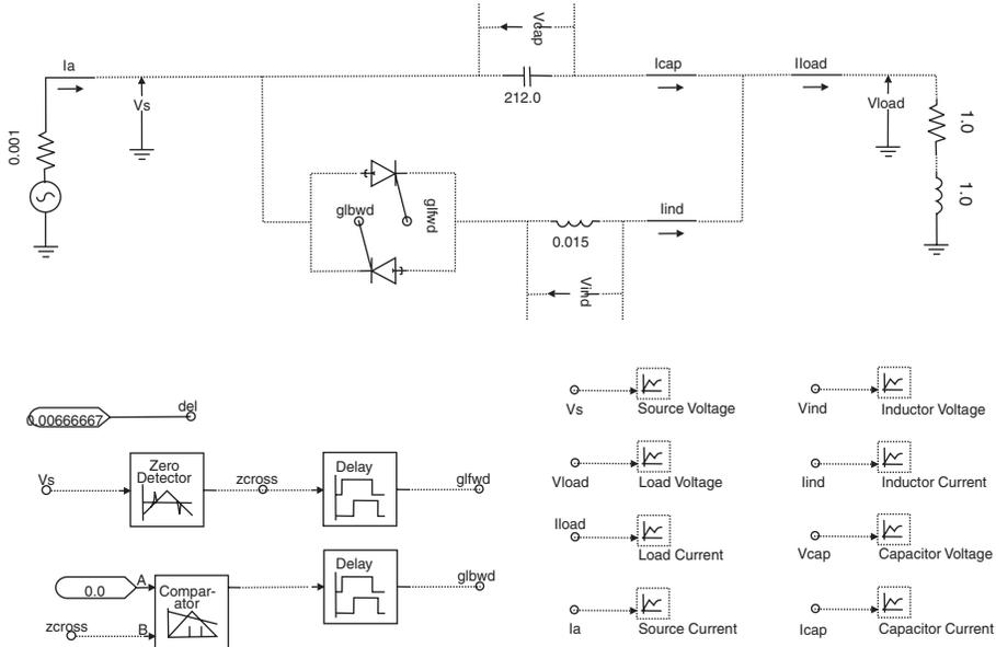
Fig. 8.27 TCSC basic circuit implemented in PSCAD/EMTDC.
