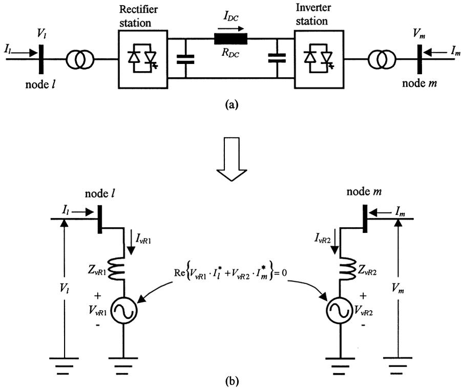
Fig. 4.7 HVDC Light. (a) the VSC at the sending end performs the role of rectifier and the VSC at the receiving end performs the role of inverter; and (b) equivalent circuit.
