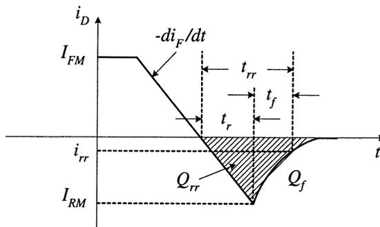
**Fig. 5.2** Diode reverse recovery parameters and definitions.
