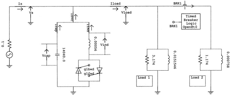
Fig. 8.17 SVC power circuit implemented in PSCAD/EMTDC.
