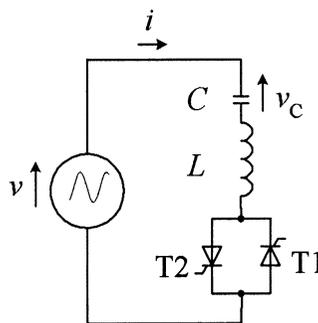
Fig. 6.17 Circuit for analysis of practical capacitor switching.
