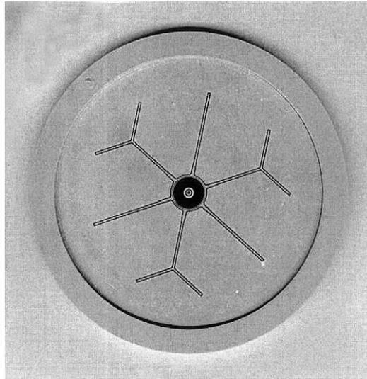
**Fig. 5.5** Photograph of a 5-inch light-triggered thyristor with integrated breakover diode. (Courtesy of Siemens and EUPEC.)
