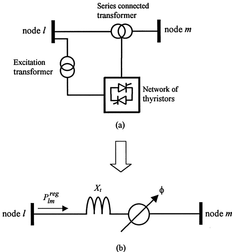
**Fig. 4.3** SPS. (a) structure formed by a series transformer, an excitation transformer and a network of thyristors; and (b) variable phase angle representation.
