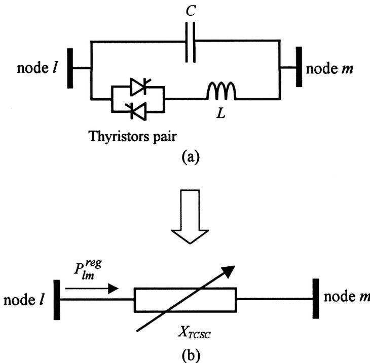
Fig. 4.2 TCSC. (a) structure formed by fixed capacitor and TCR; and (b) variable reactance representation.
