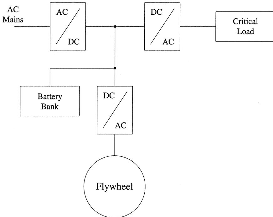
Fig. 6.64 Flywheel based UPS system with battery bank.
