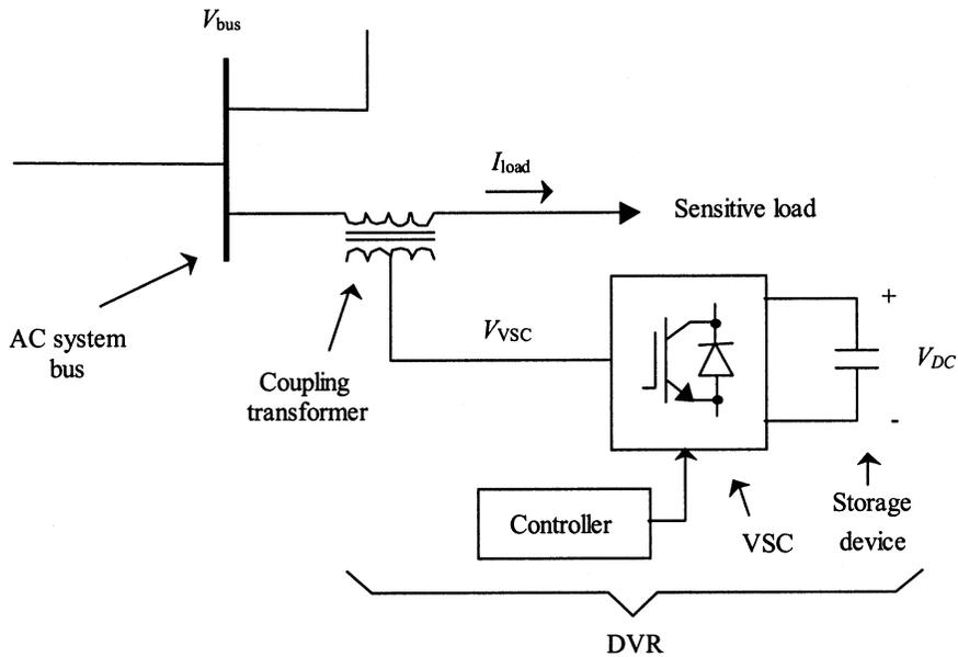
Fig. 8.55 Schematic representation of the DVR.
