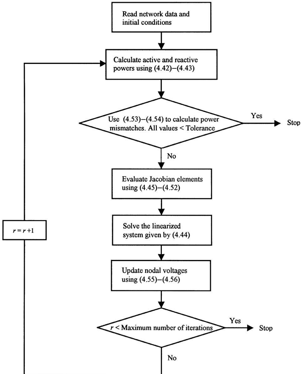
Fig. 4.15 Flow diagram for power flow Newton–Raphson method.
