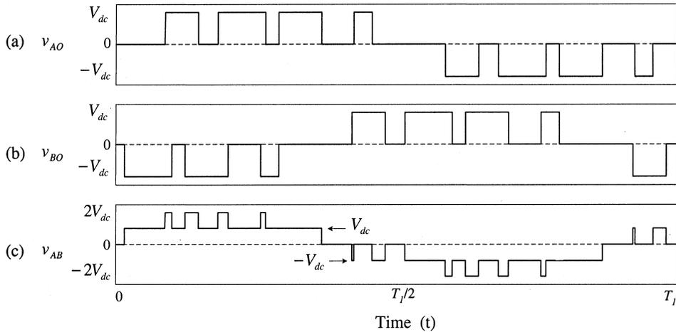
**Fig. 6.52** Sinusoidal PWM for the three-level single-phase full bridge NPC VSC. (a) line-to-neutral voltage waveform  $v_{AO}$ ; (b) line-to-neutral voltage waveform  $v_{BO}$ ; and (c) resultant line-to-line voltage waveform  $v_{AB}$ .
