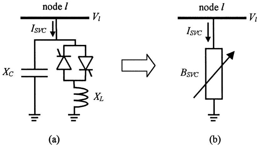
Fig. 4.1 SVC. (a) structure formed by fixed capacitor and TCR; and (b) variable susceptance representation.
