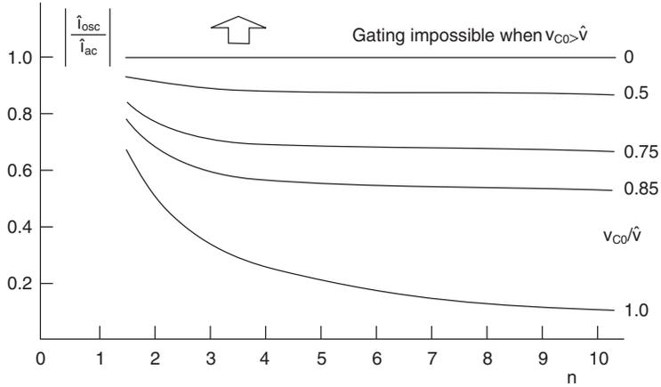
Fig. 6.19 Amplitude of oscillatory current component. Thyristors gated when  $v = v_{C0}$ .
