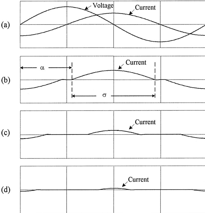
Fig. 6.2 Voltage and line current waveforms of a basic single-phase TCR for various firing angles. (a)  $\alpha = 90^\circ$ ,  $\sigma = 180^\circ$ ; (b)  $\alpha = 100^\circ$ ,  $\sigma = 160^\circ$ ; (c)  $\alpha = 130^\circ$ ,  $\sigma = 100^\circ$ ; (d)  $\alpha = 150^\circ$ ,  $\sigma = 60^\circ$ .
