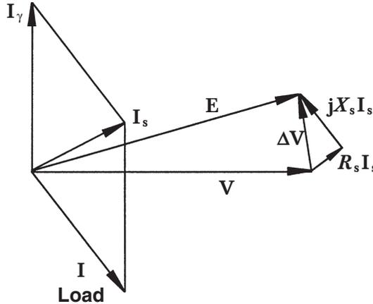
Fig. 2.15 Phasor diagram, compensated for constant voltage.
