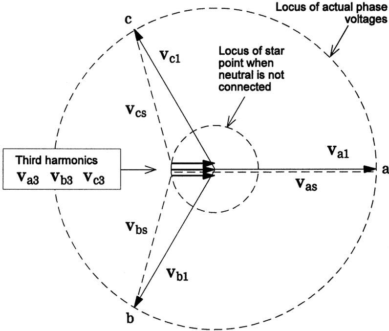
Fig. 2.48 Third-harmonic oscillation of the star-point potential.
