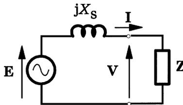
**Fig. 2.7** AC supply and load circuit.
