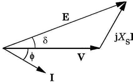
Fig. 2.9 Phasor diagram, inductive load.
