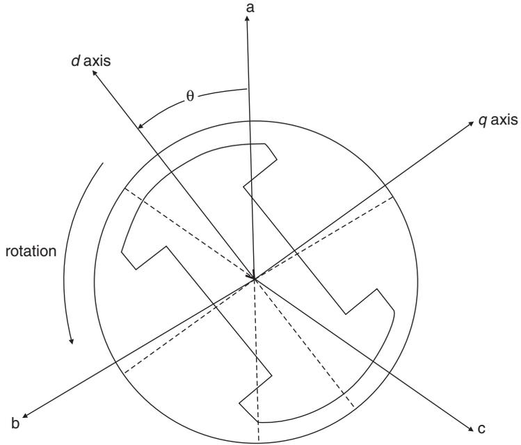
Fig. 1.2 Schematic diagram of a synchronous machine.
