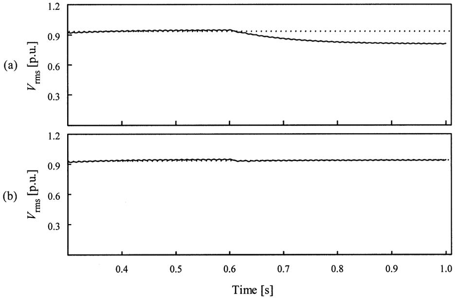
**Fig. 8.19** Voltage  $V_{rms}$  at the load point: (a) with SVC operating in open-loop mode; and (b) with SVC operating in closed-loop mode.
