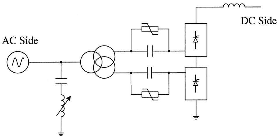
**Fig. 6.78** Single-line diagram of a monopolar HVDC power transmission system with capacitor commutated converter (CCC).
