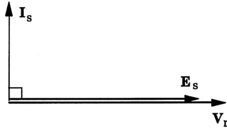
Fig. 3.4 Phasor diagram of uncompensated line on open-circuit.
