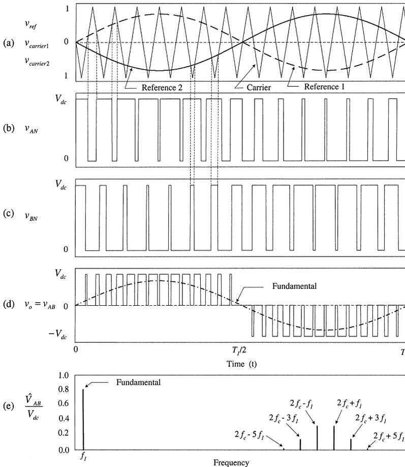
**Fig. 6.49** Three-level sinusoidal PWM method for single-phase full-bridge VSC. (a) two reference signals (sinusoidal) and carrier (triangular) signal ( $f_c = 15 \cdot f_1$  and  $M_a = 0.8$ ); (b) voltage waveform  $v_{AN}$ ; (c) line-to-line voltage waveform  $v_{AB}$ ; and (d) normalized harmonic amplitude of the voltage waveform  $v_{AB}$ .
