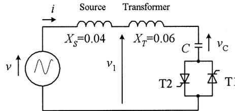
Fig. 6.21 Switching a discharge capacitor; circuit diagram.
