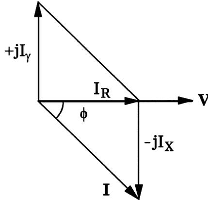
Fig. 2.11 Phasor diagram for power factor correction.
