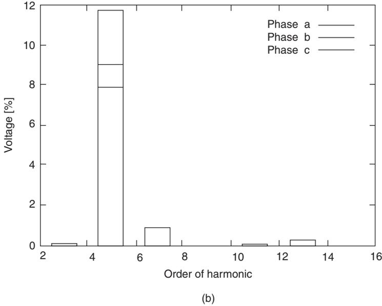
Fig. 7.9 Voltage waveform and harmonic content at the TCR.
