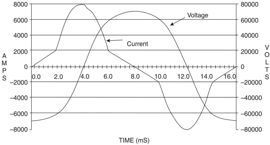
Fig. 7.11 Voltage and current waveforms in the TCSC capacitor.
