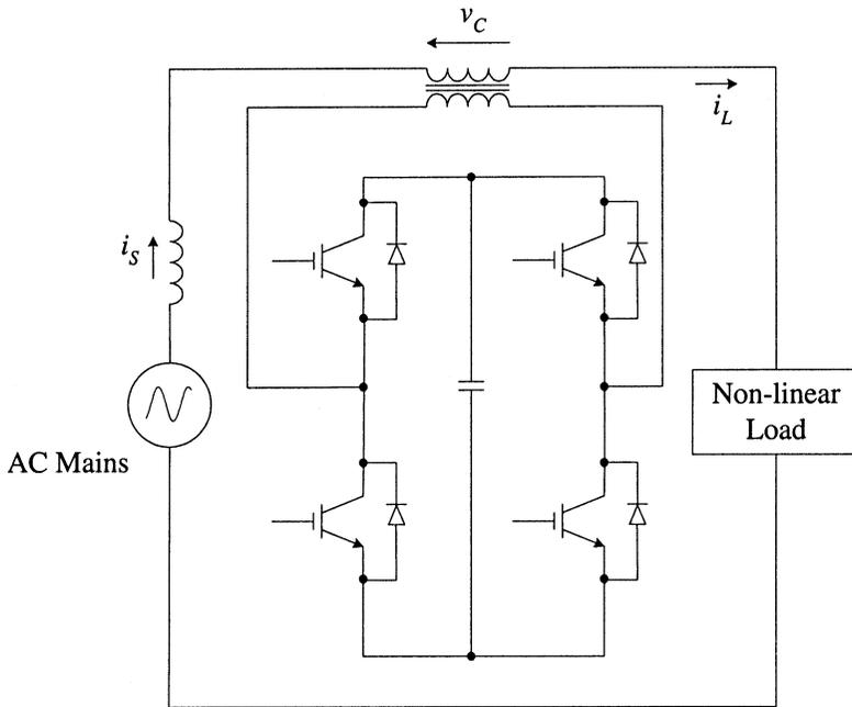
Fig. 6.90 VSC based single-phase series connected active filter.
