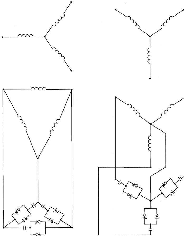
**Fig. 6.12** Alternative arrangements of three-phase thyristor-switched capacitor. (a) delta-connected secondary, Delta-connected TSC; and (b) wye-connected secondary, wye-connected TSC (four-wire system).
