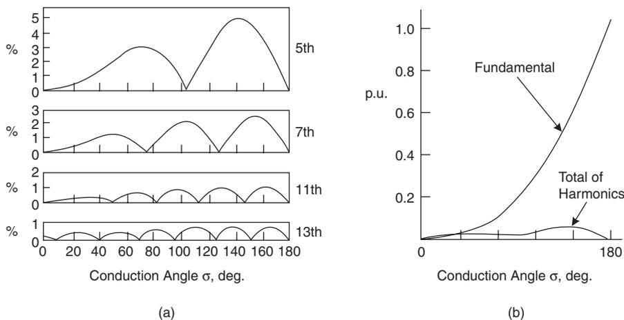
**Fig. 6.5** TCR Harmonics. (a) major harmonic current components of TCR. Each is shown as a percentage of the fundamental component at full conduction. The percentages are the same for both phase and line currents; and (b) total harmonic content of TCR current, as a fraction of the fundamental component at full conduction. The percentages are the same for both phase and line currents.
