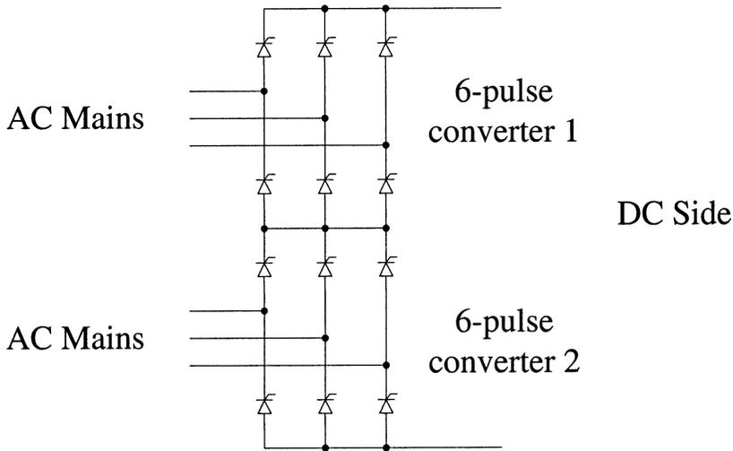
**Fig. 6.68** Circuit configuration of a 12-pulse thyristor converter.
