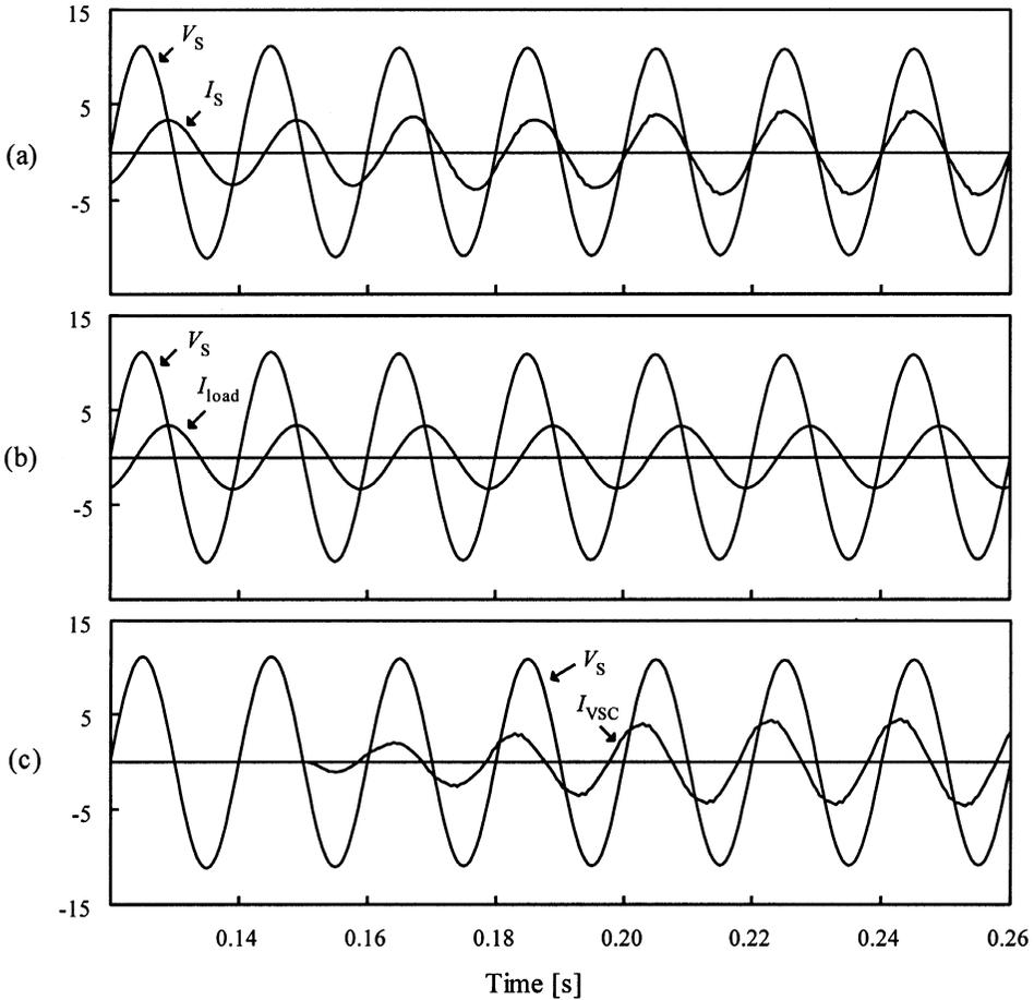
**Fig. 8.68** Key waveforms for the PFC circuit: (a) source voltage  $V_s$  and current  $I_s$ ; (b) source voltage  $V_s$  and load current  $I_{load}$ ; and (c) source voltage  $V_s$  and converter current  $I_{vsc}$ .
