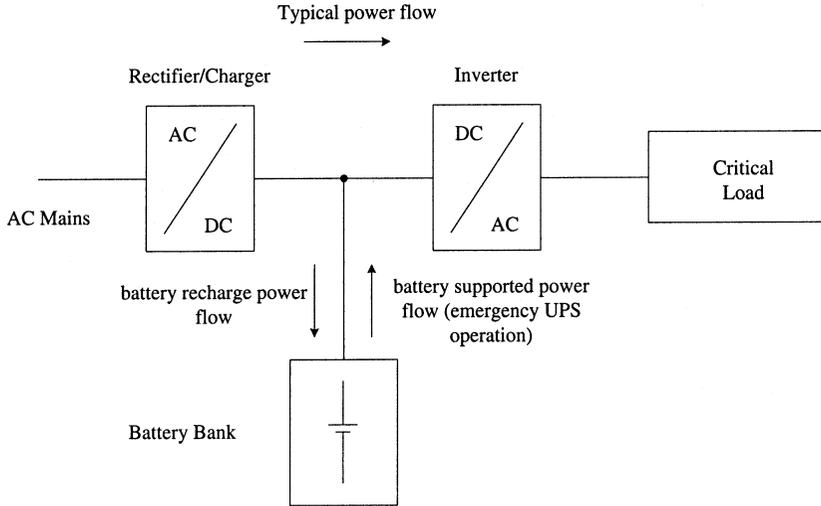
Fig. 6.53 Block diagram of a basic UPS system.
