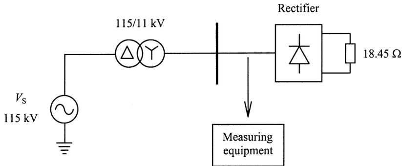
Fig. 8.1 Test circuit to be built in PSCAD.
