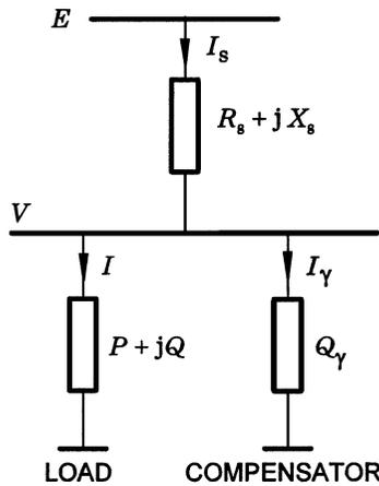
Fig. 2.12 Equivalent circuit of supply and load.
