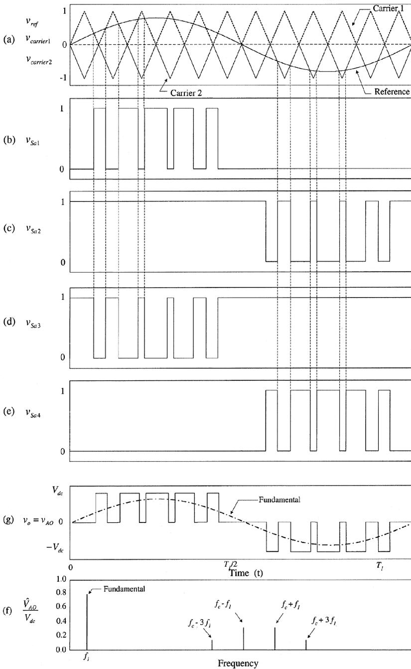
**Fig. 6.51** Sinusoidal PWM for the three-level single-phase half-bridge NPC VSC. (a) reference and two carrier waveforms phase-shifted by  $180^\circ$ ; (b) control signal for switch  $S_{a1}$ ; (c) control signal for switch  $S_{a2}$ ; (d) control signal for switch  $S_{a3}$ ; (e) control signal for switch  $S_{a4}$ ; (g) resultant line-to-neutral voltage waveform  $v_{AO}$ ; and (f) harmonic spectrum of the line-to-neutral voltage waveform  $v_{AO}$ .
