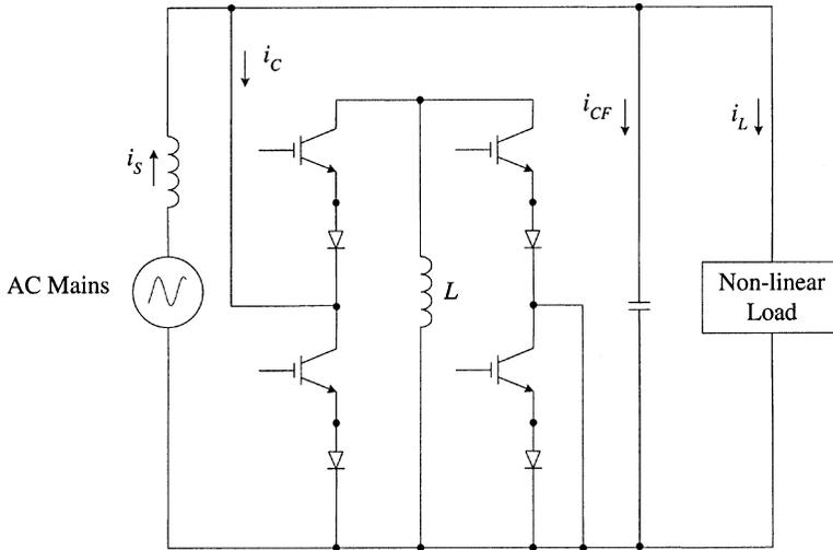
Fig. 6.88 CSC based single-phase shunt connected active filter.
