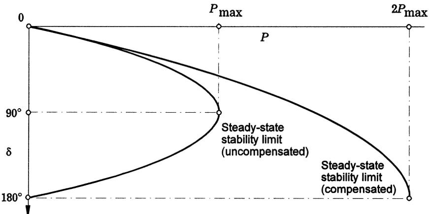
Fig. 3.16 Power transmission characteristic with dynamic shunt compensation.
