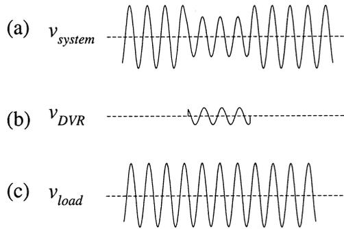
**Fig. 6.57** Key waveforms of the DVR operation.
