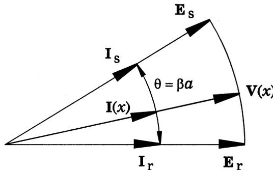
Fig. 3.2 Phasor diagram of line terminated in  $Z_0$ .
