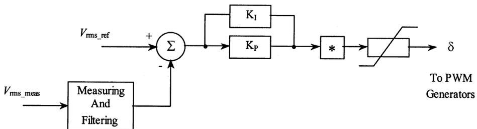
Fig. 8.49 Control scheme designed for the D-STATCOM.
