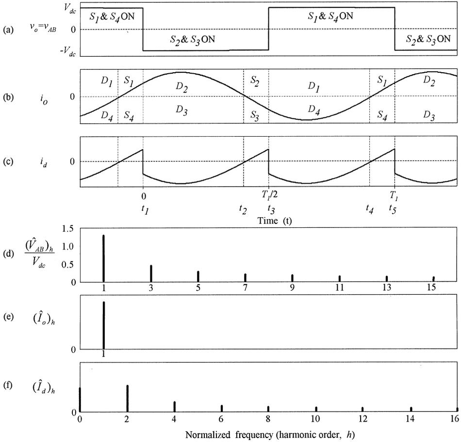
**Fig. 6.27** Key waveforms of the single-phase full-bridge VSC circuit operation. (a) output voltage  $v_o = v_{AB}$ ; (b) output current  $i_o$ ; (c) input DC bus current  $i_d$ ; (d) harmonic spectrum of the output voltage  $v_o = v_{AB}$ ; (e) harmonic spectrum of the output current  $i_o$ ; and (f) harmonic spectrum of the input DC bus current  $i_d$ .
