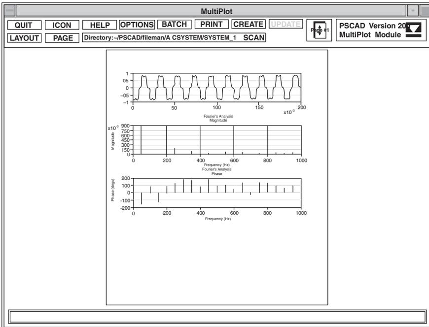
Fig. 8.10 Multiplot module used for further analysis of output waveforms.
