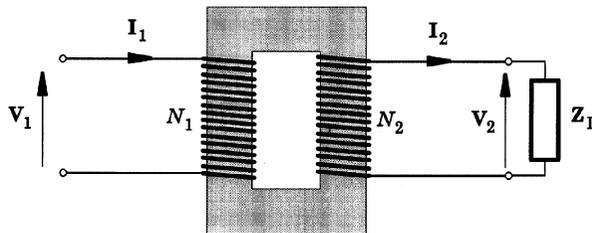
Fig. 2.37 Basic transformer.
