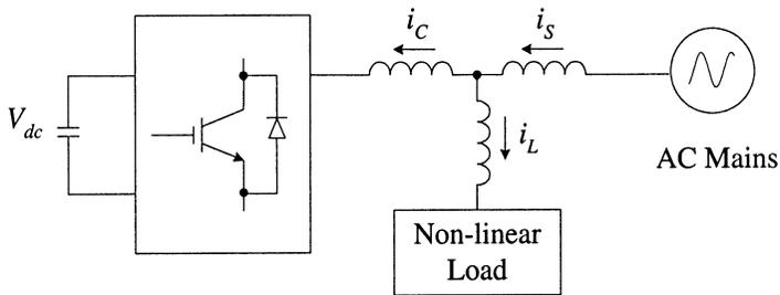
Fig. 6.83 VSC based shunt connected active filter.
