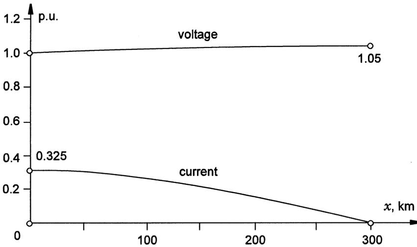
Fig. 3.5 Voltage and current profiles for a 300-km line at no load (open-circuit).
