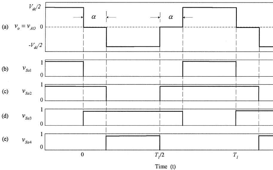
**Fig. 6.35** Key waveforms of the three-level single-phase half-bridge NPC VSC circuit operation. (a) output voltage  $v_o = v_{AO}$ ; (b) control signal for the switch  $S_{a1}$ ; (c) control signal for the switch  $S_{a2}$ ; (d) control signal for switch  $S_{a3}$ ; and (e) control signal for switch  $S_{a4}$ .
