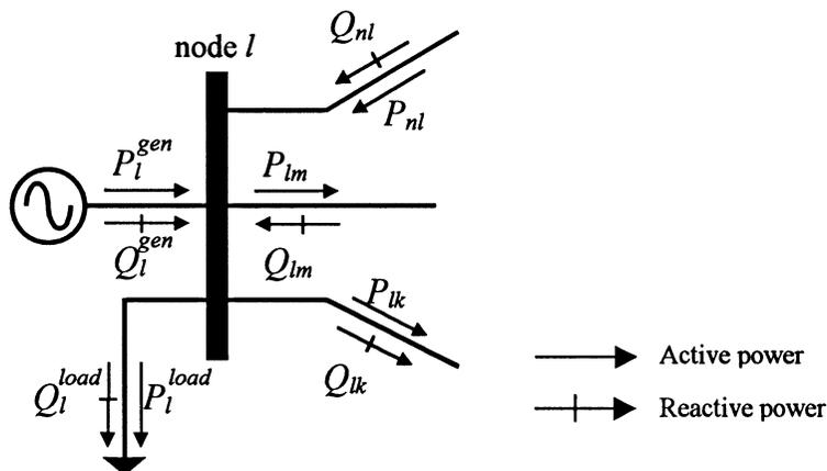
Fig. 4.10 Generic node of the electrical power network.
