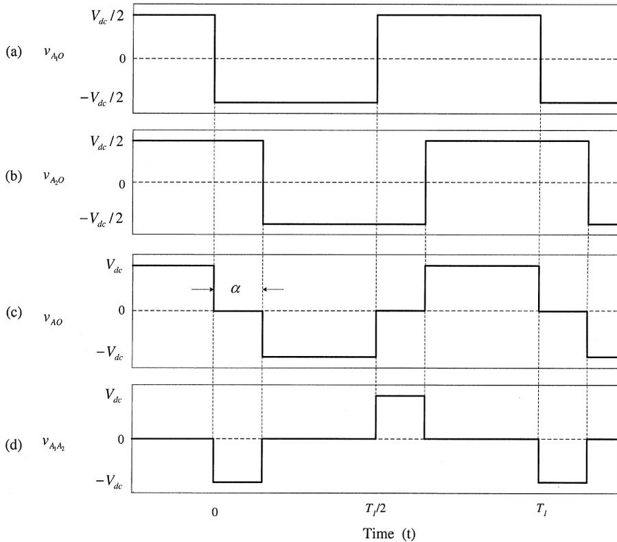
**Fig. 6.41** Key waveforms of the three-level converter with parallel legs and a summing inductor circuit operation. (a) voltage waveform between the mid-point of the left phase leg  $A_1$  and the DC bus mid-point  $O$ ,  $v_{A1O}$ ; (b) voltage waveform between the mid-point of the right phase leg  $A_2$  and the DC bus mid-point  $O$ ,  $v_{A2O}$ ; (c) voltage waveform between the phase point and the DC bus mid-point,  $v_{AO}$ ; and (d) voltage waveform across the inductor  $v_{A1A2}$ .
