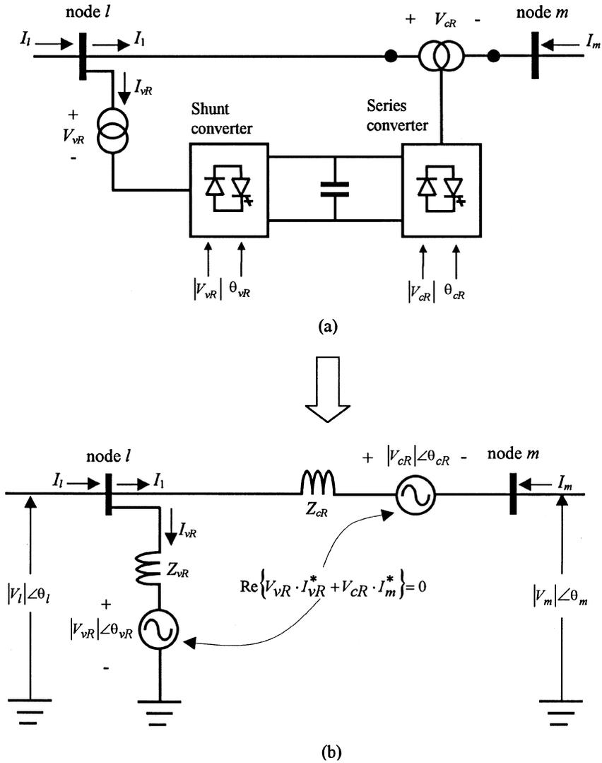
**Fig. 4.6** UPFC. (a) back-to-back VSCs with one VSC connected to the AC network via a shunt transformer and a second VSC connected to the AC network via a series transformer; and (b) equivalent circuit based on solid-state voltage sources.
