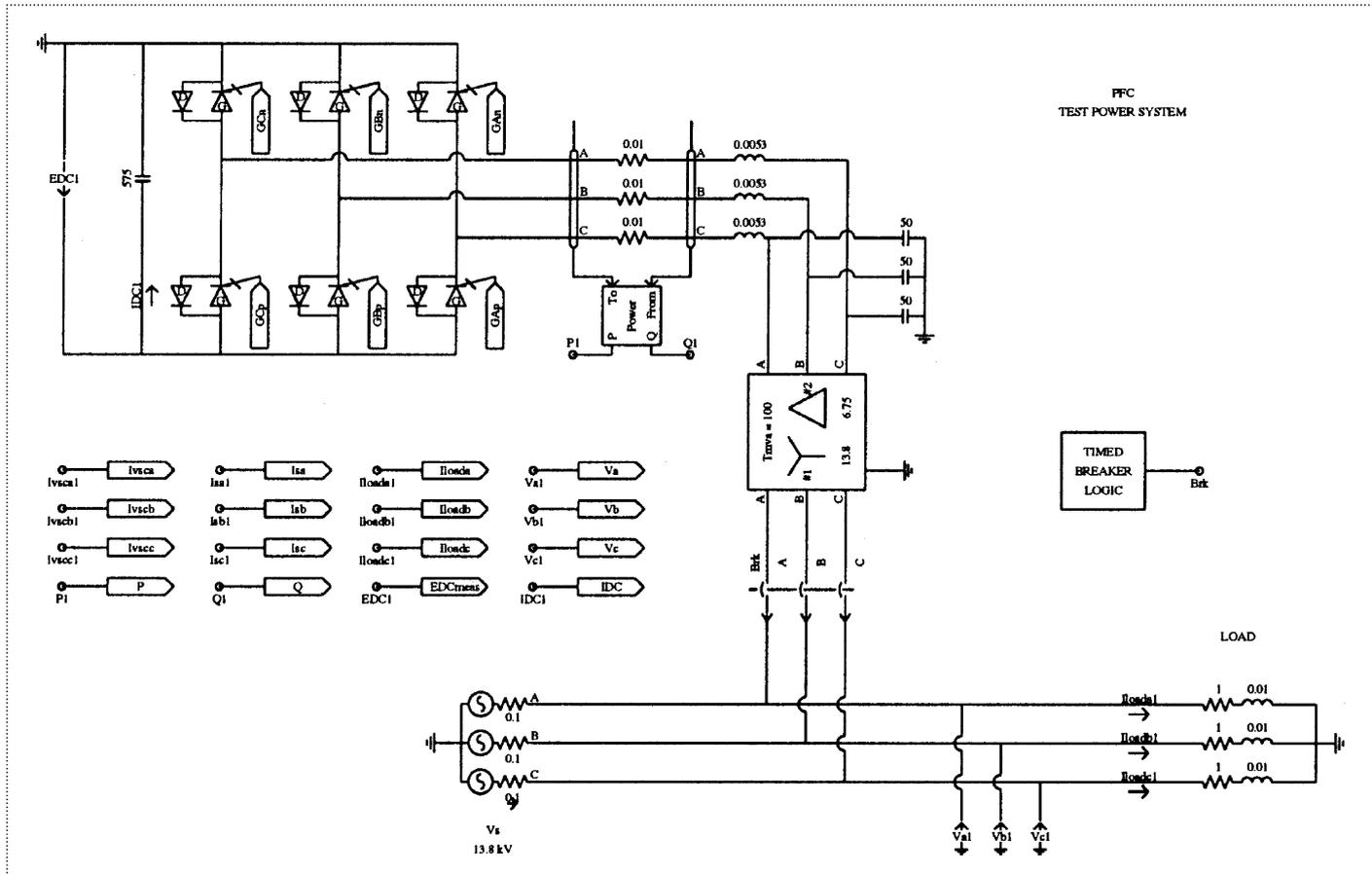
Fig. 8.65 PFC test system implemented in PSCAD/EMTDC.
