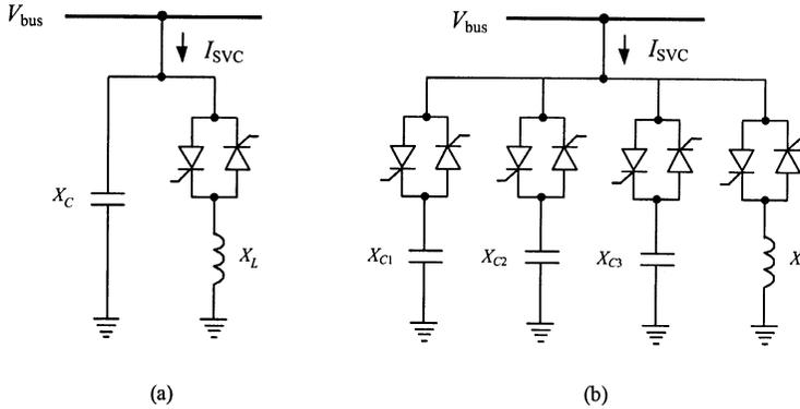
Fig. 8.12 Typical SVC's structures: (a) a TCR with a fixed capacitor; and (b) a TCR with a TSC.
