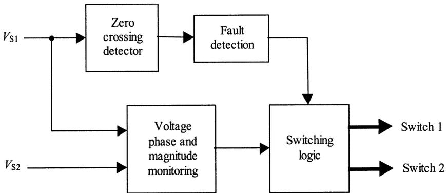
Fig. 8.93 Control circuit designed for the SSTS.
