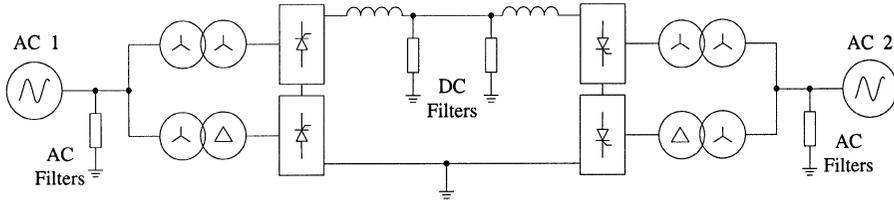
Fig. 6.71 Back-to-back HVDC power system with 12-pulse converters.
