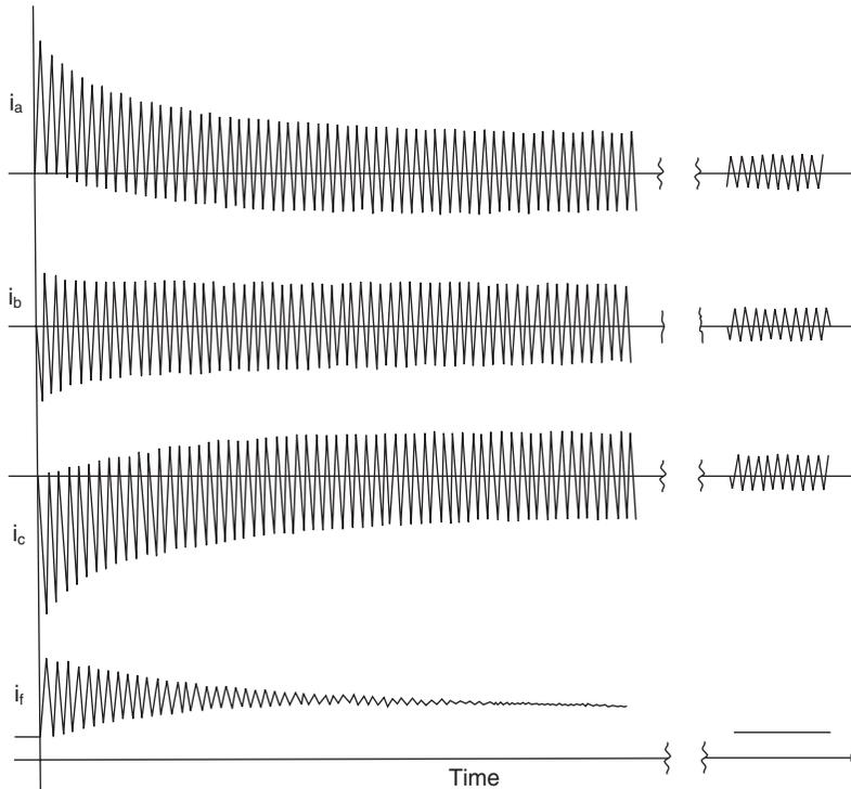
**Fig. 1.19** Short-circuit currents of a synchronous generator (© 1995 IEEE).
