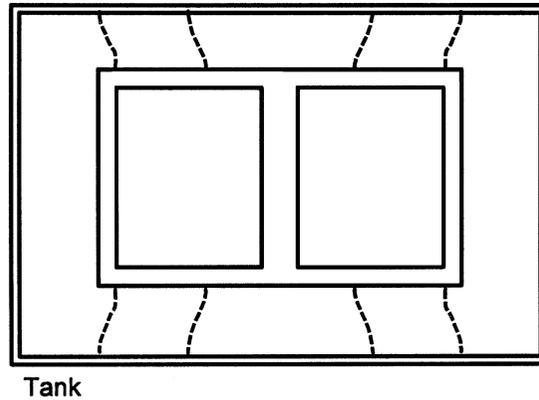
Fig. 2.45 Residual fluxes in 3-limb core and tank.
