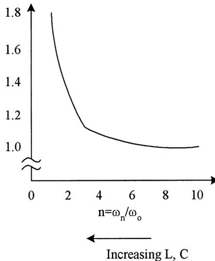
Fig. 6.18 Voltage and current magnification factor  $n^2 / (n^2 - 1)$ .
