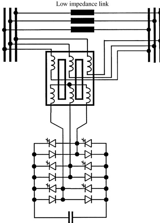
Fig. 1.14 Three-phase dynamic voltage restorer.
