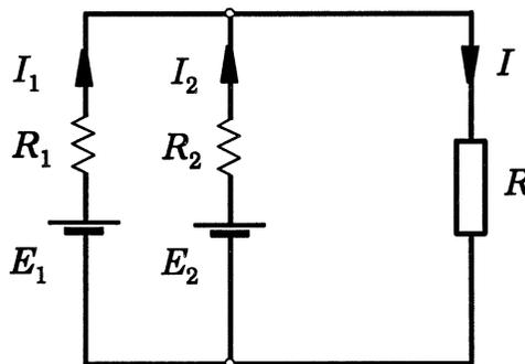
Fig. 2.42 Parallel batteries supplying a DC load.
