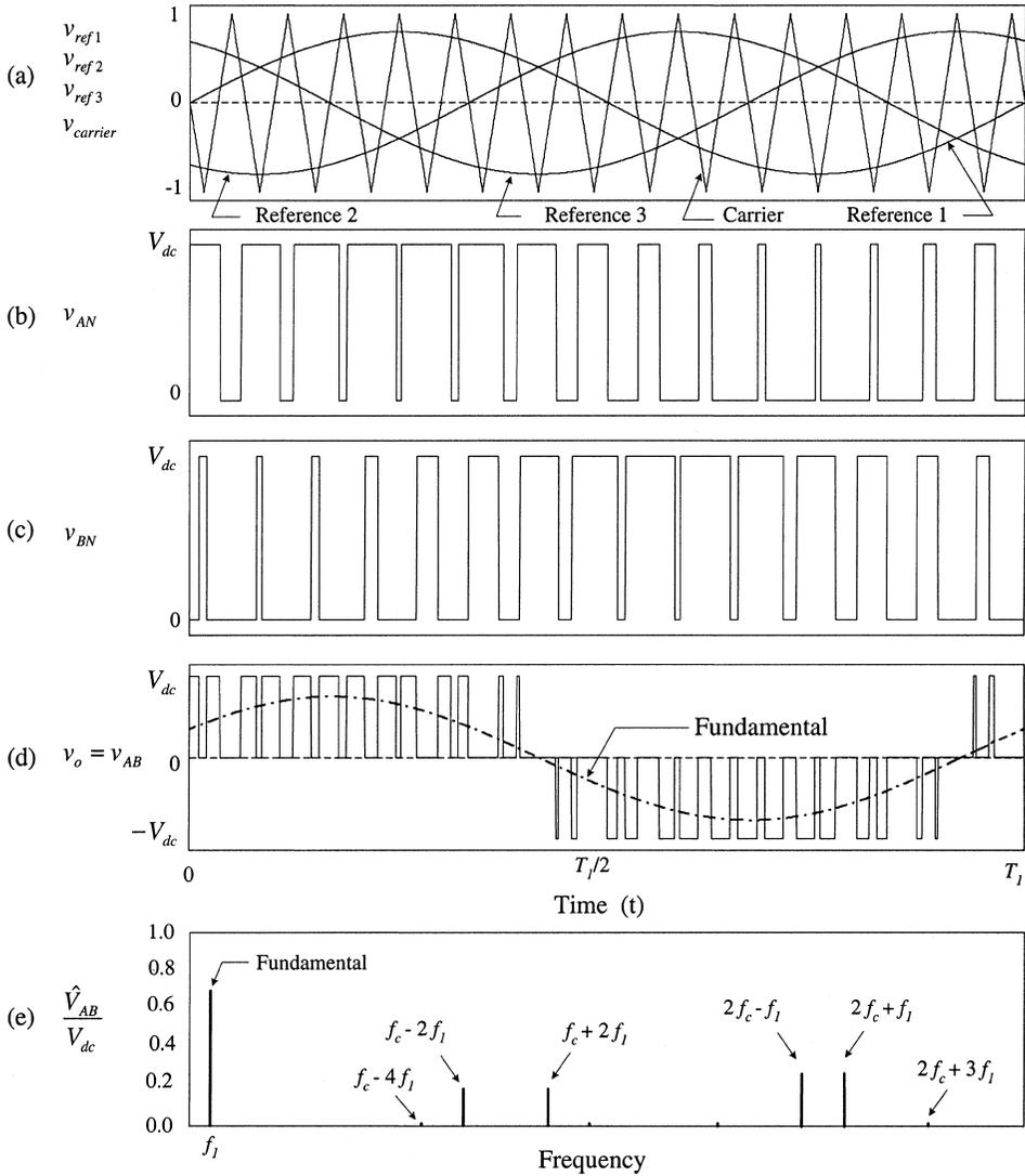
**Fig. 6.50** Two-level sinusoidal PWM method for the conventional six-switch three-phase VSC. (a) reference signals and carrier signal (triangular) ( $f_c = 15 \cdot f_1$  and  $M_a = 0.8$ ); (b) voltage waveform  $v_{AN}$ ; (c) voltage waveform  $v_{BN}$ ; (d) line-to-line output voltage waveform  $v_{AB}$ ; and (e) normalized harmonic amplitude of the voltage waveform  $v_{AB}$ .
