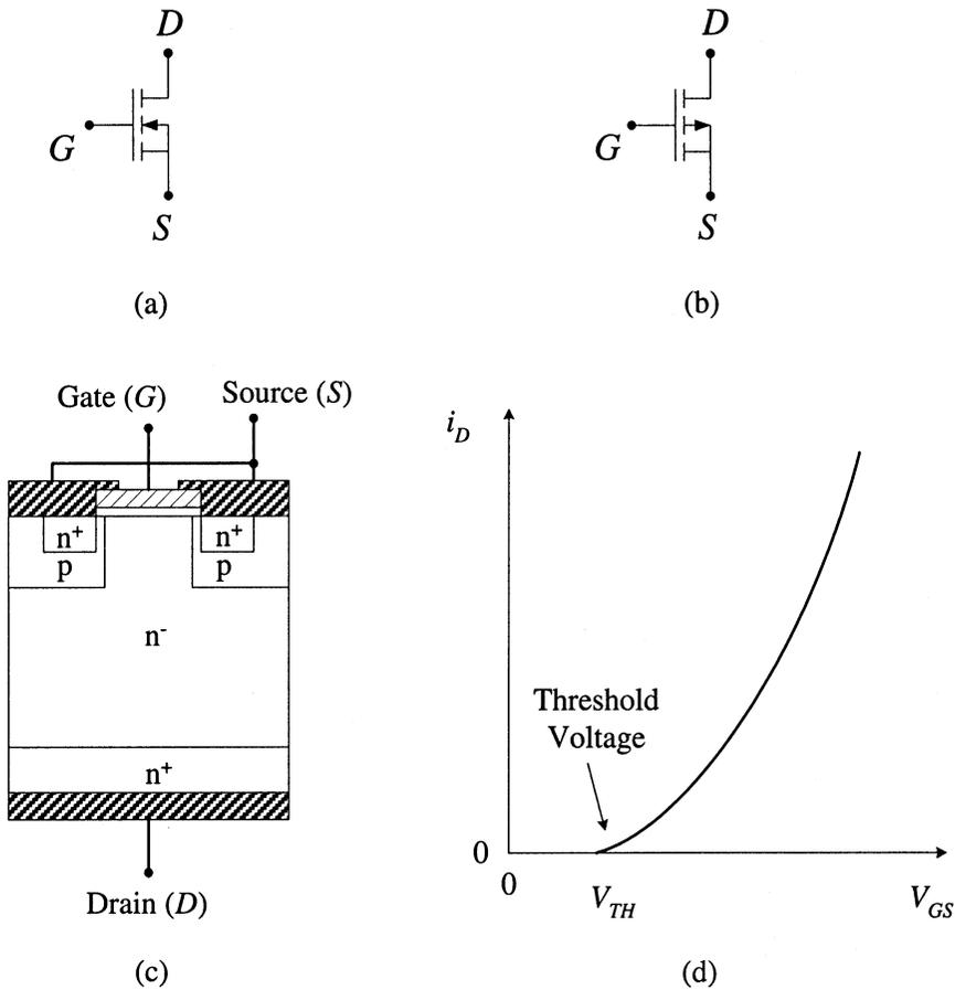
**Fig. 5.8** Power MOSFET: (a) circuit symbol for an  $n$ -channel; (b) circuit symbol for a  $p$ -channel; (c) basic structure of an  $n$ -channel device; and (d) voltage signal control of a typical  $n$ -channel device.
