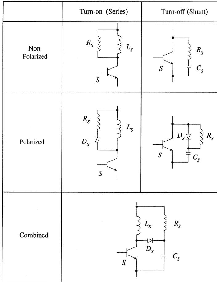
Fig. 5.14 Conventional dissipative snubber circuits.
