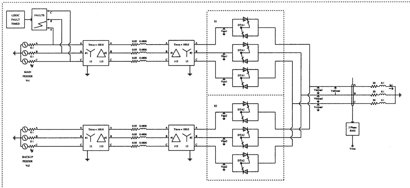
Fig. 8.94 SSTS test system implemented in PSCAD/EMTDC.
