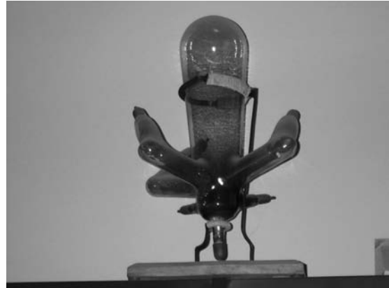
FIGURE 2.49 Three-phase mercury arc rectifier.
