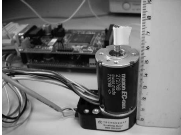
FIGURE 7.37 Photograph of the fractional power PMSM drive.
