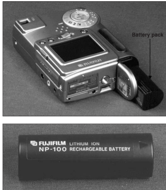
Figure 5.9 Digital camera with lithium-ion battery pack.
