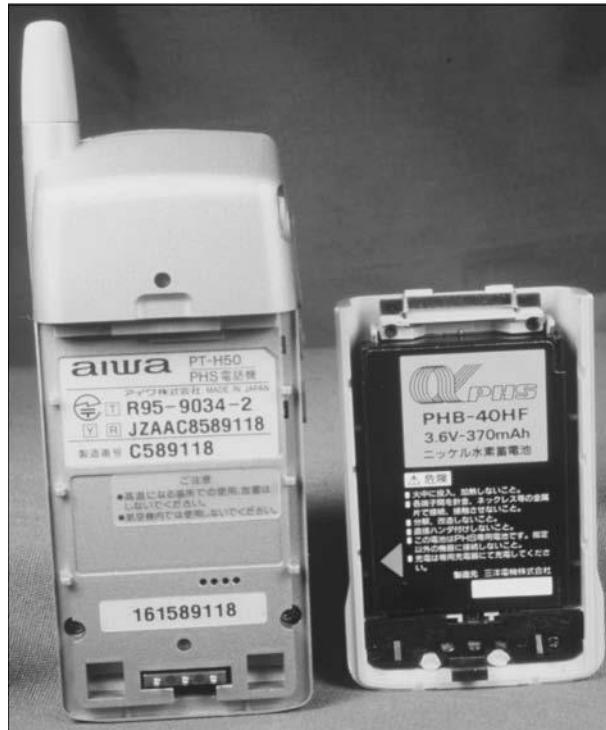
Figure 5.7 Ni-MH battery with attached plastic housing.
