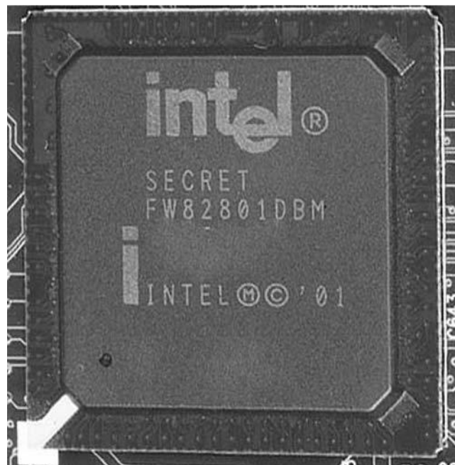
Figure 3.13 BGA package on notebook computer motherboard.
