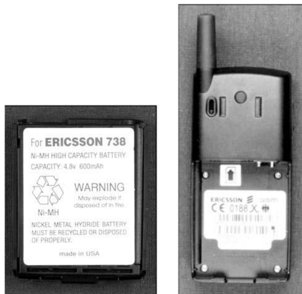
Figure 5.8 Compact Ni-MH battery pack for a cell phone.
