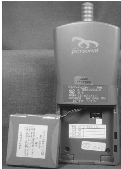
Figure 5.3 Cell phone battery with wired connection.
