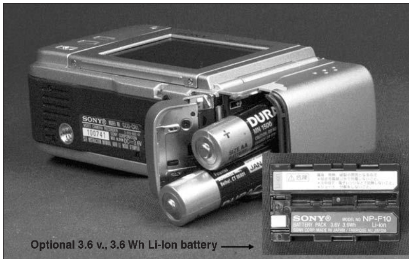
Figure 5.11 Digital camera using AA cells or lithium-ion cell.
