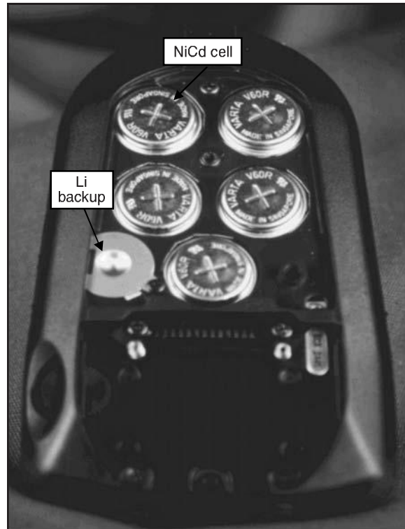
Figure 5.14 Voice recorder with button cell batteries.
