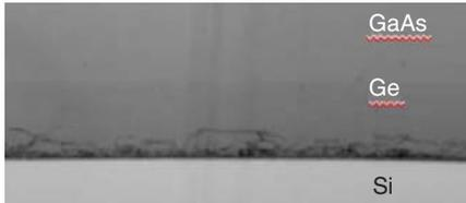
Figure 10.10 Cross-sectional TEM image of GaAs on Ge on off-cut SOI.
