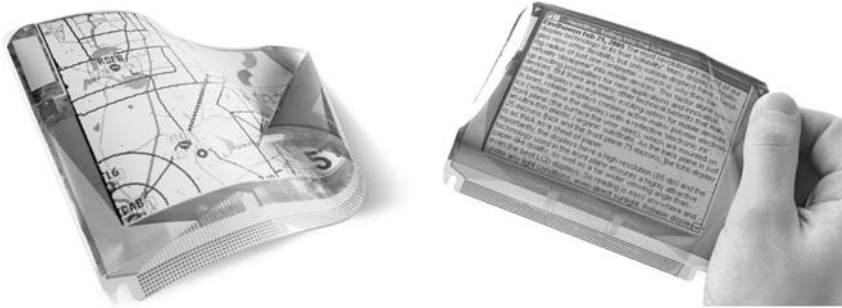
Fig. 14.12. Two pictures of the rollable QVGA active-matrix electronic ink display. Images with four gray levels are displayed.
