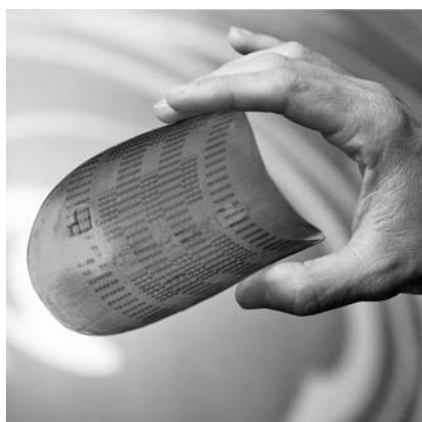
Fig. 13.6. Fully processed 150-mm wafer foil containing all-polymer transistors and integrated circuits.
