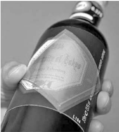
Fig. 16.10. Because the new scanner is mechanically flexible, it can be bent to cover curved surfaces such as labels of wine bottles.
