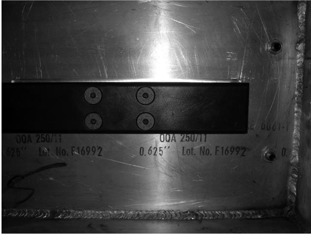
*Figure 7.7 View of the upper half-shell from below showing the center plate attachment as well as two of the four bolts that hold the ground planes to the movement mechanism. Note the black plasma coating on the center plate. The center plate is held onto the Delrin block with four long bolts*
