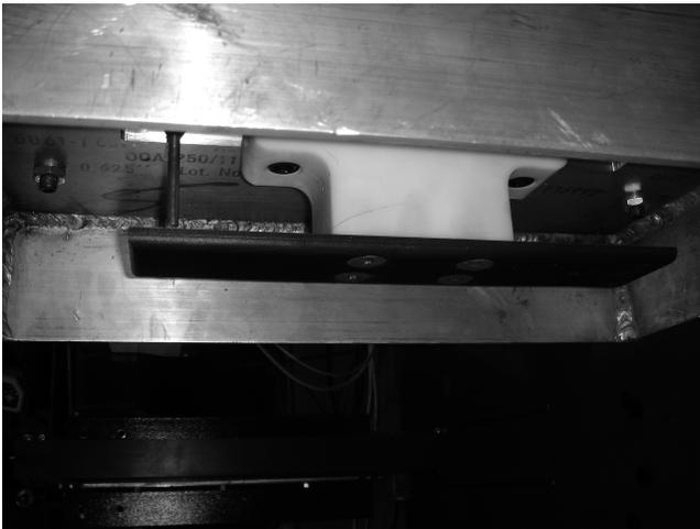
*Figure 7.6 Upper half of the sensor. The central plate is held in place on a Delrin block with four recessed screws to allow for a smooth surface. The Delrin block is solid and held in place in its channel with two bolts*
