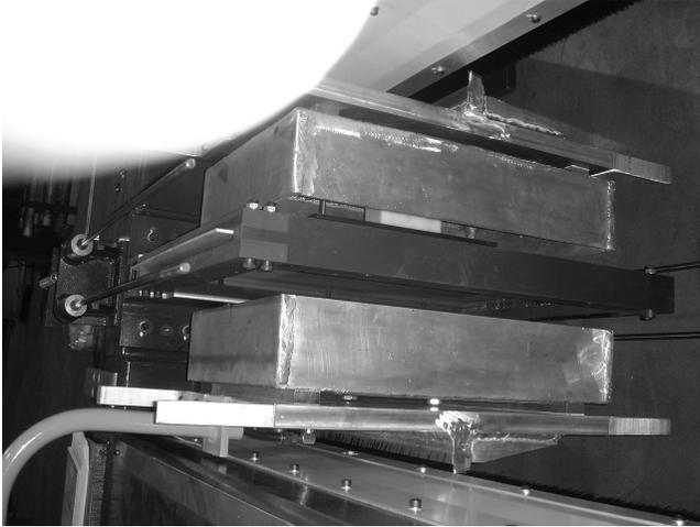
*Figure 7.5 The two halves of the sensor placed over one of the calibration frames. The two calibration frames are located on the two extremes of the sensor's travel (see Section 7.4). Note how the two halves are attached to the motion mechanism at the top and bottom. The driving mechanism cannot be seen—it is hidden behind the guiding strips. One of the probes and the upper center plate with its Delrin support can also be seen above the calibration frame*
