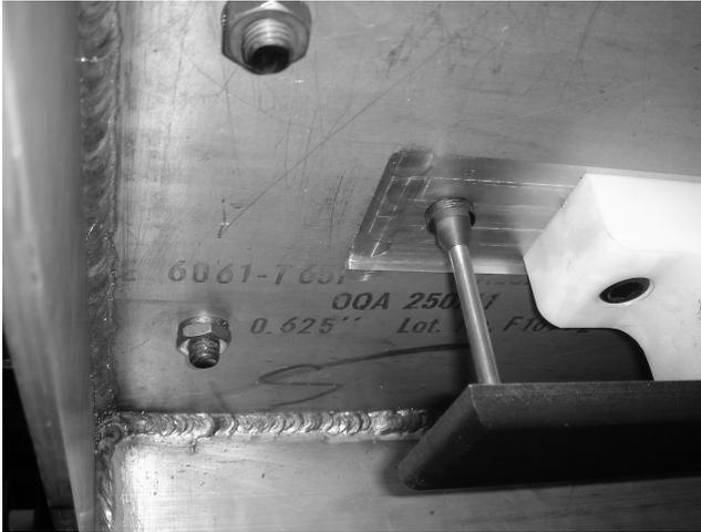
*Figure 7.3* Detail of the probe. Note the insulation at the aluminum shell. The probe is adjustable through a screw mechanism on the outside of the shell to allow for optimal coupling with the plate. Note also the rounding-off of the center plate designed to minimize the change of the fabric snagging on the plate. The channel is designed to keep the Delrin block in place with minimum chance of displacement should the center plate snag the fabric
