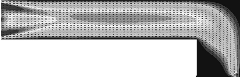
2.13 Laminar flow field of a 56 \times 2 " planetary reactor at a pressure of 600 mbar and a total flow rate of 400 slm.
