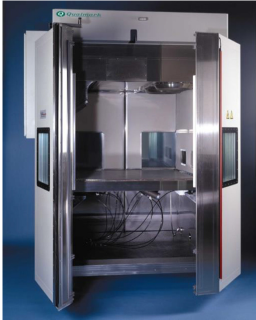
Figure 6.5 Typical HALT chamber. Source: QualMark 2015. Reproduced with permission of QualMark Corporation
