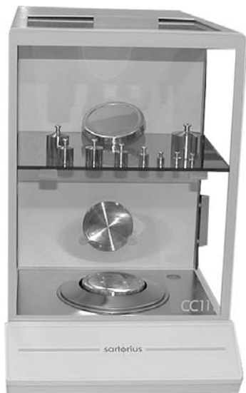
High quality mass balance with displacement feedback. Digital output can resolve mass increments to 0.00001 g.
