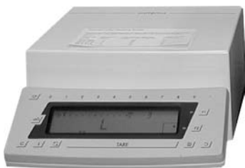
High quality mass balance with displacement feedback. Digital output can resolve mass increments to 0.00001 g.
