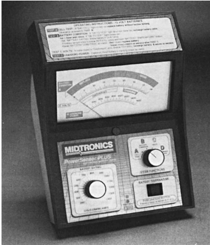
Fig. 12.25 Conductance monitoring equipment
