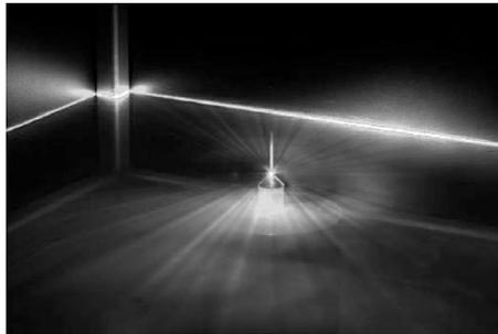
**Figure 7.2.** Conical mirror used to generate the optical reference plane. For a color version of this figure, see [www.iste.co.uk/thomas/sensors.zip](http://www.iste.co.uk/thomas/sensors.zip)
