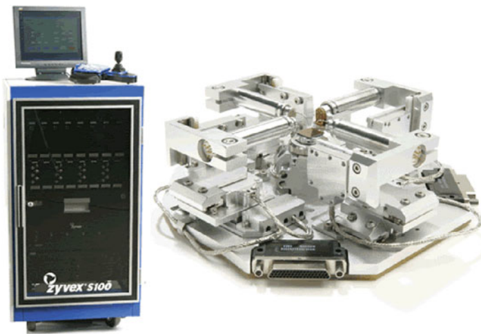
Fig. 2.1 Zyvox S100 Nanomanipulator system. Right image is the PC-based modular design system and left image is the head unit
