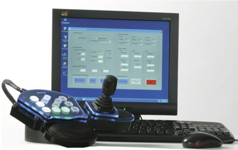
Fig. 2.2 Joystick and keypad control with user-friendly graphical user interface in a Windows environment
