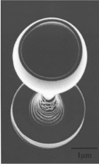
6.12 A diamond-like carbon wine glass with an outside diameter of 2.75 μm and height of 12 μm fabricated by direct writing with a 30 keV focused gallium beam in a hydrocarbon atmosphere (Reprinted with permission from Matsui *et al.*, 2000 ©2000, American Institute of Physics).
