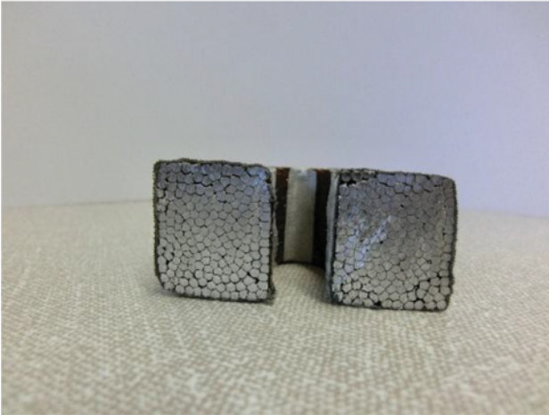
Figure 4.1 Pressed coil for high slot fill factor.
