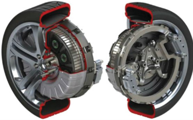
Figure 4.6 In-wheel electric motor, air cooled and axle water jacket [66]. Reproduced with permission of Protean Electric Ltd.
