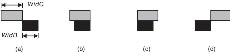
Figure 2.15 Different conducting position when WidB < WidC .
