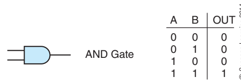
Figure 11-34 AND gate symbol and truth table.
