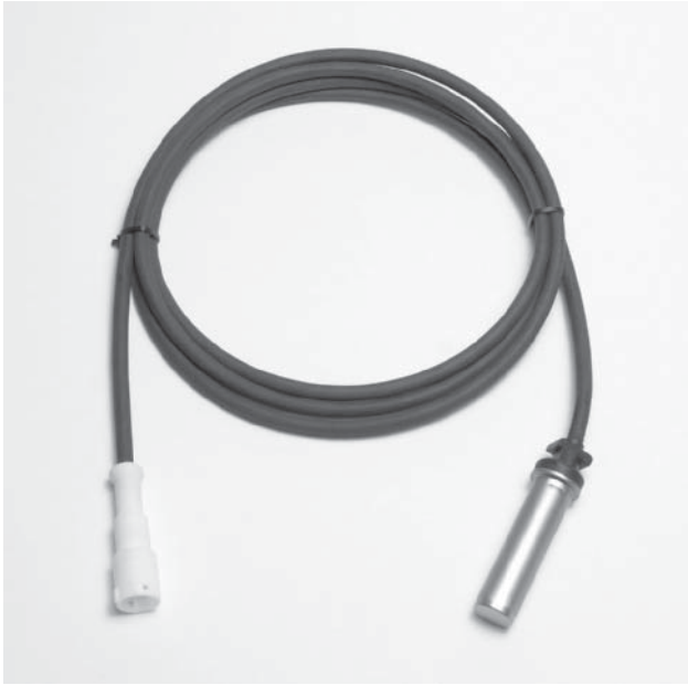
Figure 15-16 Typical ABS wheel-speed sensor with integrated wiring harness and connector.
