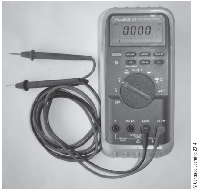
Figure 2-23 Digital multimeter with test leads attached for a voltage measurement.
