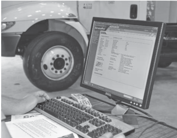
Figure 12-31 Electronic service tool used to modify ECM programmable parameters after tire size or rear-axle ratio change.
