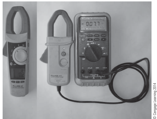
Figure 2-28 Clamp-on current probes. Probe on left is a stand-alone tool which displays current in amperes on a digital display. Probe on right is used with a DMM voltmeter. The voltmeter displays a voltage value which must be converted to current.
